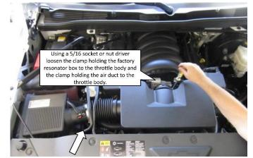
2. Using a 5/16 socket or nut driver loosen the clamp holding the factory resonator box to the throttle body and the clamp holding the air duct to the throttle body.
