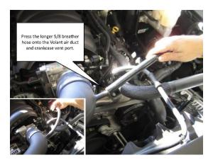
**9.** Press the longer 5/8 breather hose onto the CORSA air duct and crankcase vent port.
