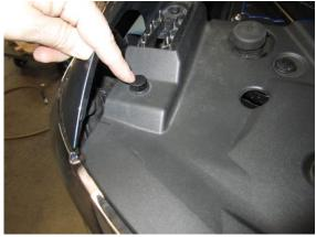
**16.** Reinstall the shroud support pins.
