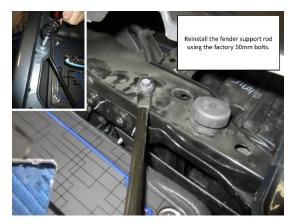
**15.** Reinstall the fender support rod using the factory 10mm bolts.
