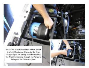
**3.** Install the air filter onto the filter flange. If you are having trouble installing the filter try reaching through the flange to help push the filter into place.
