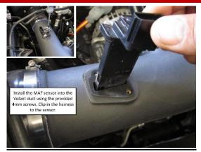
**14.** Install the MAF sensor into the CORSA duct using the provided 4mm screws. Clip in the harness to the sensor.
