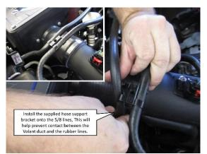
**17.** Install the supplied hose support bracket onto the 5/8 lines. This will help prevent contact between the CORSA duct and the rubber lines.
