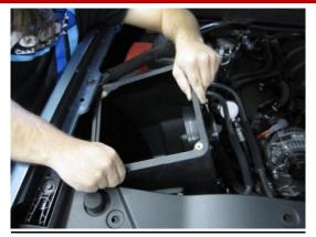
**1**. Place the CORSA box into the factory location.
