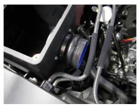
5. Attach the hump hose to the filter adapter using 5/16 socket or nut driver.
