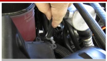
**1.** Remove the tree rivet holding the MAF harness to the air box.
