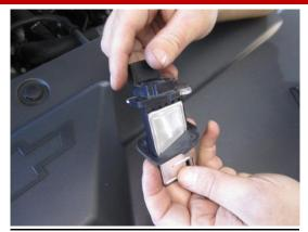
13. Install the supplied CORSA MAF gasket.
