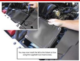
**1.** You may now install the lid to the CORSA air box using the supplied truss head screws.
