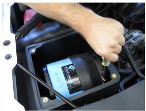
Tighten the filter into place only using a 5/16 socket or nut driver. Do not use a flathead screwdriver.
