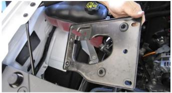
**9.** Remove the four 10mm bolts holding the air box mounting plate in place then remove the plate.
