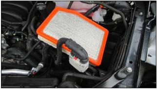
**9.** Remove factory air filter from lower air box.
