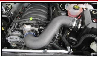
Insert CORSA air duct into hump hose and reducer.
