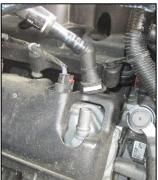
Remove factory breather hose at both ends by squeezing gray clip and pulling hose from fitting.
