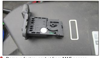
**12.** Remove factory gasket from MAF sensor.
