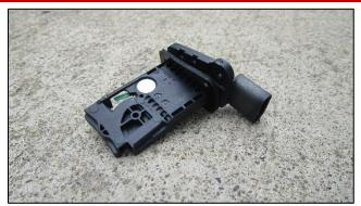
Install CORSA MAF gasket onto MAF sensor.
