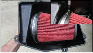
Install filter onto adapter in CORSA air box.Tighten clamp using a ratchet and 8mm socket.
