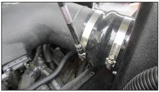
**B.** Adjust duct fitment as necessary and tighten all four clamps using a ratchet and 8mm socket.
