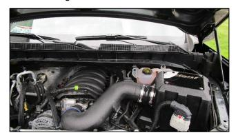
**12.** Remove protective wrap from CORSA lid. Connect negative battery terminal.
