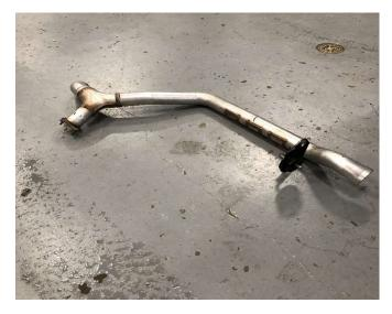
**12.** Carefully remove the passenger side tail pipe section.
