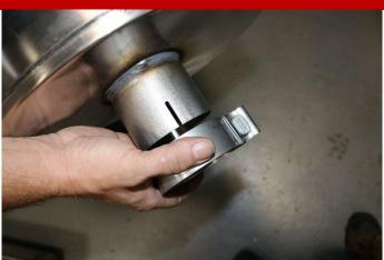
**4.** Put the 3" TORCA clamp on the expanded and notched end of the muffler.
