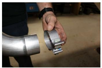
**13.** Insert a TORCA 2.5" Clamp into the expanded and notched end of the Drivers side Front Tail Pipe.
