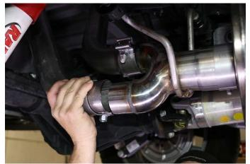
**16.** Slide the passenger side front tail pipe into the bottom section of the Y-Pipe as shown.
