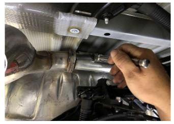
Loosen the factory flange on the driver's side tail pipe using a 13mm socket.
