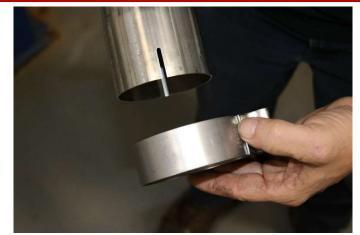
**9.** Insert a 3" TORCA clamp into the expanded and notched end of the Y – Pipe Assembly as shown.
