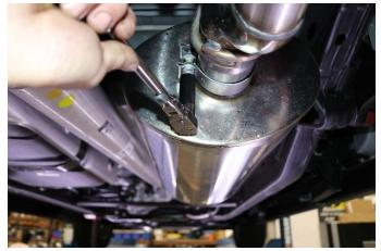
**12.** Snug the TORCA 3" clamp using a 15mm socket on the Y-Pipe Assembly as shown.
