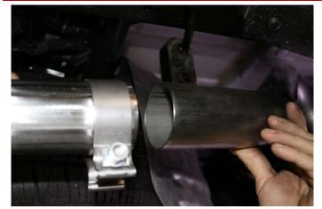
**20.** Slide the expanded and notched end of the passenger side rear tailpipe into the passenger side front tailpipe. Snug the TORCA 2.5" clamp using a 15mm socket.
