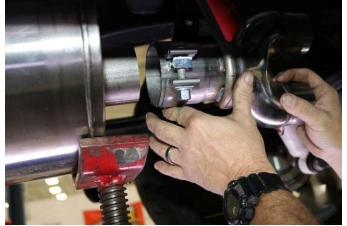
**10.** Slide the Y- Pipe Assembly into the side of the muffler supported by the stand as shown.
