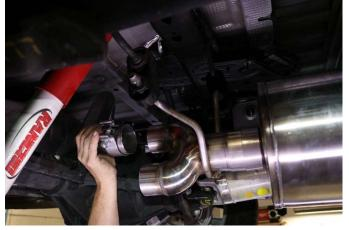
**14.** Slide the driver's side front tail pipe into the top section of the Y-Pipe as shown.
