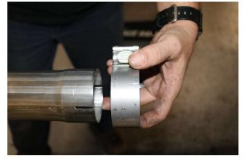
**18.** Insert a TORCA 2.5" clamp into the expanded and notched end of the passenger side rear tailpipe as shown.
