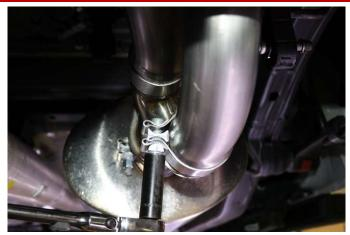
Snug the driver's and the passenger side front tailpipe TORCA clamps using a 15mm socket as shown. Make sure to leave the clamps loose enough to adjust position and rotation of the pipes.
