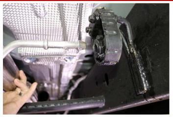
2. Put the headpipe hanger into the headpipe hanger grommet. Verify that there is at least a finger gap between the hanger and the frame of the truck when headpipe is secured in place.
