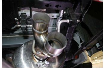
Insert the hangers on the Y-Pipe Assembly into the factory hanger grommets as shown.
