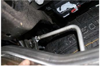
19. Insert the hanger on the passenger side rear tailpipe into the hanger grommet on the vehicle.
