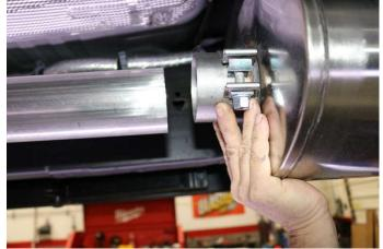
**6.** Slide the expanded end of the muffler or extension pipe onto the headpipe.
