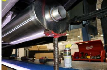
**1.** Use a stand to support the other end of the muffler as shown.
