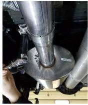
**5.** If your vehicle is a 157" WB, you will need to add the extension pipe to the inlet side of the muffler.
