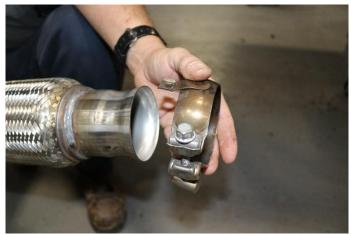
1. Reuse the stock spherical clamp and insert it on the head pipe on the side closest to the flex pipe as shown.
