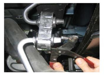
Remove the front section of the factory exhaust system along with the muffler and lay it aside. **8.** Remove the rear tailpipe grommet from the hanger at the rear of factory tailpipe, using grommet pullers or similar device.
