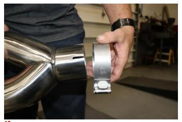
**14.** Insert a TORCA 3" Clamp into the expanded and notched end of the 4" Pro Series Tip Assembly
