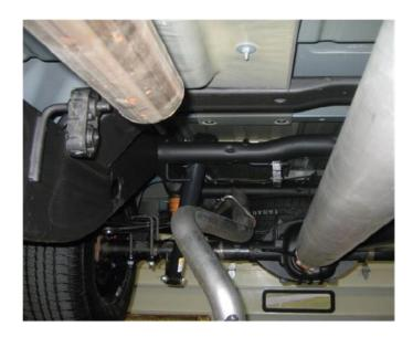
**9.** Remove the factory tail pipe section of the exhaust.
