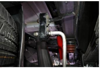
**12.** Insert the rear hanger on the Tailpipe Assembly into the factory hanger grommet as shown.
