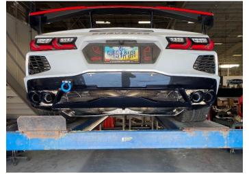
**38.** At this time, adjust the tip tube and tip positions until all tips are centered within the cutouts in the rear valence, and there is approximately ½" reveal at the CORSA logo of each tip. Torque all exhaust clamp bolts to 45 FT-LBS.
