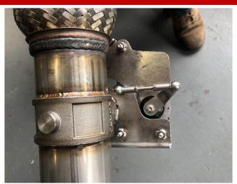
(FOR AFM VALVE ONLY) The AFM valve actuators should now be connected to the CORSA AFM valve assemblies as shown.
