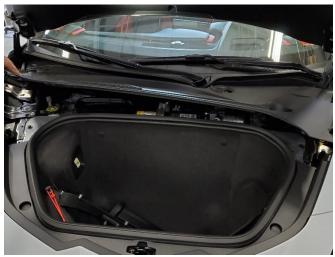
2. Unclip the front trunk battery cover panel and remove from the vehicle. Set aside the panel in a protected location.
