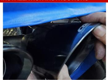
**35.** Locate one of the CORSA stainless (or Carbon) inner tip assemblies, and a 2.5" clamp from the hardware kit. Position the clamp on the tip inlet so the clamp bolt is on top of the tip and the clamp nut is facing inwards. Insert the inlet of the inner tip assembly onto the elbow pipe with approximately 1.5" of overlap.
