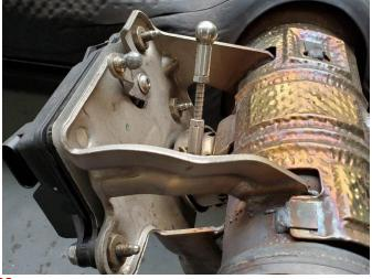
28. Remove both of the AFM valve actuator linkages from the AFM valve actuators and the stock AFM valve assemblies.
