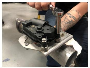
6. (FOR AFM VALVE DELETE ONLY) Align and secure both of the factory AFM valve actuators to the CORSA AFM delete assemblies using a 10mm socket and a 1/4" ratchet. Torque to 89 IN-LBS.
