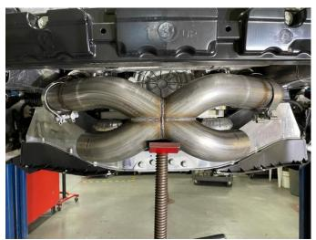
14. Support the center of the CORSA X-pipe with a jack stand. Adjust the height of the jack stand until there is approximately a ½" gap between the top of the X-pipe inlet and the chassis on both sides as shown.
