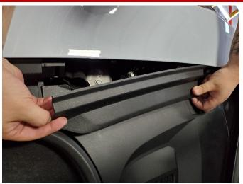
Beginning at the front of the vehicle, unclip the front trunk side panels and remove from the vehicle. Set aside the panels in a protected location.
