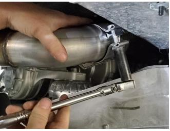
**16.** Tighten both of the exhaust clamps at the X-pipe inlet using a 15mm socket and 3/8" ratchet to secure the X-pipe assembly.
