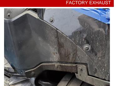
The rearward most rear under tray is secured by two push clips (1 per side), four T15 TORX screws (2 per side), and six 7mm bolts (3 per side). Remove the push clips first using a removal tool or flathead screwdriver, followed by the T15 TORX screws, and then the bolts using a 7mm socket and 1/4" ratchet. This will free the rearward under tray from the vehicle. Set aside the rearward under tray and fasteners in a protected location.
