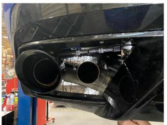
**34.** Adjust the rotation of the CORSA outer tip assembly until the CORSA logo is centered on the top of the tip, then tighten the exhaust clamp at the tip inlet using a 15mm socket and 3/8" ratchet.
