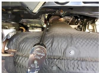
Remove the two M10 nuts that secure the driver side cat back mounting flange to the factory catalyst using a 15mm socket, a 3/8" ratchet, and a 24" long extension. Set aside the fasteners in a protected location.
