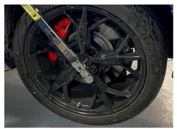
Remove the ten lug nuts and the two rear wheels from both sides of the vehicle using a 22mm socket and ½" ratchet or ½" drive breaker bar. This will allow access to the factory inner fender liners. Set aside the rear wheels and lug nuts in a protected Location.
