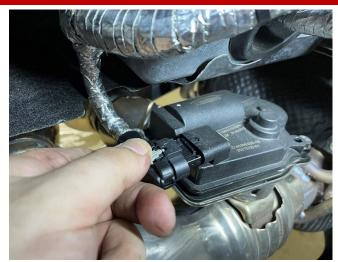
17. (FOR NPP VALVE ONLY) Disconnect the wiring connectors to both of the NPP valve actuators: these are located on the pipes leading to the outer exhaust tips. Note that the grey locking tab on the wiring connectors must be slid outwards before disconnecting the wires from the actuators.
