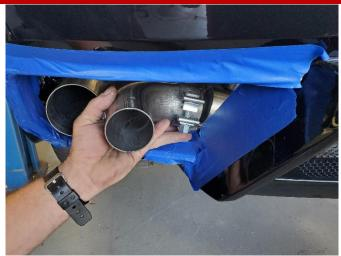
**31.** Locate one of the CORSA inner tip elbow pipes, and a 2.5" clamp from the hardware kit. Position the clamp on the elbow pipe inlet so the clamp bolt is facing towards the bend and the clamp nut is facing downwards. Insert the inlet of the elbow pipe onto the non-valved outlet of the driver side muffler with approximately 1.375" of overlap.
