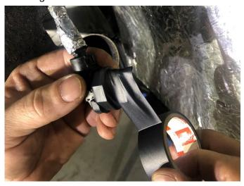
**28.** (FOR MUFFLER DELETE ONLY) Tape off the NPP valve wiring connectors to aid in keeping moisture out of the electrical connection, as they are no longer utilized on the rear muffler delete versions of the CORSA exhaust installation.
