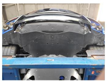
The rear bumper cover, two rear under trays, two inner fender liners, and the rear wheels will all need to be removed first in order to allow removal of the factory exhaust.
