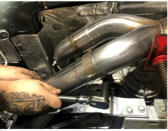
23. Tighten the exhaust clamp at the driver muffler (or muffler delete) inlet using a 15mm socket and 3/8" ratchet to secure the muffler/muffler delete assembly.
