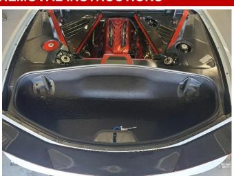
**13.** Remove the sixteen T15 TORX screws that secure the top of the factory rear bumper cover to the chassis. Start with the fourteen screws that run along the top edge of the bumper.
