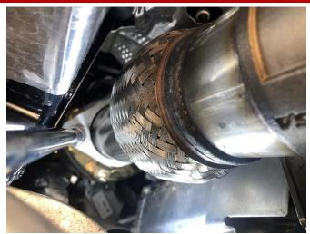
11. Next, secure the driver side cat back mounting flange to the factory catalyst using a 15mm socket, a 3/8" ratchet, and a 24" long extension. Torque to 32 FT-LBS.
