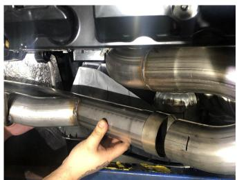
20. Position the clamp on the CORSA driver muffler (or muffler delete) inlet so the clamp bolt is in front of the expansion and the clamp nut is facing downwards. Insert the inlet of the driver muffler/muffler delete assembly on to the driver side outlet of the X-pipe with approximately 1.75" of overlap.
