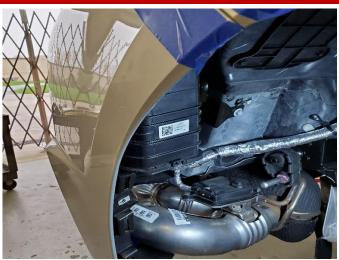
10. Repeat Removal Step 9 for the passenger side of the vehicle. Set aside both inner fender liners and fasteners in a protected location. Removal Steps 9-10 will allow access to the factory fender to rear bumper cover connections on each side of the vehicle.
