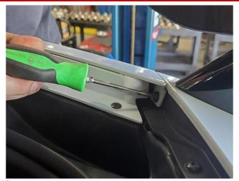
14. Remove the last two T15 TORX screws that are facing rearward and tucked into the corner of the fender on each side. This will allow the bumper cover to move independently from the vehicle. Set aside the fasteners in a protected location.
