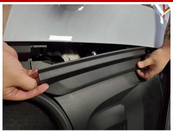
Beginning at the front of the vehicle, unclip the front trunk side panels and remove from the vehicle. Set aside the panels in a protected location.
