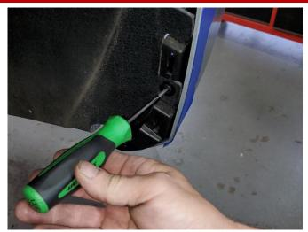
The inner fender liners are secured by eleven T15 TORX screws, four push clips, and three 7mm bolts per side. Starting on the driver side, remove the push clips first using a removal tool or flathead screwdriver, followed by the T15 TORX screws, and then the bolts using a 7mm socket and 1/4" ratchet. This will free the inner fender liner from the vehicle.
