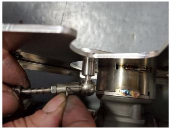
(FOR AFM VALVE ONLY) Locate the two CORSA AFM valved head pipe assemblies, and the two stock AFM valve actuator linkages and four locking pins set aside in Removal Steps 27 & 28. Connect both of the AFM valve actuator linkages to the CORSA AFM valve assemblies. Secure the connections with the locking pins.
