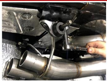
22. Locate two of the factory rear grommet bolts set aside in Removal Step 18. Insert both bolts through the driver rear exhaust grommet and secure the grommet to the chassis using a 13mm socket and 3/8" ratchet. Torque to 17 FT-LBS.
