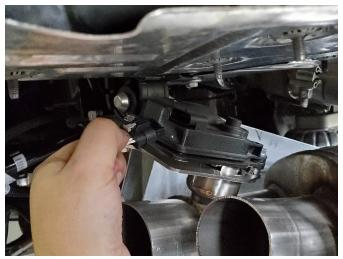
27. (FOR NPP VALVE ONLY) Connect the opposite end of the wiring extensions to the NPP valve actuator on both sides of the vehicle. Push in the grey locking tabs on the wiring connectors to secure the connections.
