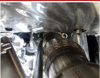
Secure the passenger side cat back mounting flange to the factory catalyst using a 13mm socket, a 3/8" ratchet, and a 24" long extension. Torque to 17 FT-LBS.
