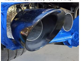
**33.** Locate one of the CORSA stainless (or Carbon) outer tip assemblies, and a 3" clamp from the hardware kit. Position the clamp on the tip inlet so the clamp bolt is on top of the tip and the clamp nut is facing inwards. Insert the inlet of the outer tip assembly onto the elbow pipe with approximately 1.5" of overlap.
