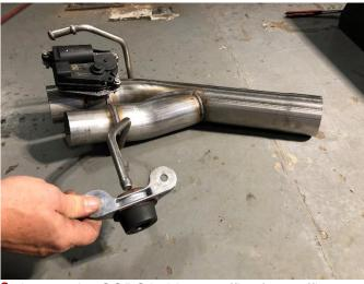
19. Locate the CORSA driver muffler (or muffler delete) assembly, a 3" clamp from the hardware kit, and one of the rear grommets set aside in Removal Step 25. Install the rear exhaust grommet onto the rear hanger position. Make sure the protruding rubber side of the grommet faces away from the piping (rearward) as shown.
