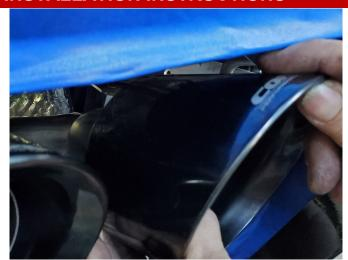
**37.** Locate one of the CORSA inner tip assemblies, and a 2.5" clamp from the hardware kit. Position the clamp on the tip inlet so the clamp bolt is on top of the tip and the clamp nut is facing inwards. Insert the inlet of the inner tip assembly onto the elbow pipe with approximately 1.5" of overlap.
