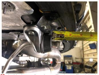
**25.** At this time, adjust the muffler (or muffler delete), X-pipe, and head pipe positions until there is approximately 1/2" between the outer face of the rear grommets and the forward edge of the head on the rear hangers on both driver and passenger sides of the vehicle as shown. It is critical for proper fitment to get the system adjusted a square as possible on the vehicle.
