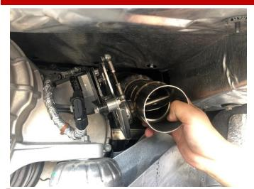
7. (ALL VERSIONS) Locate the three M8 nuts set aside in Removal Step 20. Insert the passenger side CORSA head pipe assembly onto the studs from the catalyst as shown, then hand tighten the M8 nuts to hold the head pipe in place. Note the position of the AFM valve actuator within the chassis when it is correctly positioned.
