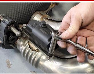
**26.** (FOR NPP VALVE ONLY) Remove the six bolts (3 per side) that secure both of the factory NPP valve actuators using a 10mm socket and a 1/4" ratchet. Set aside the NPP actuators in a protected location. The NPP valve actuators will be reused during the installation of the CORSA exhaust system.
