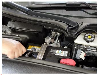
**3.** Disconnect the negative battery terminal using a 10mm socket and 3/8" ratchet.
