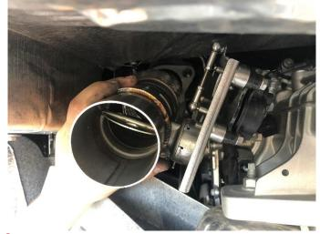
Locate the two M10 nuts set aside in Removal Step 19. Insert the driver side CORSA head pipe assembly onto the studs from the catalyst as shown, then hand tighten the M10 nuts to hold the head pipe in place, leaving the nuts loose enough that the head pipe can still pivot and rotate.
