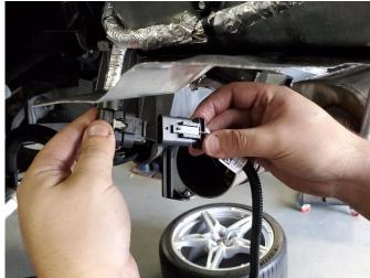
**26.** (FOR NPP VALVE ONLY) Locate both NPP valve wiring extensions from the hardware kit. Connect both wiring extensions to the chassis side of the NPP valve wiring connectors. Push in the grey locking tabs on the wiring connectors to secure the connections.
