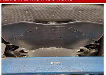
The forward most rear under tray is secured by one push clip and ten 7mm bolts. Remove the push clip first using a removal tool or flat head screwdriver. Next, remove the bolts using a 7mm socket and 1/4" ratchet to free the forward under tray from the vehicle. Set aside the forward under tray and fasteners in a protected location.
