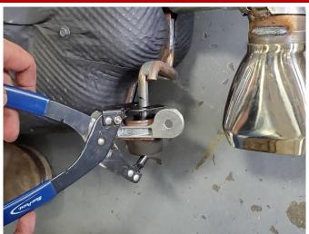
**25.** Remove both of the rear exhaust grommets from the exhaust hangers using grommet pullers or similar device. Note the orientation of the grommets for the installation of the CORSA exhaust system.
