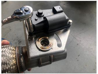
2. (FOR AFM VALVE ONLY) Locate the two stock AFM valve actuators set aside in Removal Step 29, and six of the supplied M6 bolts from the hardware kit. Align and secure both of the factory AFM valve actuators to the CORSA AFM valve assemblies using a 10mm socket and a ¼" ratchet. Torque to 89 IN-LBS.
