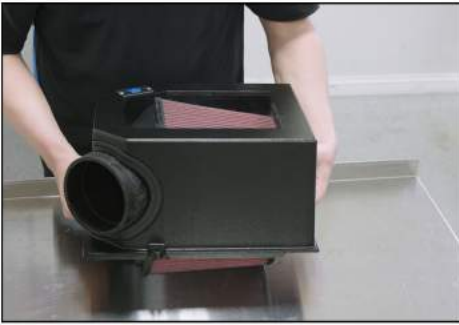
16. Insert FILTER ELEMENT into AIR INDUCTION HOUSING.
