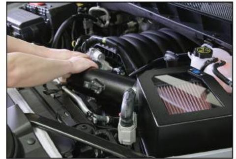
21. Install AIR INDUCTION HOUSING into the vehicle.
