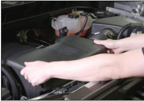
7. Remove OUTLET/DUCT from vehicle.
