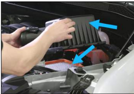
10. Remove AIR INDUCTION HOUSING COVER and air filter. Place the factory AIR INDUCTION HOUSING on work bench.
