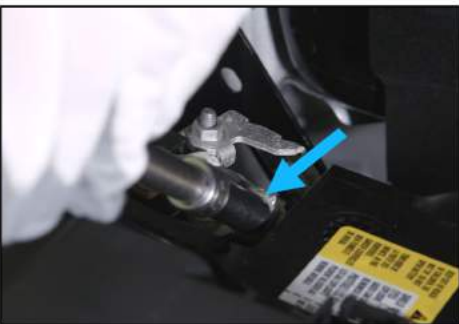
25. Reconnect negative battery terminal with 10mm socket and ratchet.
