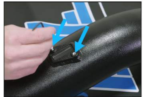
12. Remove both screws on the MAF/TUBE with 2.5mm allen wrench.
