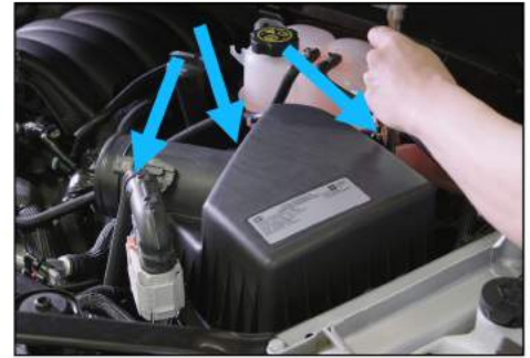
9. Remove the OEM COVER using the ratchet, 8mm socket and extension. Remove all three screws.
