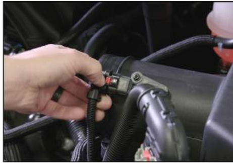
8. Disconnect the wire harness from the MAF sensor.
