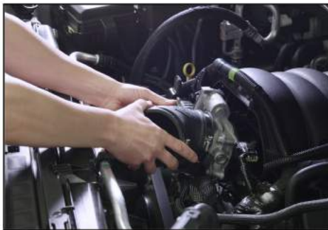
14. Install INLET/DUCT onto throttle body. Leave all connections loose.
