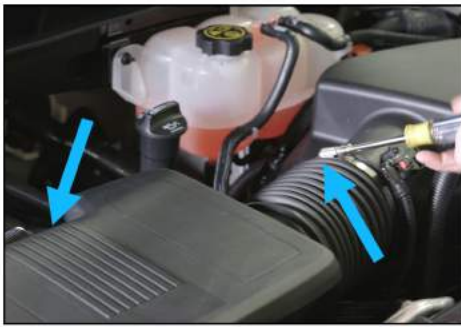
4. Loosen clamp on throttle body and air cleaner assembly.
