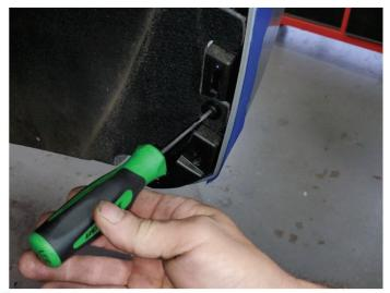
9. The inner fender liners are secured by eleven T15 TORX screws, four push clips, and three 7mm bolts per side. Starting on the driver side, remove the push clips first using a removal tool or flathead screwdriver, followed by the T15 TORX screws, and then the bolts using a 7mm socket and ¼" ratchet. This will free the inner fender liner from the vehicle.
