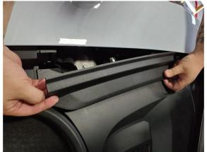
1. Beginning at the front of the vehicle, unclip the front trunk side panels and remove from the vehicle. Set aside the panels in a protected location.
