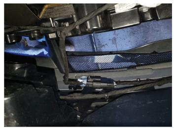
15. Get 1 to 2 helpers for Removal Steps 15 & 16. There are three wiring harness connectors that need to be disconnected to be able to remove the factory rear bumper cover from the vehicle. We recommend a person on each side of the vehicle CAREFULLY slides the rear bumper cover straight back over the exhaust tips and holds the bumper cover in the air while a third person disconnects the driver side connector....
