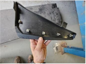
8. Unclip the two rear splash guard panels from the outside rearmost corners of the inner fender liners. Set aside the panels in a protected Location.
