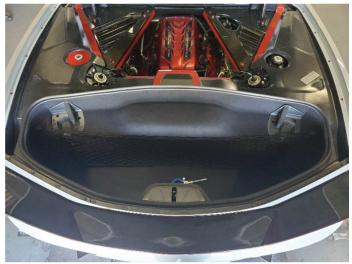
Remove the sixteen T15 TORX screws that secure the top of the factory rear bumper cover to the chassis. Start with the fourteen screws that run along the top edge of the bumper.
