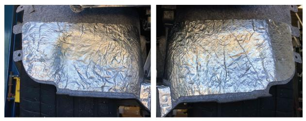
**17.** Locate the silver factory heat shields that are attached to the wheel well liners. Clean them thoroughly and make sure they are free of dirt, oil and other contaminants.
