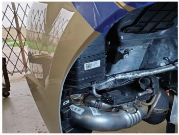
Repeat Removal Step 9 for the passenger side of the vehicle. Set aside both inner fender liners and fasteners in a protected location. Removal Steps 9-10 will allow access to the factory fender to rear bumper cover connections on each side of the vehicle.
