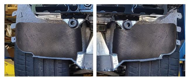
**18.** Test fit the two black shield to each side. Peel back top of release liner and line up along the top of the silver shield and press in place. Once the top is adhered, reach behind the shield and slowly pull backing liner down while pressing the shield in place. Press firmly to make sure shields are competely adhered. The adhesive is very aggressive. Take your time to get original position correct.
