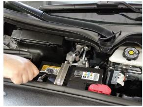
**3.** Disconnect the negative battery terminal using a 10mm socket and 3/8" ratchet.
