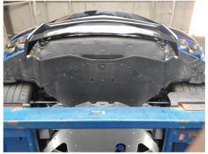
4. The rear bumper cover, two rear under trays, two inner fender liners, and the rear wheels will all need to be removed first in order to allow removal of the bumper cover
