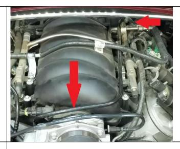
Remove 15mm bolt from drive belt tensioner. Install J&L bracket and reinstall bolt. Bolt torque spec is 37 Ft/lbs.
