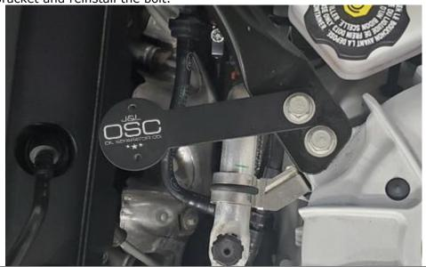
Page 1 of 2 9-21-21 Use the supplied screws and attach J&L Separator to the bracket as shown below.
