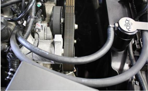
6 Reinstall mounting bolt for bypass assembly, reinstall engine cover and you're all done!
