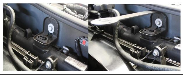
Route the 22" hose from the Valley cover (lower fitting on the car) to the fitting on the Oil Separator closest to the engine. Route the 26" Hose from the upper fitting on the engine (to manifold) to the fitting closest to the radiator on the Oil Separator. Push hoses onto fittings, you should hear/feel a click as they engage.
