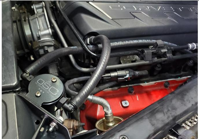
Check your oil separator after 500-1000 miles of driving to get an idea of how often it needs to be emptied. Every vehicle is different! Given the location of this oil separator be sure to check it when the vehicle is **COLD**!
