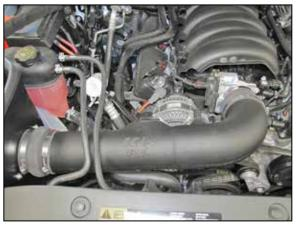
20. Install the K&N<sup>®</sup> intake tube into the hose at the filter adapter and then into the hose at the throttle body, adjust the tube for best fit and then secure with the provided hose clamps.
