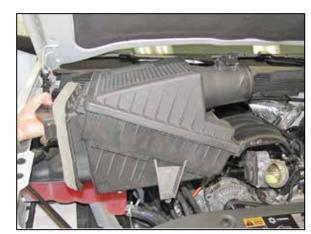
6. Pull up the air box to release it from the mounting grommets and then remove the factory air box from the vehicle.
