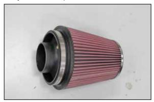
10. Install the filter adapter into the K&N<sup>®</sup> air filter and secure with the provided hose clamp. NOTE: Drycharger<sup>®</sup> air filter wrap; part # **RF-1041DK** is available to purchase separately. To learn more about Drycharger® filter wraps or look up color availability please visit http://www.knfilters.com®.
