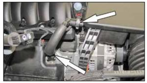
3. Disconnect the crank case vent from the intake plenum and valve cover port and remove it from the engine.
