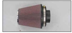
10. Install the filter adapter into the K&N $^{\circ}$  air filter and secure with the provided hose clamp.
