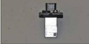
15. Remove the two screws securing the mass air sensor into the air filter housing and then remove the mass air sensor from the air filter housing. Install the mass air sensor into the K&N<sup>®</sup> adapter and secure with the provided hardware.
