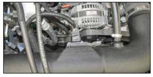
20. Reconnect the mass air sensor electrical connection.
