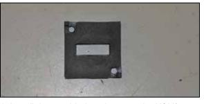
14. Install the provided gasket onto the K&N<sup>®</sup> mass air sensor adapter.
