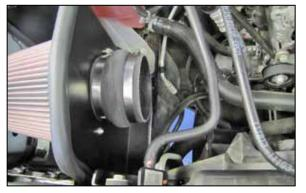
13. Install the provided hump hose (08418) onto the filter adapter and secure with the provided hose clamp. 18. Install the K&N<sup>®</sup> intake tube into the hose at the filter adapter and then into the hose at the throttle body. Adjust the tube for best fit and then secure with the provided hose clamps.
