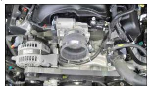
12. Install the provided step hose (084055) onto the throttle body and secure with the provided hose
