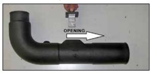
16. Install the mass air sensor assembly into the K&N<sup>®</sup> intake tube and secure with the provided hardware.
