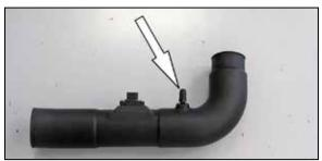
17. Install the vent fitting into the K&N<sup>®</sup> intake tube. NOTE: NPT fitting has tapered threads and only designed to be installed until hand tight, then tighten one rotation or when the fitting becomes difficult to return.
