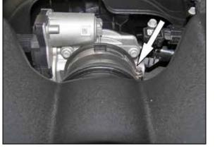
5. Loosen the hose clamp securing the intake plenum to the throttle body and then remove the intake plenum from the vehicle.
