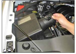
6. Lift up and remove the air filter housing from the vehicle.
