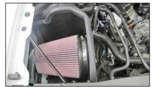
11. Install the filter assembly into the heat shield filter top first, then rotate the filter and pass the adapter through the hole in the heat shield. Secure the filter adapter to the heat shield using the provided hardware.
