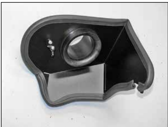
17. Install the provided edge trim onto the heat shield as shown. NOTE: Some trimming of the edge trim will be necessary.
