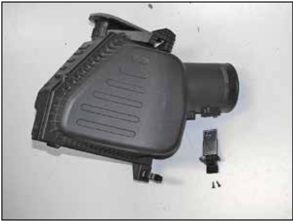
18. Remove the mass air sensor from the factory air filter housing.
