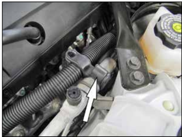
8. Disconnect the mount securing the sound tube to the A/C line.
