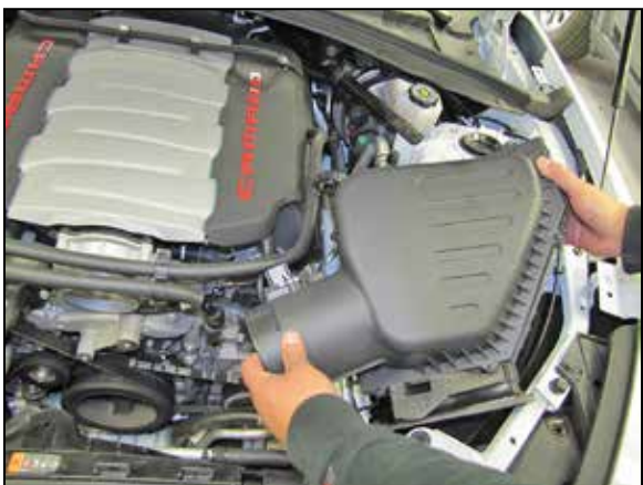
12. Lift up the air filter housing to dislodge it from the mounting grommets and then remove it from the vehicle. NOTE: K&N Engineering, Inc., recommends that customers do not discard factory air intake.
