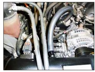
20. Connect the passenger side CCV hose to the K&N intake tube. Reconnect the mass air sensor electrical connection.
