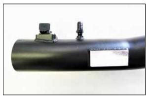
16. Install the mass air sensor into the K&N intake tube and secure with the provided hardware. Apply thread sealant to the CCV fitting and install it into the K&N intake tube.
