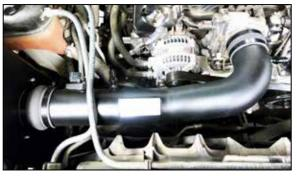
18. Install the K&N<sup>®</sup> intake tube into the hose at the filter adapter and then into the hose at the throttle body. Adjust the tube for proper fit and then secure with the provided hose clamps.
