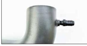
17. Apply thread sealant to the remaining CCV fitting and install it into the K&N intake tube.
