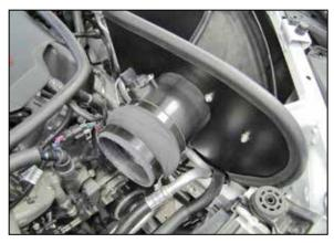
22. Install the provided step hump coupler (08633) onto the filter adapter and secure with the provided hose clamp.
