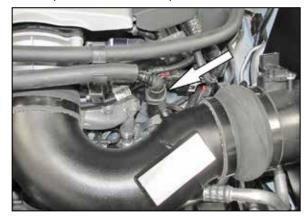
25. Connect the crank case vent hose to the quick
