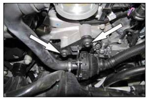
6. Remove the two bolts securing the sound drum to the front of the engine.
