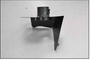
13. Install the K&N<sup>®</sup> mass air sensor into the heat shield and secure with the provided hardware.
