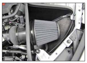
27. Install the K&N $^{\circ}$  air filter and secure with the provided hose clamp.
