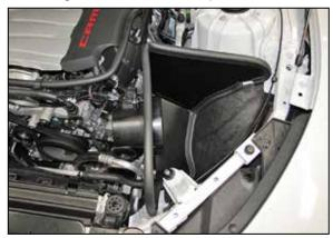
20. Install the K&N<sup>®</sup> heat shield assembly onto the air filter housing mounting grommets.
