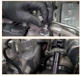
06. Locate the tapered hose in your kit with two bends. Install a worm-gear clamp over the wider end and slip it over the fitting marked OUT on the catch can. Lead the tapered end under the emissions hose and slip a worm-gear clamp over this end. Now locate the double-barb hose fitting in your kit and install it to the tapered end of the hose. (2x worm-gear clamp)
