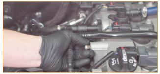
08. Install the PCV adapter. This adapter is sealed by a small O-ring at the end. Take care when installing the adapter to avoid damaging this seal. If the adapter is installed on an angle, the O-ring will be damaged. Lubricate the O-ring with fresh engine oil and insert the adapter into the valve cover. Lift up on the CCV lines as you thread in the fitting and take your time to avoid damaging it.
