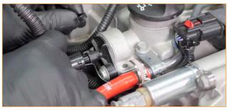
21. Locate the hose in your kit with a 180Đ bend on one end and one of the larger quick-disconnect fittings. Slip a worm-gear clamp over the hose and install the fitting as shown here. Leave the clamp loose for now. (1x worm-gear clamp, 1x large quick-disconnect fitting)
