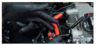
13. Locate the tapered hose in your kit with three bends. Install a worm-gear clamp over the wider end and slip it over the fitting marked IN on the catch can. Slip a worm-gear clamp over the other end of the hose and install it to the straight tube on the PCV adapter. Now tighten all six clamps to secure the hoses. (2x worm-gear clamps)
