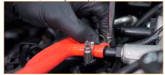
14. Turn the catch can until the lines flow smoothly, and then tighten the two bolts that secure the can to the bracket.
