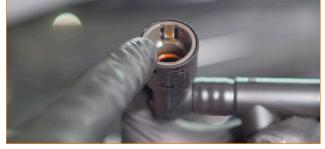
20. This step can be a bit tricky, so take your time. The tools are meant to be bent in order to maneuver them around other components on the engine. Start with the rear CCV hose connection. Slip the tools behind the connector and squeeze the connector and tools together to depress the tabs. Then slide the connector off of the fitting. Once the rear hose is loose, turn the hose for better access to the forward connection. Now repeat the removal process on the forward connection.
