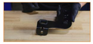
3. Slide the bracket onto the radiator. Secure the Mishimoto bracket where the upper radiator support used to be. (1x 10mm bolt)
