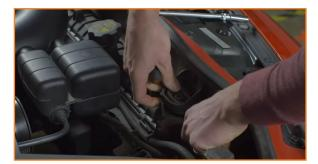
2. Transfer the bushing on the upper radiator support to the catch can bracket.
