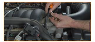
6. Connect the longer hose to the back of the engine. Run the hose up to the catch can bracket.
