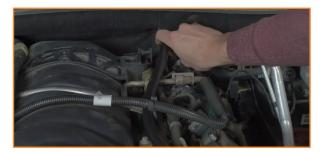
7. Connect the smaller hose to the open port at the front of the engine.
