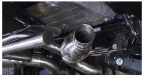
10. Align the brackets on the resonators to secure them with the bolts from your kit. Leave the bolts loose for now.
