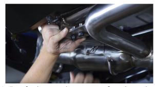
11. Transfer the rear exhaust mounts from the stock exhaust hangers to the Mishimoto tips.
