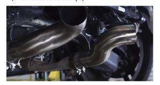
9. Slide clamps over each of the front pipes and then install the muffler pipes. The muffler pipes are marked Left and Right. Push the hangers on the exhaust pipes into the adjacent rubber mounts. (2x exhaust band clamps)
