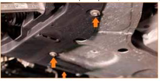
28. Look through the hole behind the panel you just removed to locate the last coolant line connection. Place a drain pan underneath the hose. Compress the clamp that secures the coolant line, and slide it up the hose. Then remove the hose from the coolant pipe. (1x spring clamp)
