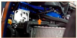
25. Pull back the passenger-side fender liner, and locate the inner coolant hose on the auxiliary radiator. Release the tree-clip that secures this hose to the body of the vehicle. Compress the clamp that secures the hose to the radiator, and slide the clamp down the hose. Then remove the hose from the fitting. (1x tree-clip, 1x spring clamp)
