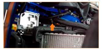
22. Release the lower radiator hose from the plastic clip that connects it to the small coolant hose below the water outlet.
