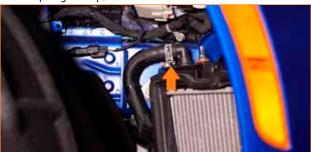
26. Remove the screw and pop-clip that secure the rear portion of the fender liner on the driver side. (1x T15 Torx screw, 1x pop-clip)
