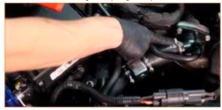
13. Compress the clamp that secures the upper radiator hose to the radiator, and move the clamp down the hose. Then remove the hose from the vehicle. (1x worm-gear clamp)
