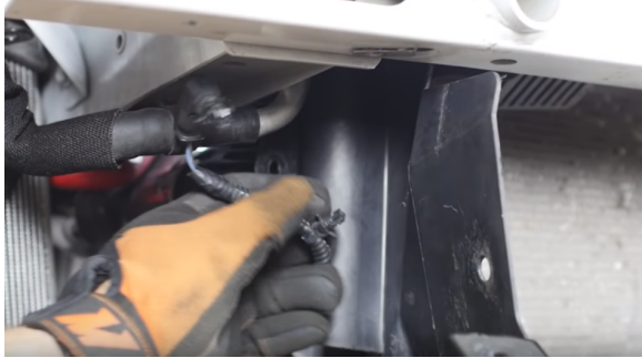
26. Remove the radiator stay ends and upper shroud. (4x 10mm bolts)
