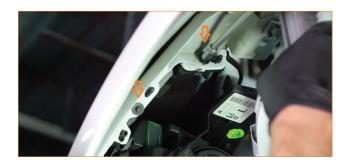
**15.** Remove the two screws that secure the bumper to the fender, and loosen the inner screw. (3x 7mm screws)
