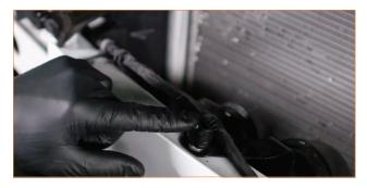
28. Locate the small bracket with the threaded insert in your kit. Lift the horn assembly off the crash bar, and install the bracket in its place. Orient the bracket so that the threaded insert faces toward the passenger side, and secure it with the stud you just removed. Then reattach the wiring harness to the stud. (1x 10mm stud)
