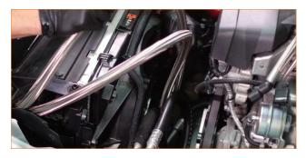
48. Locate the silicone sleeve in your kit. Slip the sleeve over the stabilizer bar where the oil lines cross under it, and secure the sleeve with the short zip ties included with your kit.
