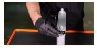
34. Locate the last bracket in your kit. Attach this bracket to the forward-most hole on the bottom of the driver side of the cooler with the provided hardware. Thread the bolt in, but do not fully tighten it. (1x 10mm bolt, 1x Nyloc nut)
