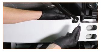
**36.** Align the driver-side bracket with the hole in the crash bar, and secure it with the provided bolt and washer. (1x 10mm bolt, 1x plastic washer)
