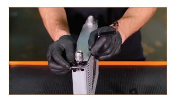
**33.** Locate the angled bracket in your kit. Attach this bracket to the driver-side of the oil cooler with the provided hardware, but do not fully tighten it yet. [2x 10mm bolts, 2x Nyloc nuts]
