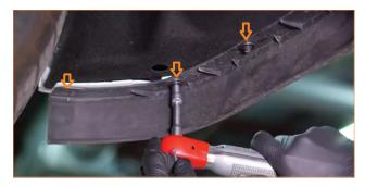
**09.** Remove the eight screws that secure the lower edge of the bumper. (8x 7mm screws)
