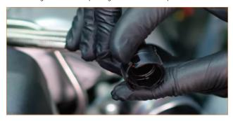
04. Disconnect the mass airflow (MAF) sensor, and release the harness from the intake tubing. To release the connector, slide the red locking tab up, depress the black tab, and pull the connector off the sensor.
