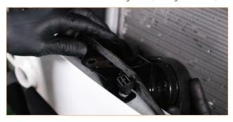
**30.** Remove the two pop-clips that secure the air diverter to the ducting. (2x pop-clips)
