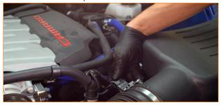
**31.** Disconnect the CCV hose from the intake. Depress the gray tab to release the fitting.
