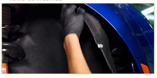
08. Release the two tree clips that secure the lighting harness to the vehicle. Release the harness connector from the body and disconnect it. To release this connector, slide the red lock tab out of the connector and depress the black tab. (2x tree clips)
