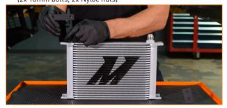
20. Locate the angled bracket in your kit. Attach this bracket to the driver side of the oil cooler with the provided bolts and nuts, but do not fully tighten yet. (2x 10mm bolts, 2x Nyloc nuts)
