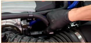
**32.** Compress the clamp that secures the sound-generator hose to the intake, and separate the hose.
