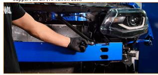
25. Slip the Mishimoto cooler and attached brackets under the crash bar while tilting it up to clear the AC condenser. Align the angled bracket with the support strut, and thread in the bolt that originally held the strut. (1x 10mm bolt)
