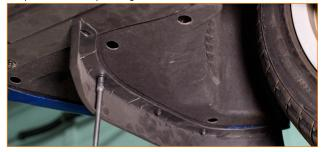
04. Remove the eight screws that secure the lower edge of the bumper. (8x 7mm screws)
