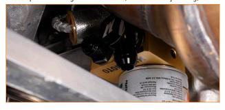
**41.** Locate the oil line with two 90° fittings in your kit. Gently push back on the radiator, and lead one end of this hose between the radiator and the radiator support.
