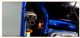
09. Remove the two screws that secure the bumper to the fender, and loosen the inner screw. (3x 7mm screws)
