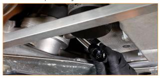
47. Lead the other oil line alongside the first; however, this line will pass on the other side of the engine mount, toward the rear of the vehicle. Attach this line to the banjo fitting on the sandwich plate. Adjust the orientation of the banjo fitting to provide maximum clearance between the steering shaft and the oil line. Then tighten the banjo bolt and the oil-line fitting.
