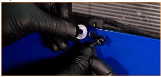
27. Remove the two pop-clips that secure the air diverter to the ducting. Align the remaining bracket in your kit with the holes in the air diverter, and reinstall the pop-clips to secure it. Attach the cooler to the bracket with the provided nut and bolt. [2x pop-clips, 1x 10mm bolt, 1x 10mm nut]
