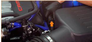
**35.** Remove the airbox and intake hose from the vehicle by lifting the airbox upward. The airbox is held in by only pegs and grommets.
