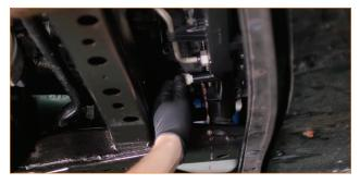
03. Separate the overflow hose from the radiator. Then squeeze the clamp that secures the coolant hose to the water neck of the radiator, and separate the hose from the radiator. (1x spring clamp)
