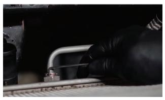
Remove the bolt that secures the radiator mount to the radiator support, and remove the mount. Repeat this process on the other side.
