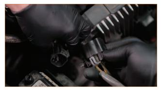
07. Compress the clamp that secures the upper radiator hose to the radiator, and then separate the hose from the radiator. (1x spring clamp)
