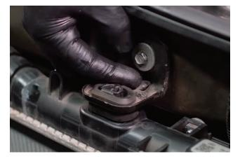
Tilt the radiator back to expose the mounting bolts for the AC condenser. Remove the bolts to separate the AC condenser from the radiator. (2x 10mm bolts)
