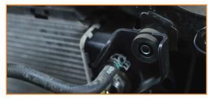
13. Remove the transmission cooler line from the radiator. (2x spring clips)
