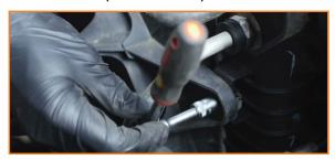
Separate the upper oil cooler line from the radiator. Slide the clip cover down the line, and then pull out the clip that secures the connection. Plug the line to prevent spillage. (1x spring clip)
