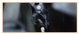
8. Remove the bolts that secure the fan shroud to the radiator. (2x 10mm bolts)
