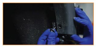
3. Disengage the bumper cap at the sides and along the bottom of the grille. There are a number of tabs just under the grille that will release this piece. Remove the loose bumper cap.
