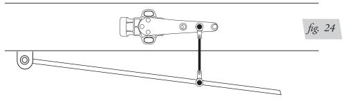
4. Loosen if needed in order to extend to reach the lower mounting point. If loosening the linkage to extend, it is required to make sure to have at least 5 threads of engagement on both ends (fig. 25).
