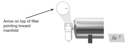
4. If choosing not to mount the filter to the tank, run necessary hose from tank to the filter and filter to the manifold using the appropriate fittings.
