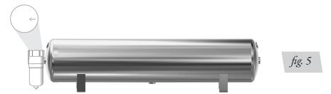
2. Ensure the filter is mounted in a vertical position. Do not install filter inverted or angled (fig. 6).
