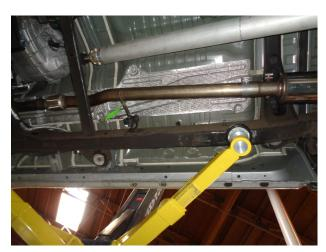
Step 3. Install the appropriate extension pipe depending on the cab size. Install the Inlet Pipe using the supplied 3.00" clamp then attach the Muffler Assembly to the Extension Pipe.
