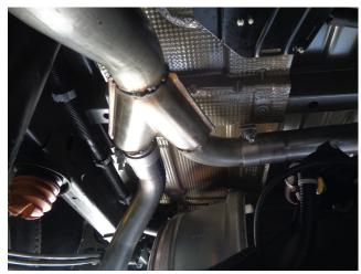
Step 4. Next loosely attach the Driver and Passenger side Extension Pipes to the Muffler Assembly using the supplied 2.50" clamps.
