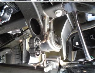
Step 5. As this vehicle was not setup for dual exhaust from the factory, hanger brackets will need to be installed. Install the hanger brackets on the rear frame section using the supplied fastener hardware as shown
