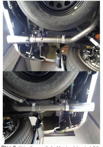
Step 6. Using the supplied rubber insulators install the Tailpipe Assemblies to the Extension pipes fitting the hangers into the installed hanger brackets. Finish by attaching the Tips using the supplied 2.75" clamps. Tips can be adjusted to fit a variety of bumpers.
