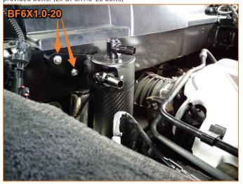
4. Install MM4606-01 hose to the PCV valve port. (1x MM4606-01 hose). Next, install the MM4606-02 hose to the intake manifold port. (1x MM4606-02 hose) Connect MM4606-01 and MM4606-02 to the catch can using the provided worm gear clamps. (2x MM1325-2 worm gear clamps)
