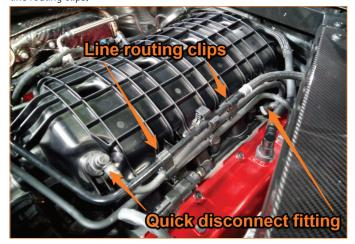
02. Install MM4553-03 hose to the PCV valve port. (1x MM4553-03 hose)
