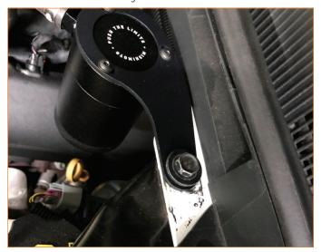
05. Route the hose with the 45-degree fitting from the male fitting on the intake manifold to the "OUT" fitting on the catch can and secure with the provided hose clamp. Route the hose underneath the wiring harness above the valve cover for a clean look. You may trim the open end of the hose if necessary.
