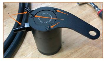
04. Locate and remove the 13mm bolt attaching the fender brace to the firewall on the driver's side of the engine bay. Install the catch can bracket under the bolt and tighten. Note the orientation of the bracket.
