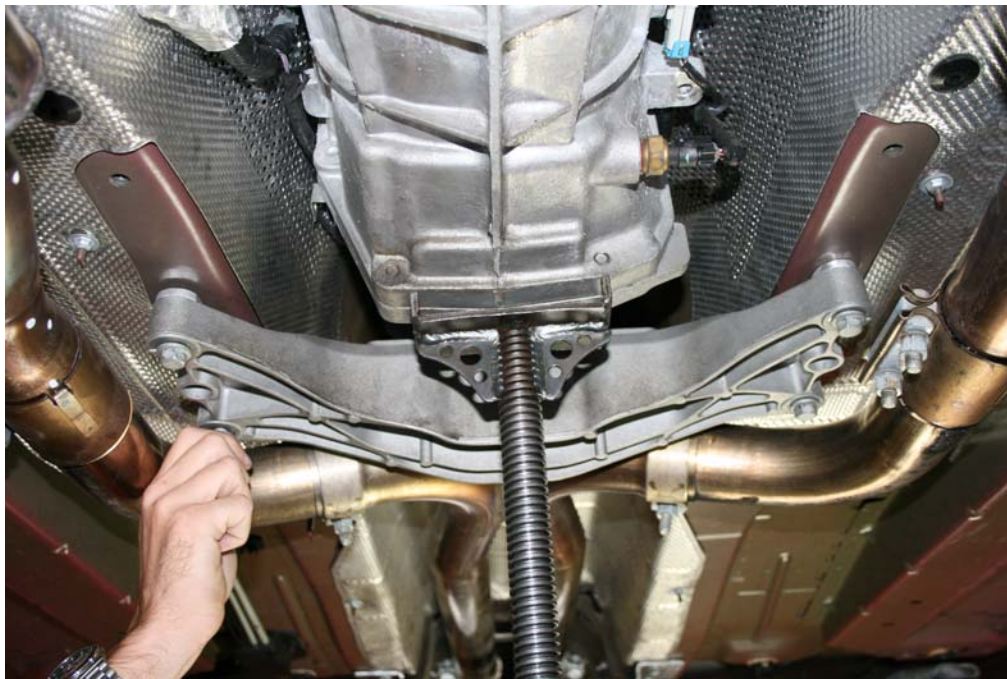
Step 8: Reinstall remaining crossmember bolts
