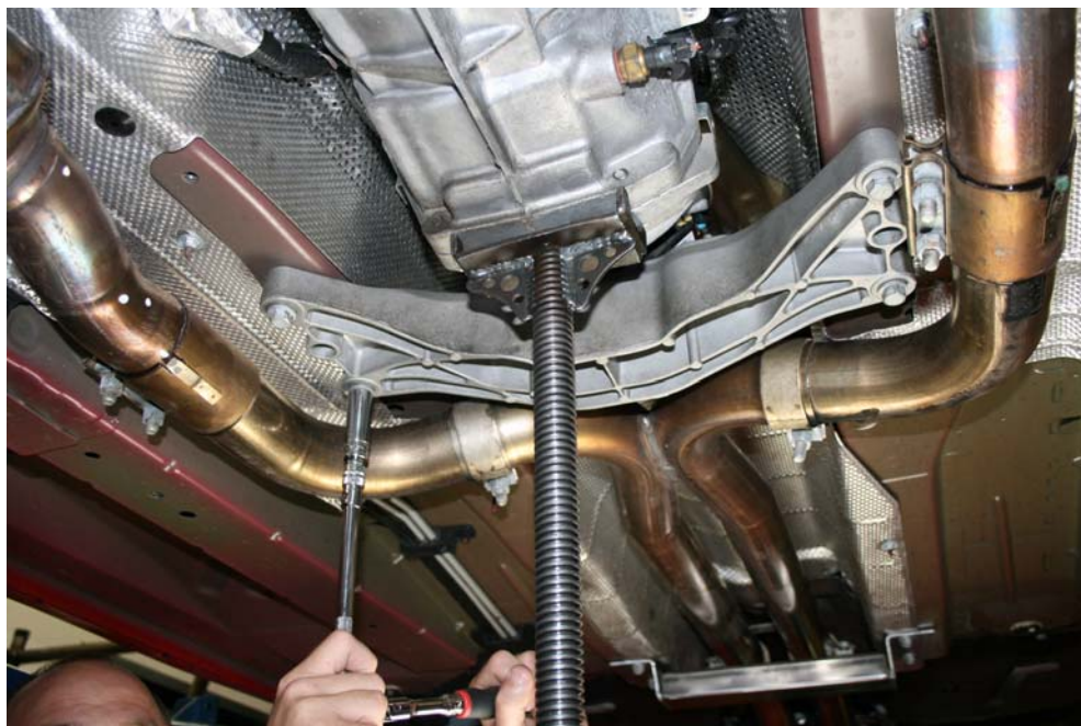
Step 3: Remove transmission crossmember bolts
