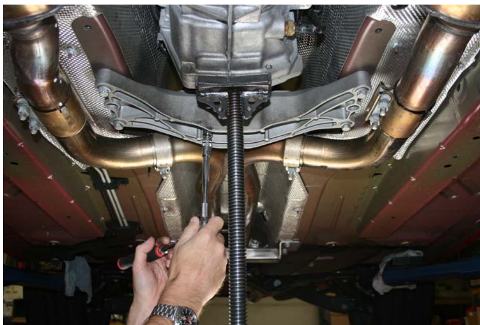
Step 2: Remove transmission mount bolts
