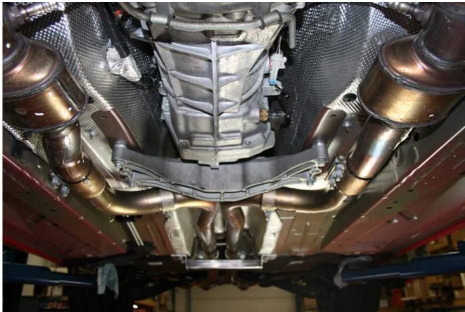
Step 10: Remove support from rear of transmission
