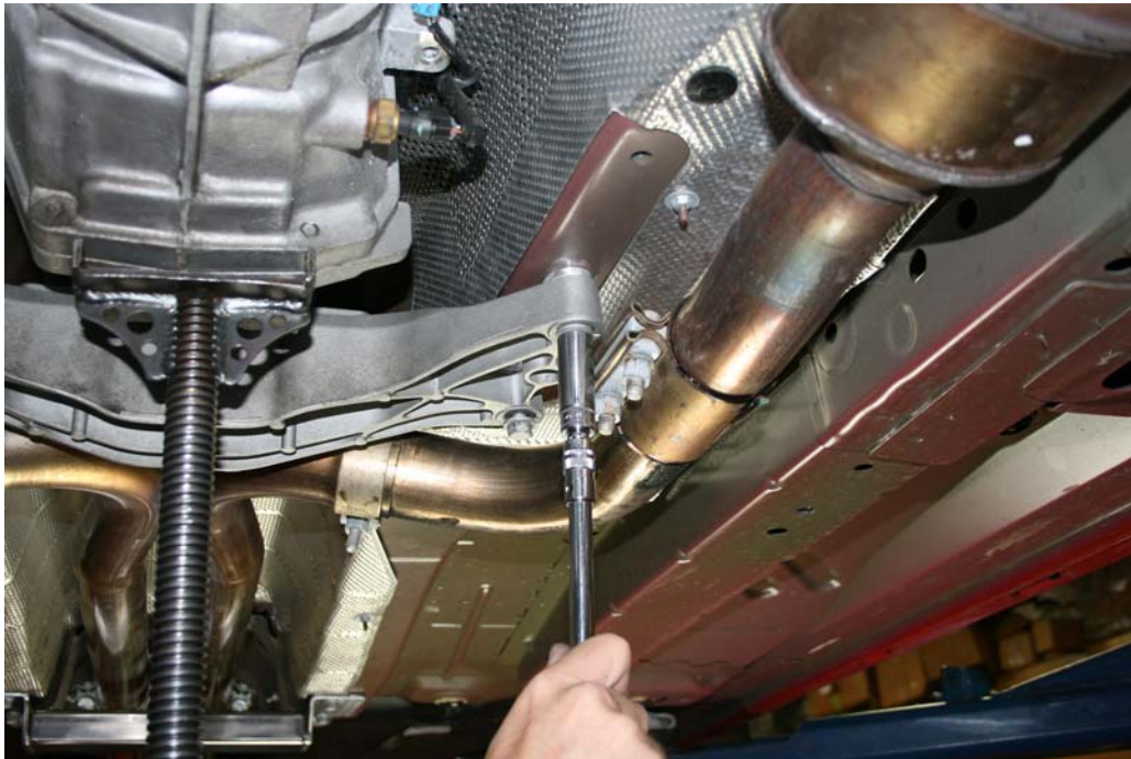
Step 9: Tighten crossmember mounting bolts
