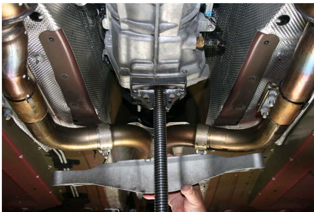
Step 4: Remove transmission crossmember from vehicle
