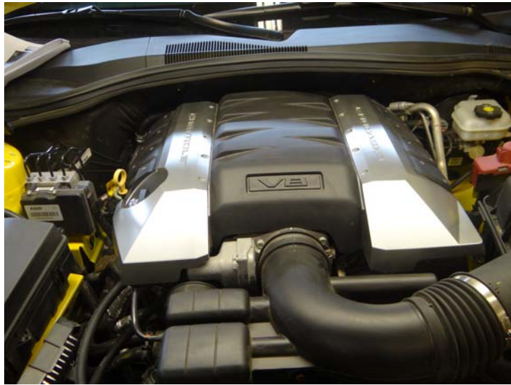
Step 14: Reinstall engine cover and oil fill cap.
