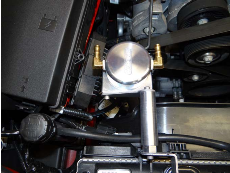
Step 10: Tighten billet clamp.
