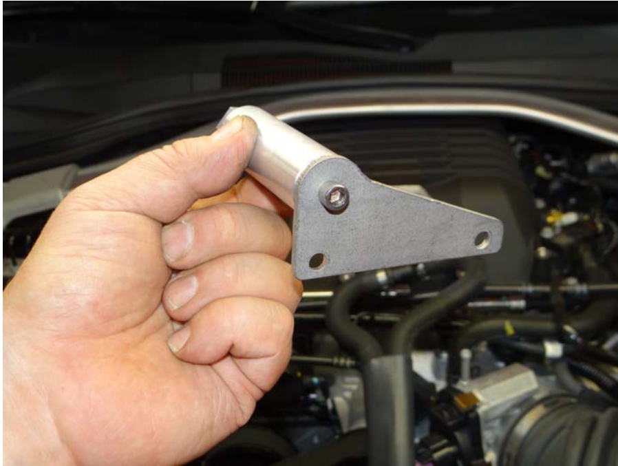
Step 4: Assemble billet mount to stainless clamp mounting bracket using (1) ¼-20 SHCS.
