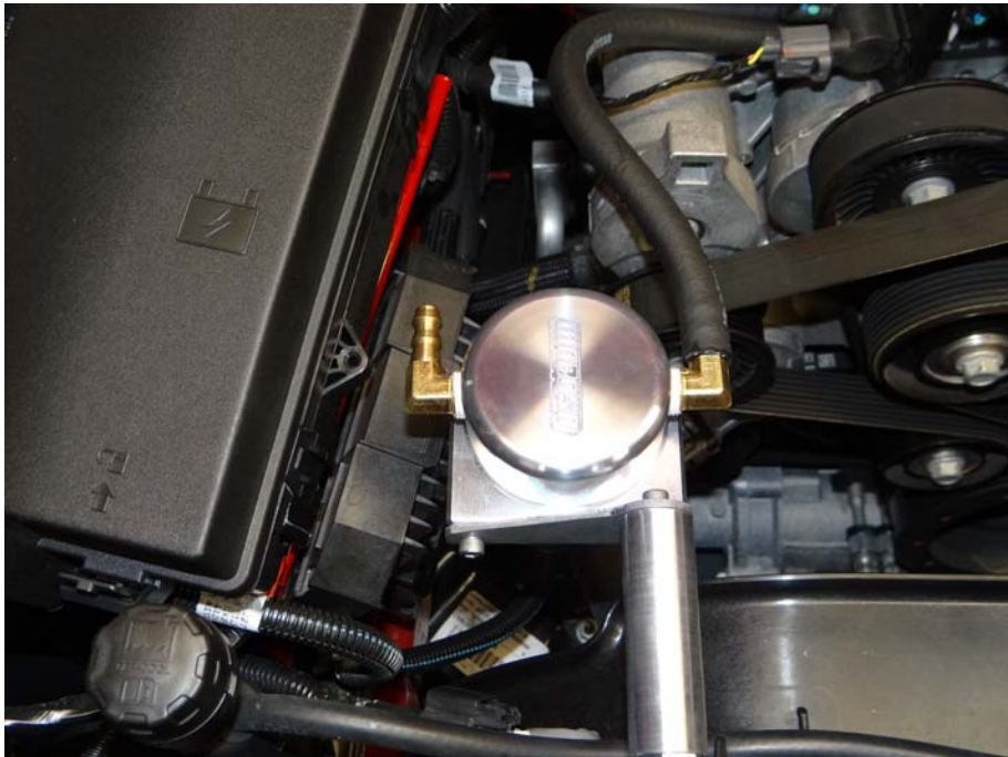
Step 11: Install 3/8 hoses to Air Oil Separator.
