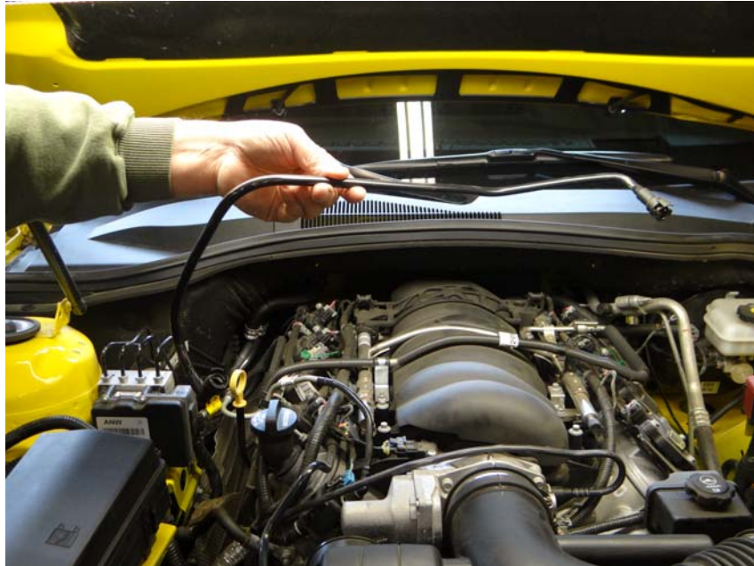
Step 6: Remove PCV line from vehicle.
