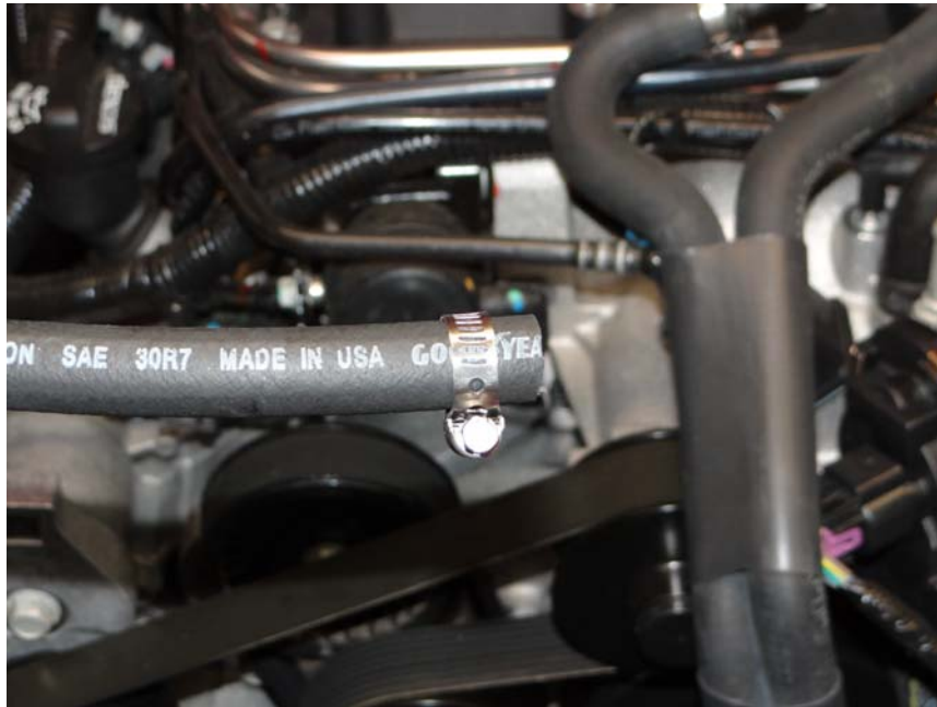
Step 6: Install hose clamp over 3/8 hose.
