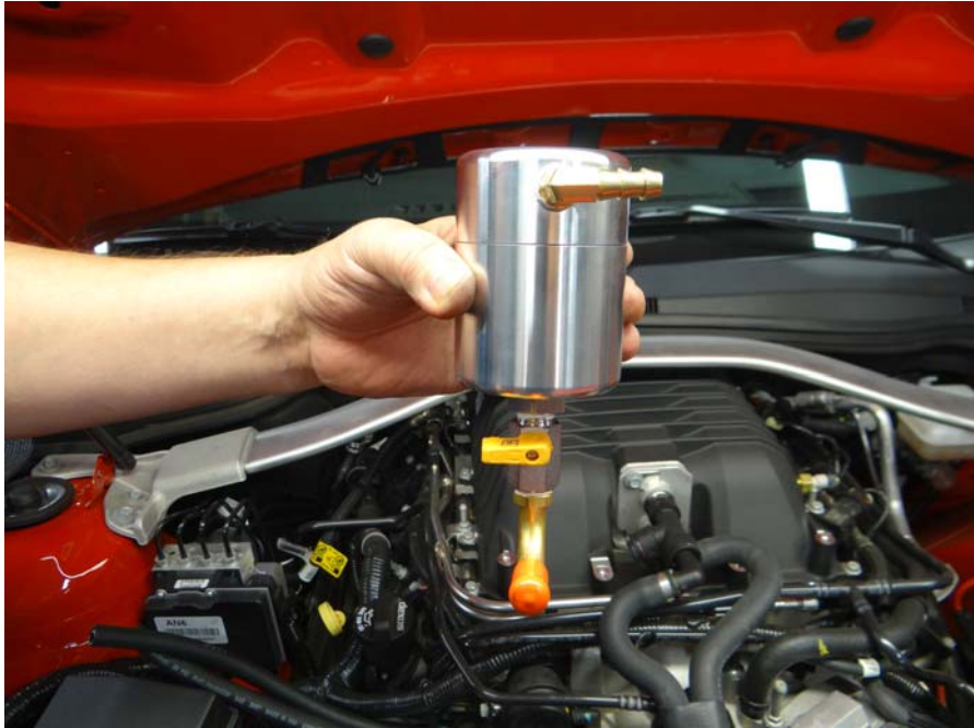
Step 8: Assemble ball valve, 90 degree drain and drain cap as shown using Teflon Tape.
