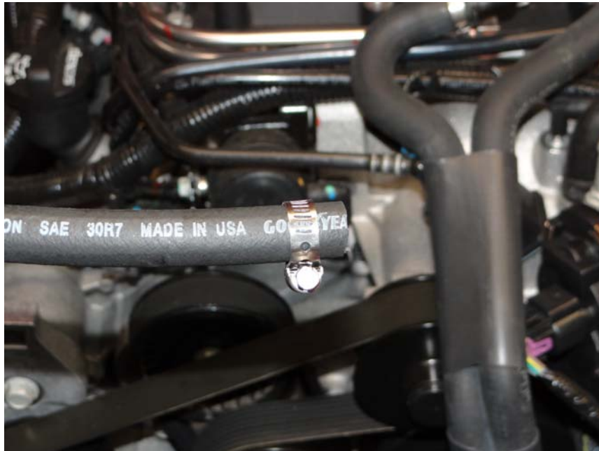
Step 3: Install hose clamp over 3/8 hose.
