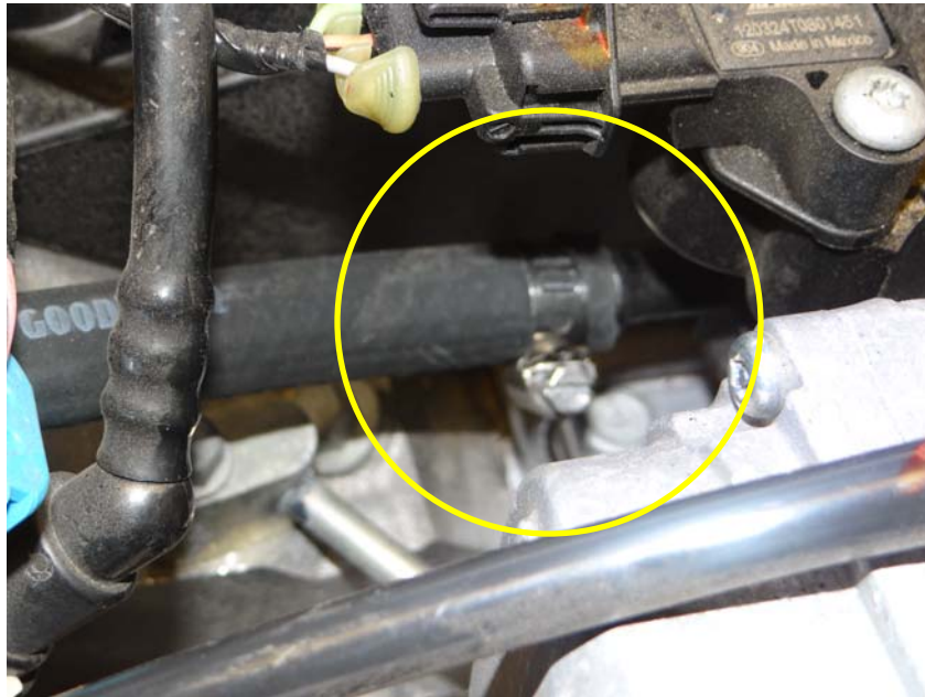
Step 12: Install hose over intake nipple.
