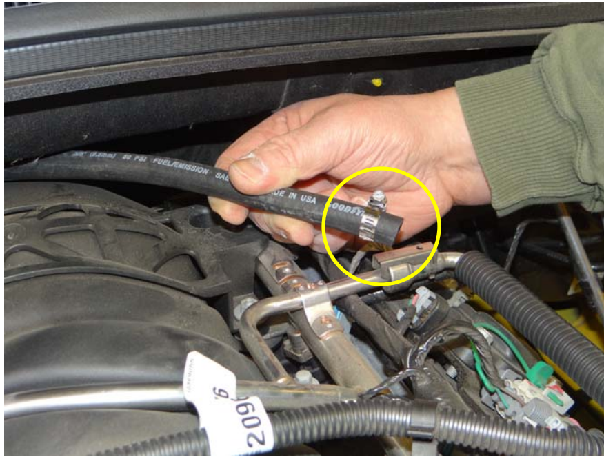
Step 8: Install hose clamp.
