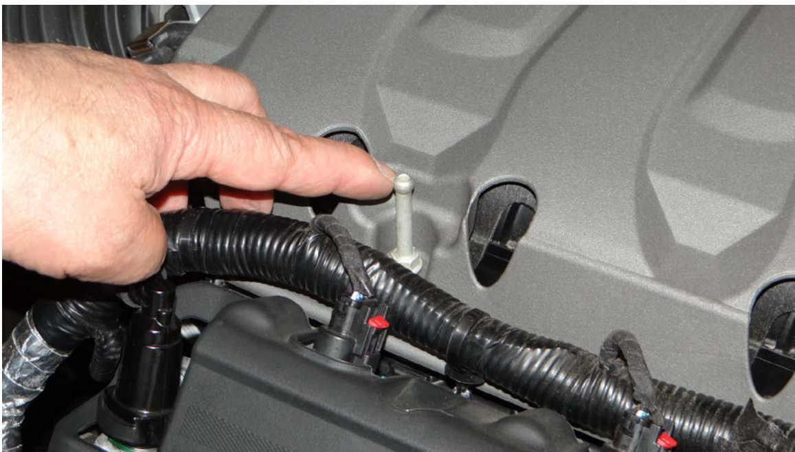
Step 3: Remove intake cover bolts.
