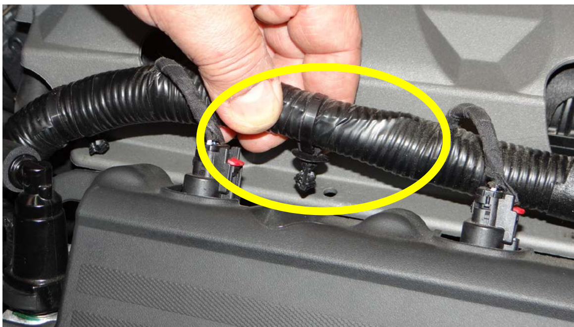
Step 4: Remove wiring harness from intake cover.
