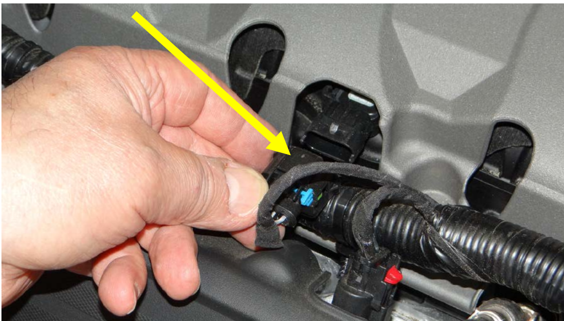
Step 5: Remove wiring harness plug as shown.
