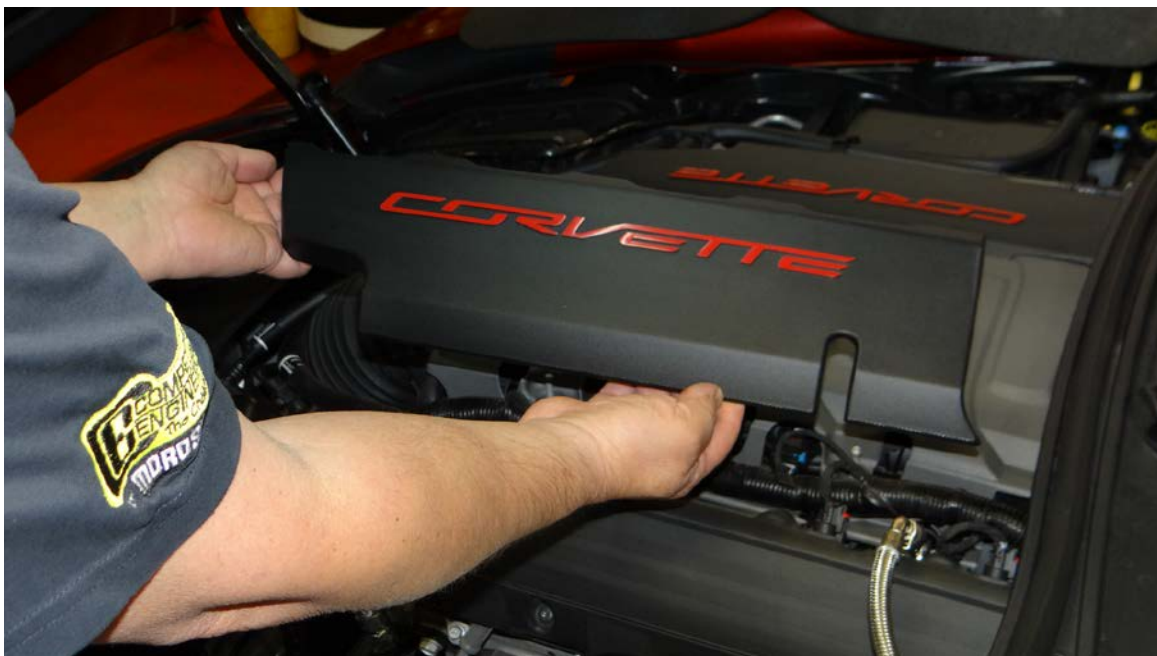
Step 1: Remove driver's side engine cover.
