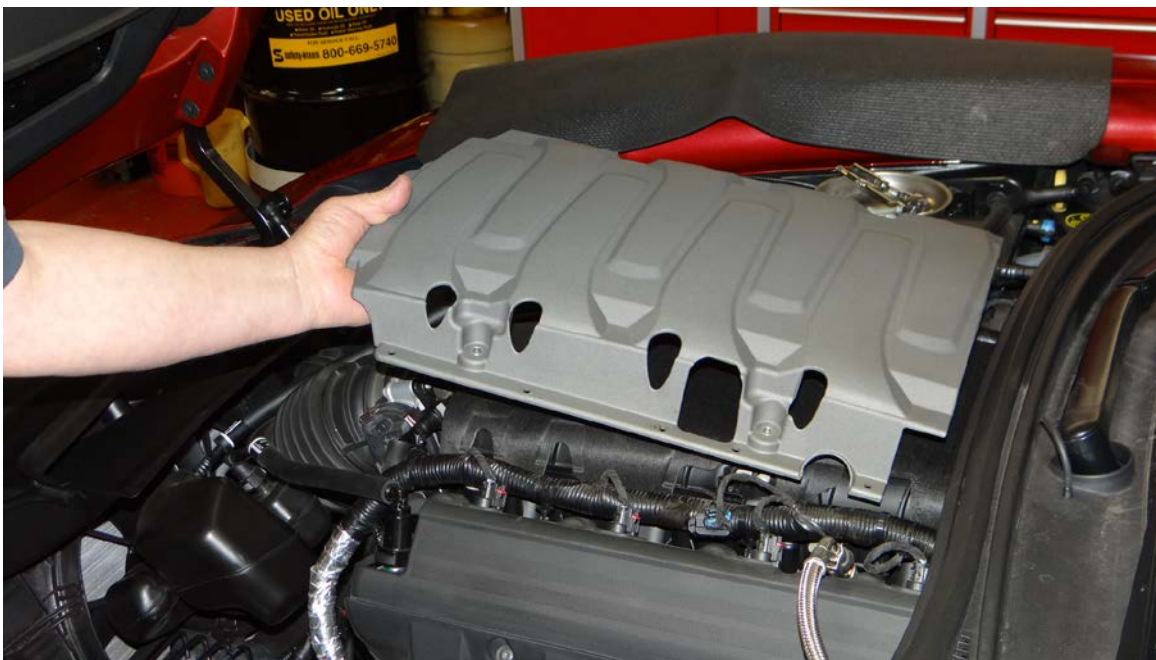
Step 6: Remove intake cover from vehicle.
