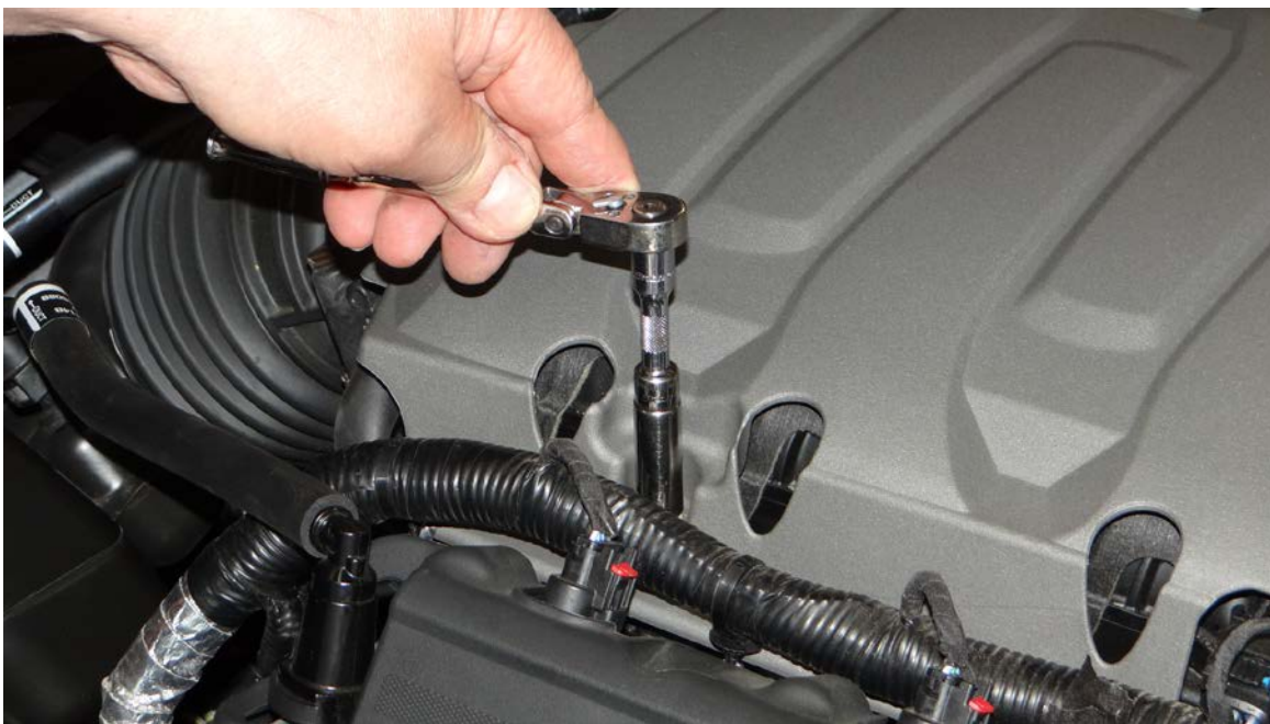
Step 3: Remove intake cover bolts.
