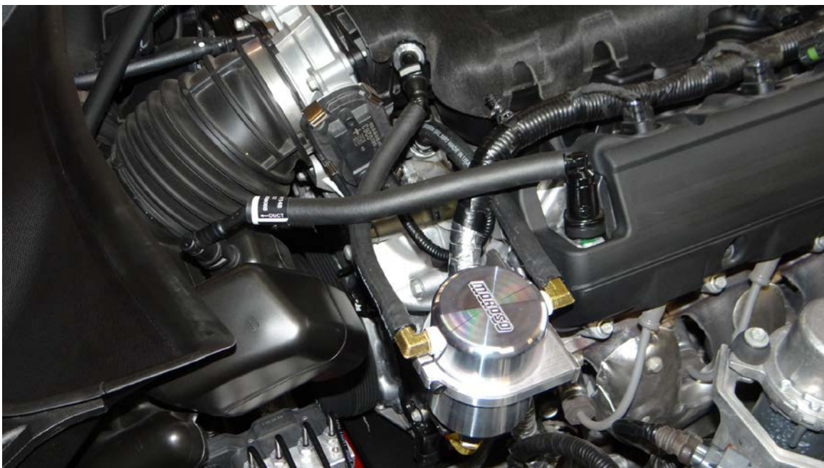
Step 21: Install hoses to Air Oil Separator.
