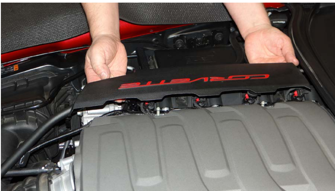
Step 2: Remove passenger's side engine cover.
