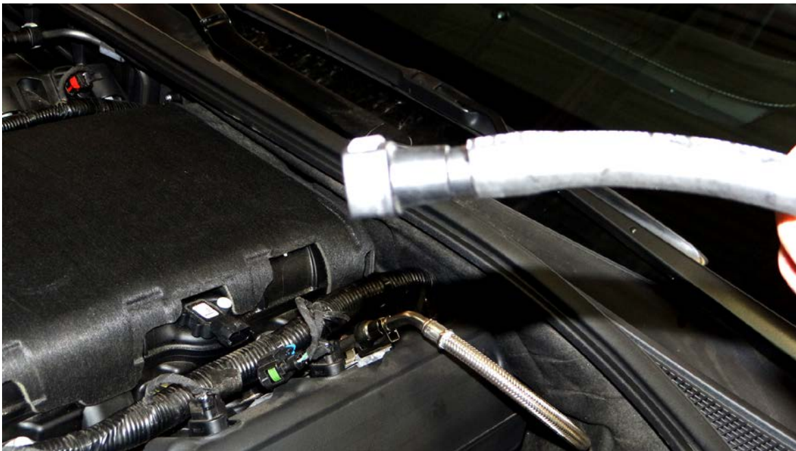
Step 14: Using hose with straight fitting, re-install fitting to lifter valley nipple, as shown in following illustration.
