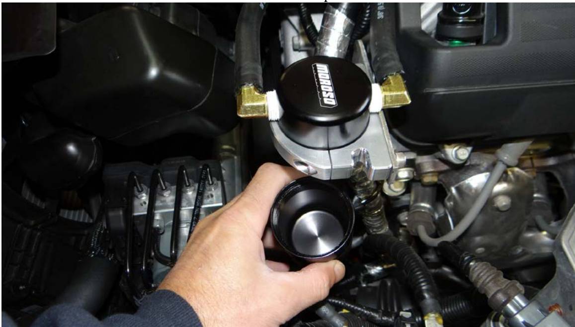
To drain Air Oil Separator remove bottom cup.
