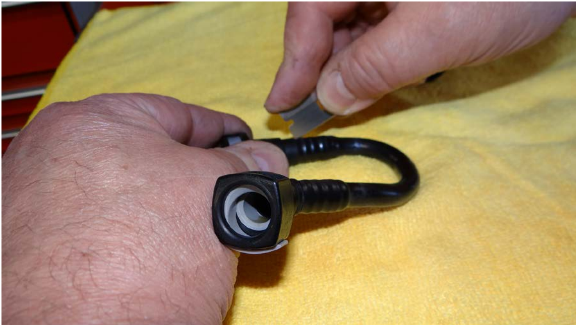
Step 11: Using razor blade, slice PCV line, and remove both fittings.
