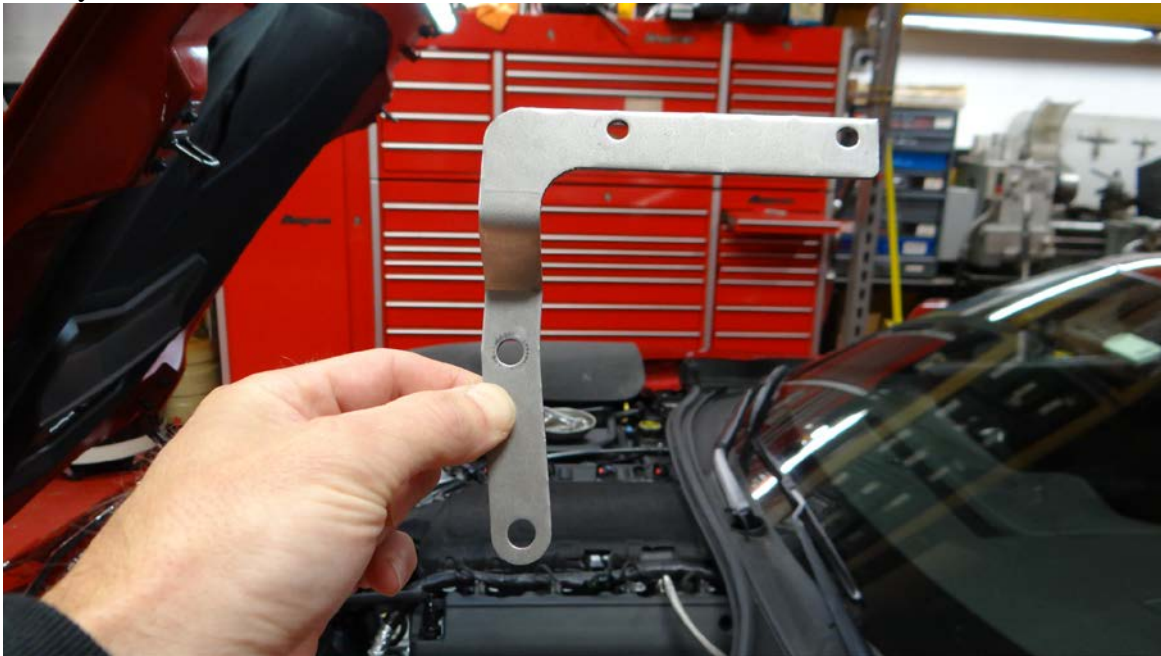
Step 9: Install stainless mounting bracket using (2) 8mm x 25mm HHCS as shown in following illustrations.
