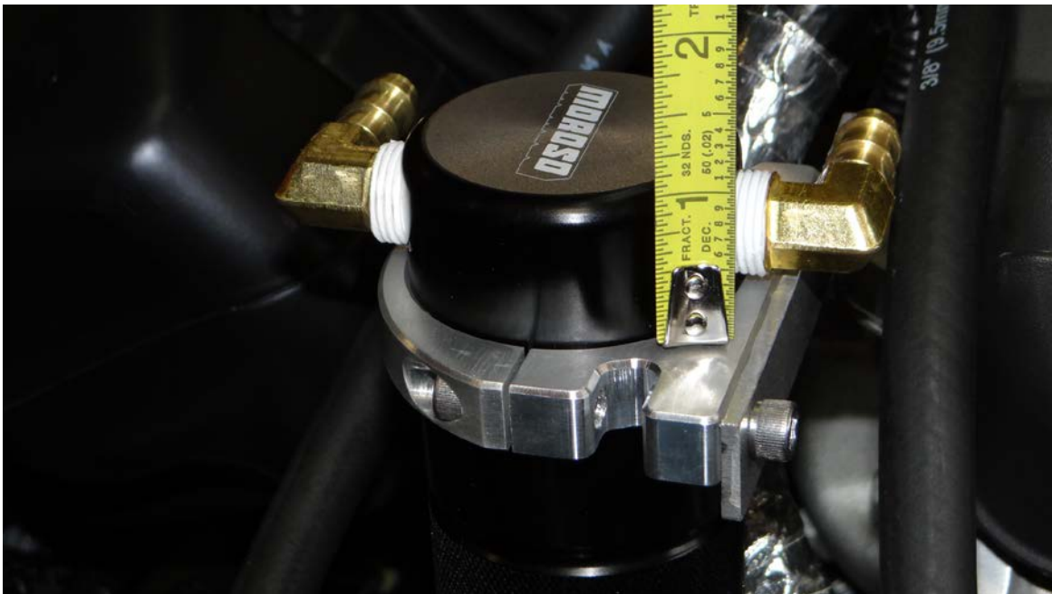
Step 20: Set height @ 1" -1 1/8" as shown and tighten clamp.
