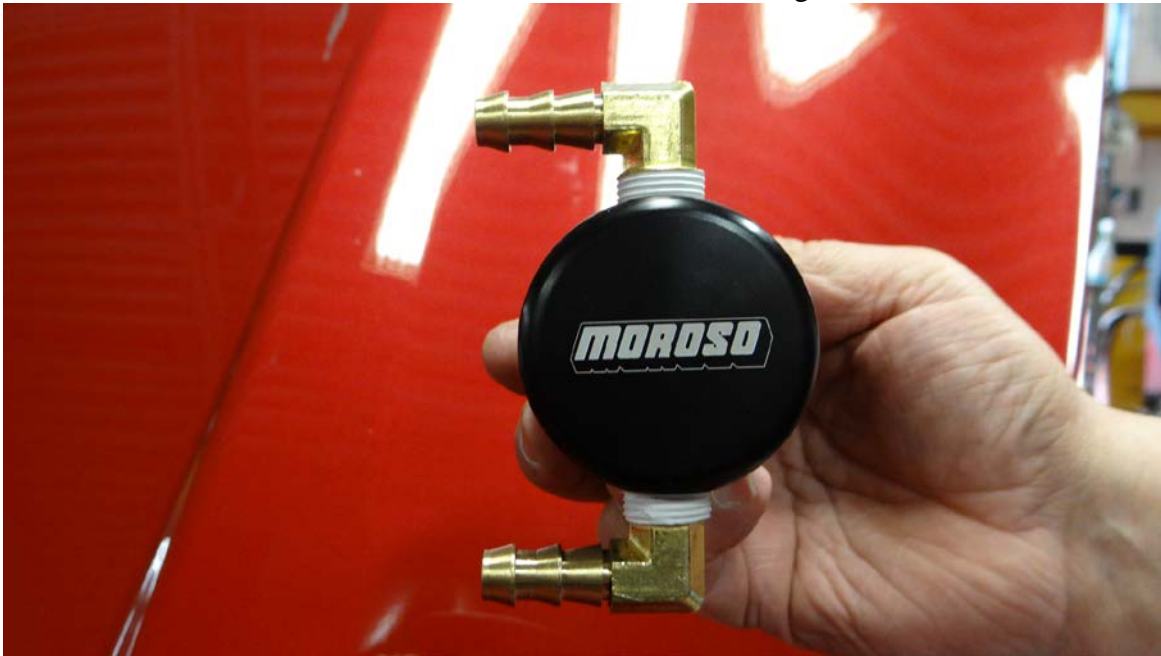
Step 18; Assemble Air Oil Separator as shown using Teflon Tape on all fittings.
