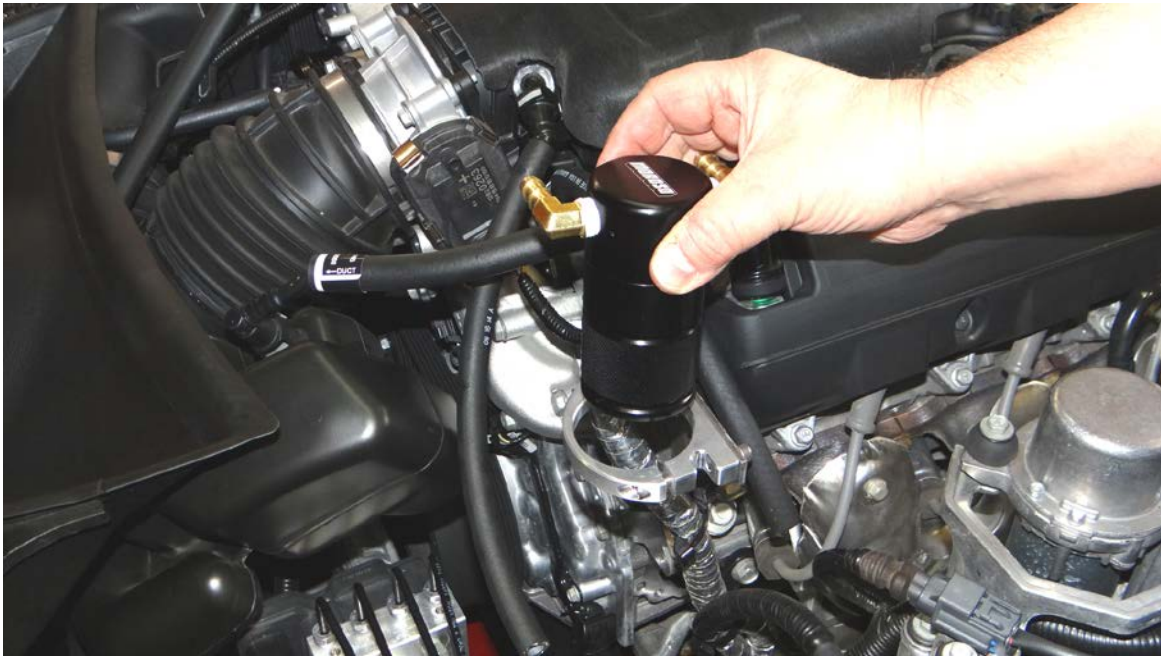
Step 19: Insert Air oil Separator into billet clamp as shown.
