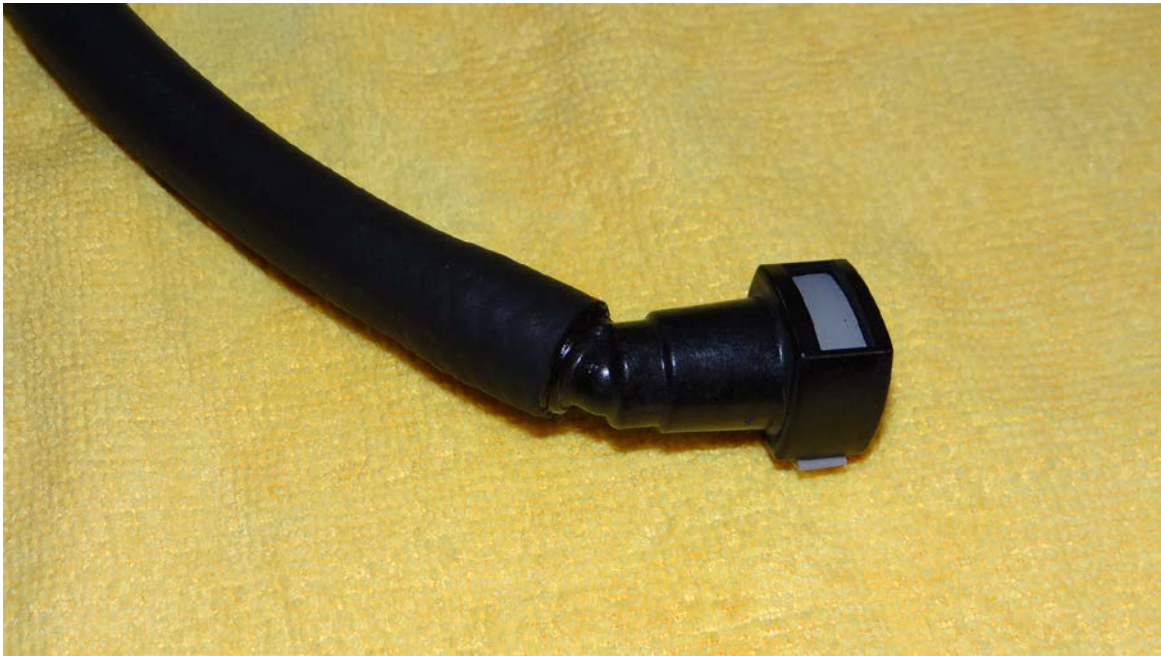
Step 13: Insert fitting into length of hose provided in kit as shown.
