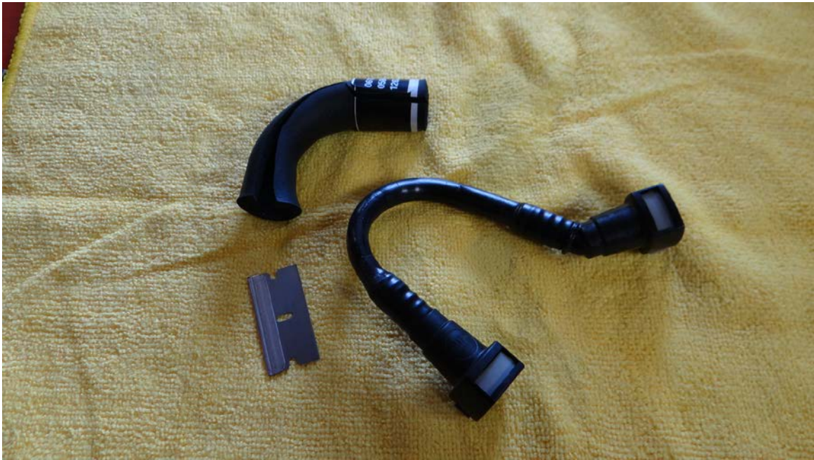
Step 10: Using a razor blade cut outer jacket from PCV line as shown.
