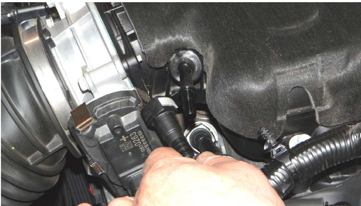
Step 7: Locate and remove PCV line from vehicle as shown.
