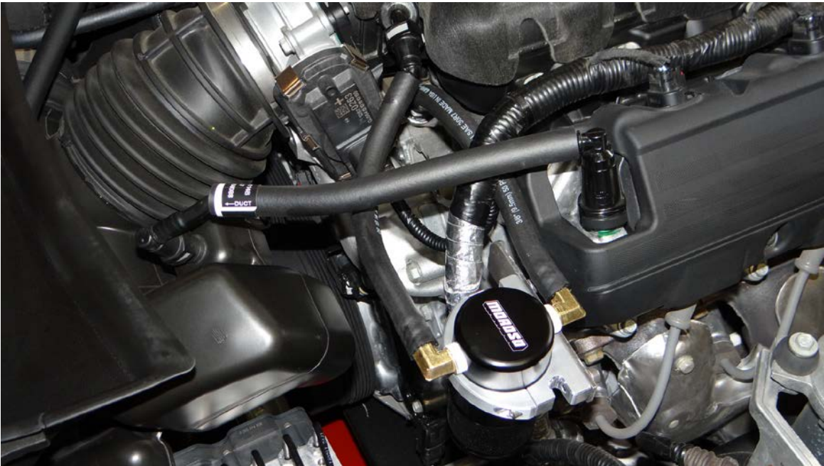
Step 24: Install hose to Air Oil Separator.
