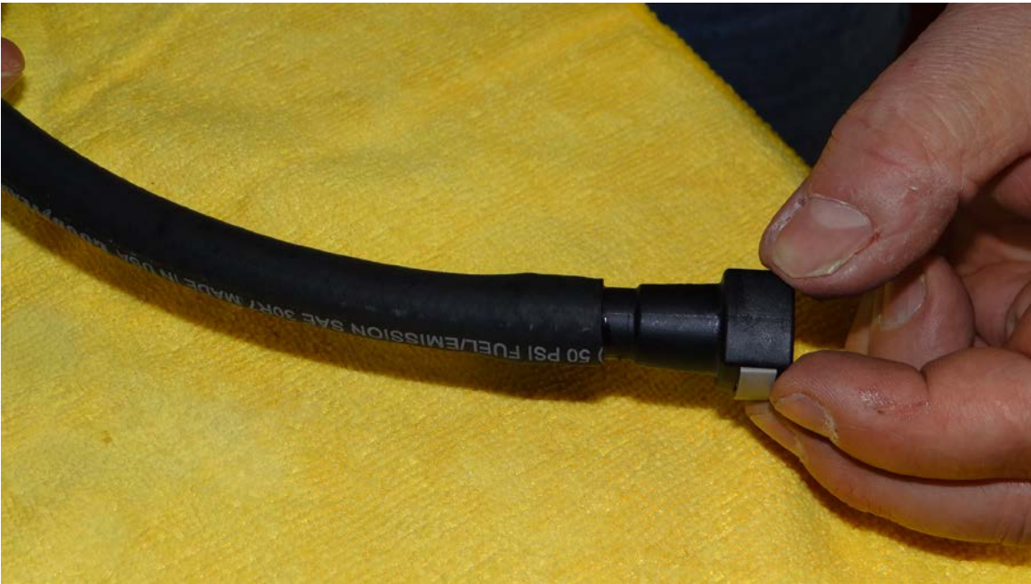
Step 12: Insert fitting into length of hose provided in kit as shown.
