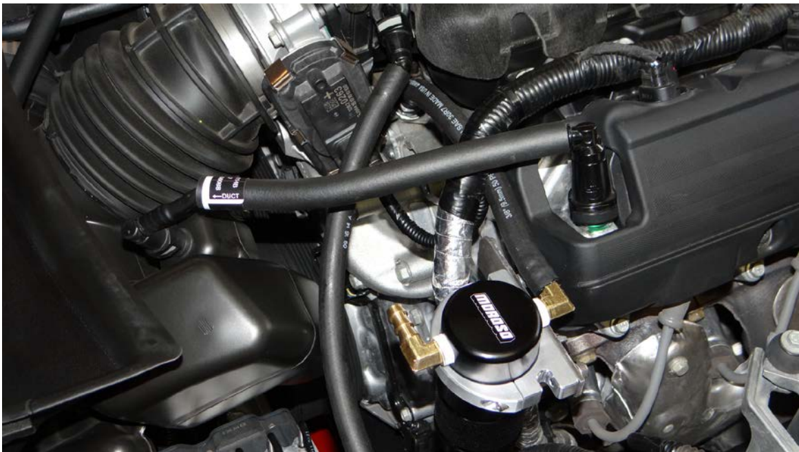
Step 22: Install hose to Air Oil Separator.
