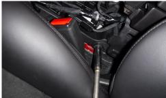
• Using a 10mm deep socket, remove the bolts on each side of the console.
