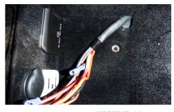
• Pull your wires through the hole in the center console.
