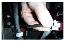
• Disconnect the 2 electrical connectors on the back of the panel.
