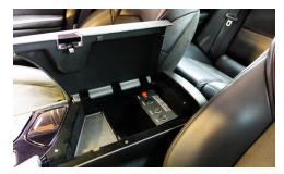
Remove the 2x4 supporting the console. Push the switch panel down in the compartment. You
