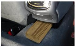
• Lift the rear of the console and place a section of 2x4 underneath. This is to create a gap between the bottom of the console storage compartment and the air conditioning ducting that feeds the rear air vents.
