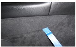
• Using the body tool, pry the trim panel on the passenger side from the center console then pull it from the retaining clips.
