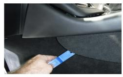
• Using the body tool, pry the trim panel on the driver side of the center console then pull it from the retaining clips.
