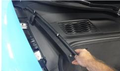
Remove the trim panels on each side of the vehicle by pulling them from the clips securing them to the body.
