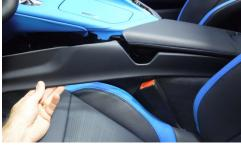
• Remove the side trim panel by pulling it from the clips holding it to the center console.
