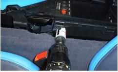
• On the side of the console compartment, the access hole needs to be as far forward and as high as possible. Before drilling, remove the switch panel as not to damage it or any switches.
