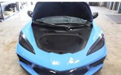
• Reinstall the 3 trim panels around the front storage compartment.
