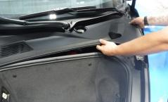
• Remove the cowl panel covering the battery by pulling it from the clips securing it to the body.
