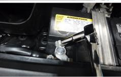
• Disconnect the negative battery terminal by using a 10mm socket to loosen the nut.
