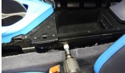
• Using a 1" hole saw, drill the access hole.
