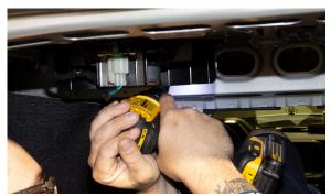
Use a 5/16" drill bit to drill the holes you marked on the rear seat brace.
