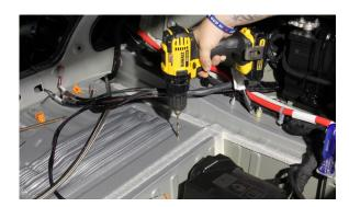
Check under the area you are drilling to ensure it is clear of any electrical or fuel systems components. If it is clear, use a 3/8" drill bit to drill the holes you marked on the trunk floor.
