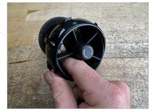
Use 1 finger to loop around back of vent core as shown
