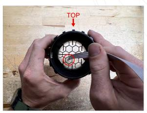
With "TOP" at 12 o'clock position, feed display cable through vent housing as shown
