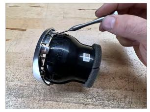
Use a small screw driver to release trim clips from vent housing (2 screw drivers may be required as tabs are stiff)
