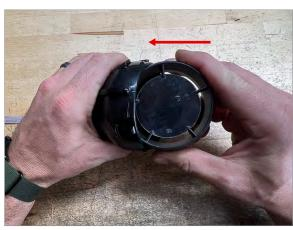
Insert display enclosure into vent as shown
