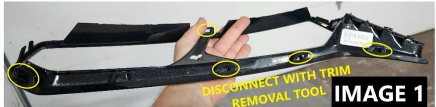
2. Use a trim removal tool to remove the clips retaining the taillight trim. **IMAGE 1**
