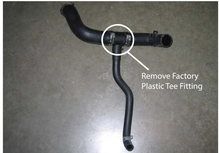
Factory Coolant Lines
