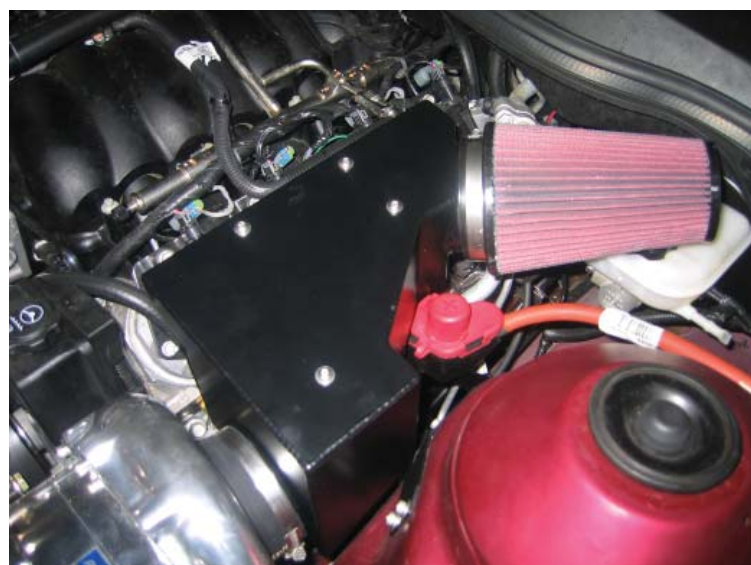
Air Inlet Box Installed
