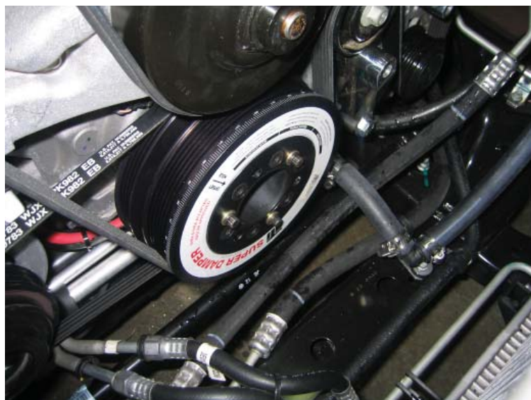
ATI PP Damper Installed
