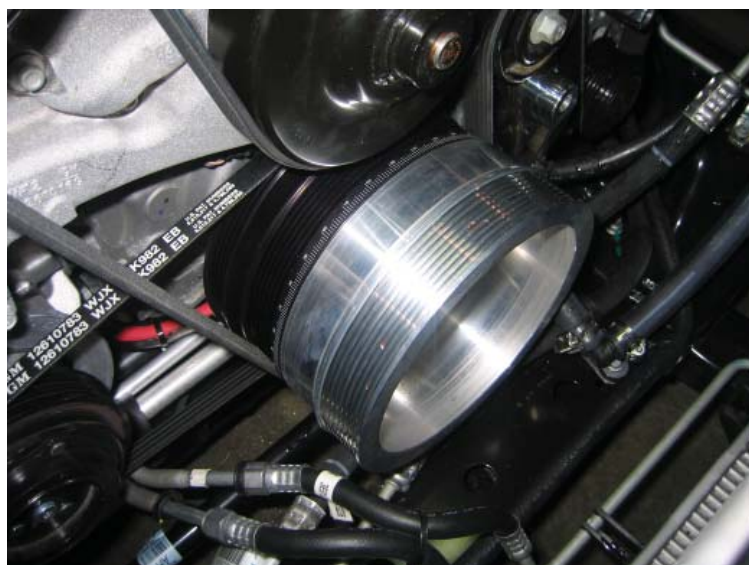
Crank Pulley Installed
