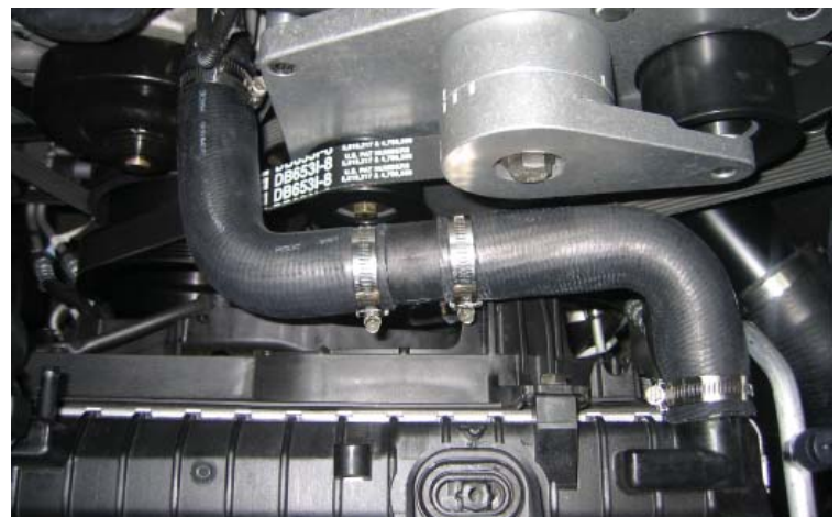
New Coolant Lines Installed
