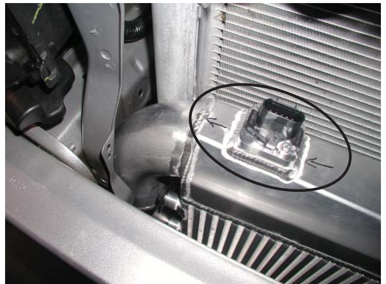
Intercooler Installed, Closeup of MAF Installed (Passenger's Side View)
