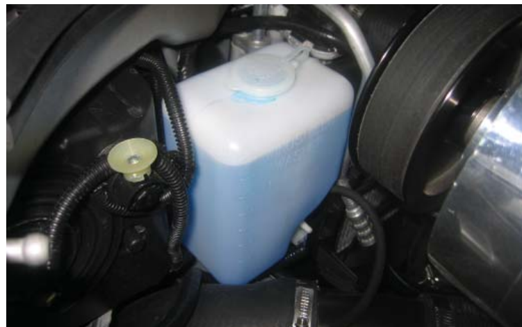
Windshields Washer Reservoir Installed
