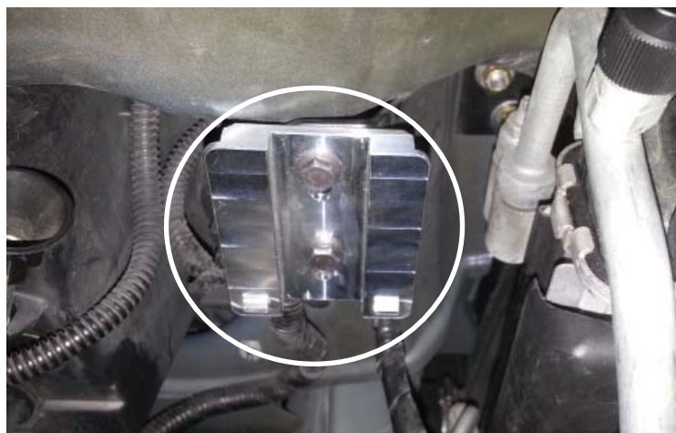
Windshield Washer Reservoir Brackets Mounted
