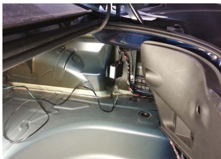
Trigger Wires and Trunk Fusebox
