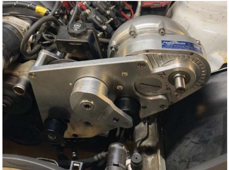
Main Bracket Installed
