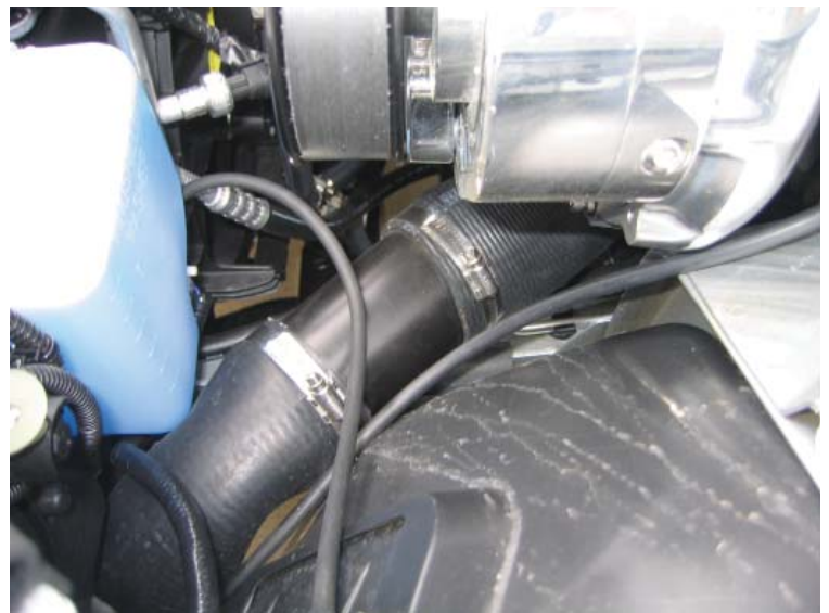
Upper Driver's Side Intercooler Tubing Installed
