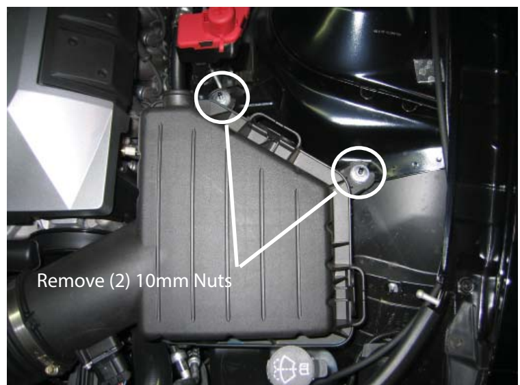
Remove Air Cleaner Box Fasteners
