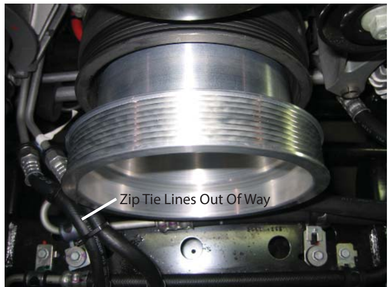
Crank Pulley Installed
