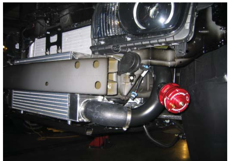
Lower Intercooler Tubing & Race Valve Installed
