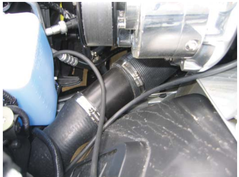
Upper Driver's Side Intercooler Tubing Installed
