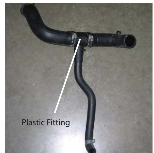
Upper Coolant Line Removed
