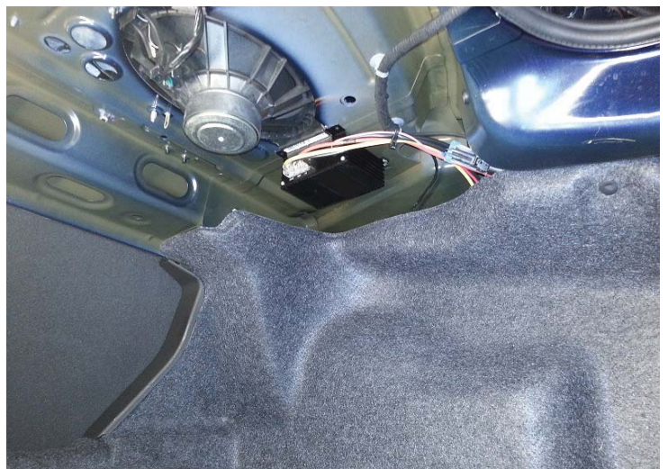
Fuel Pump Booster Installed
