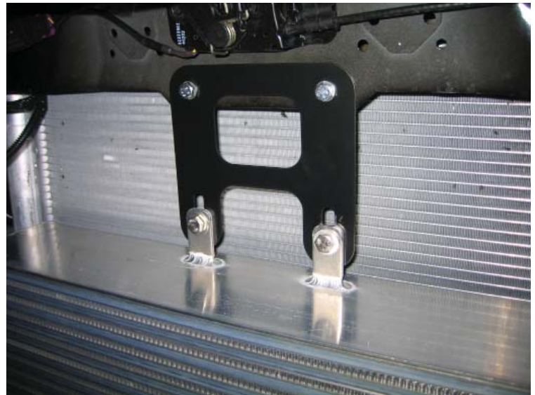
Upper Intercooler Bracket Installed
