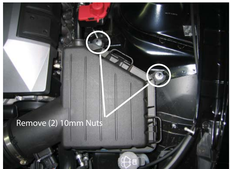
Remove Air Cleaner Box Fasteners
