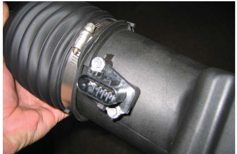
Remove Factory MAF From Intake Tube
