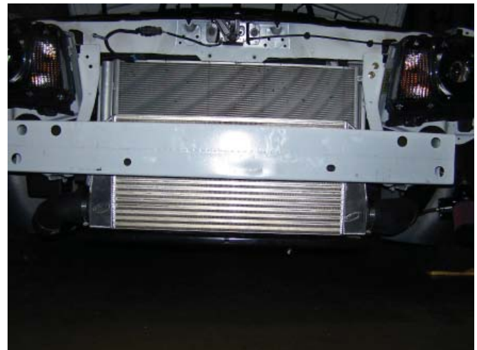
Intercooler & Bumper Support Installed
