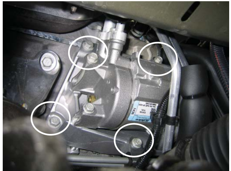
Remove (4) A/C Compressor Bolts
