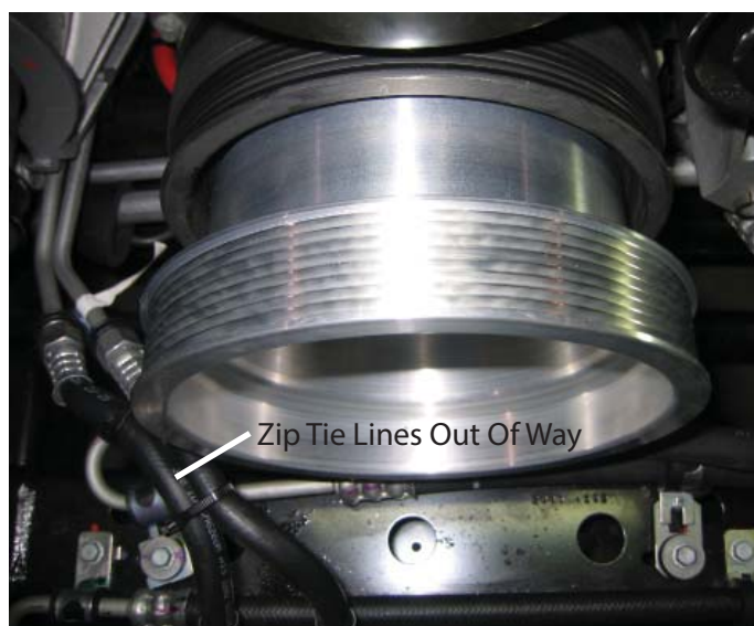
Crank Pulley Installed
