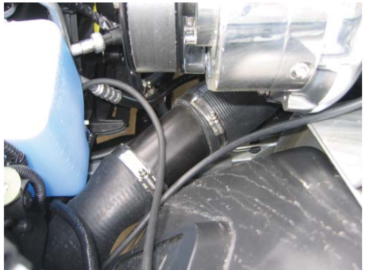
Upper Driver's Side I/C Tubing Installed
