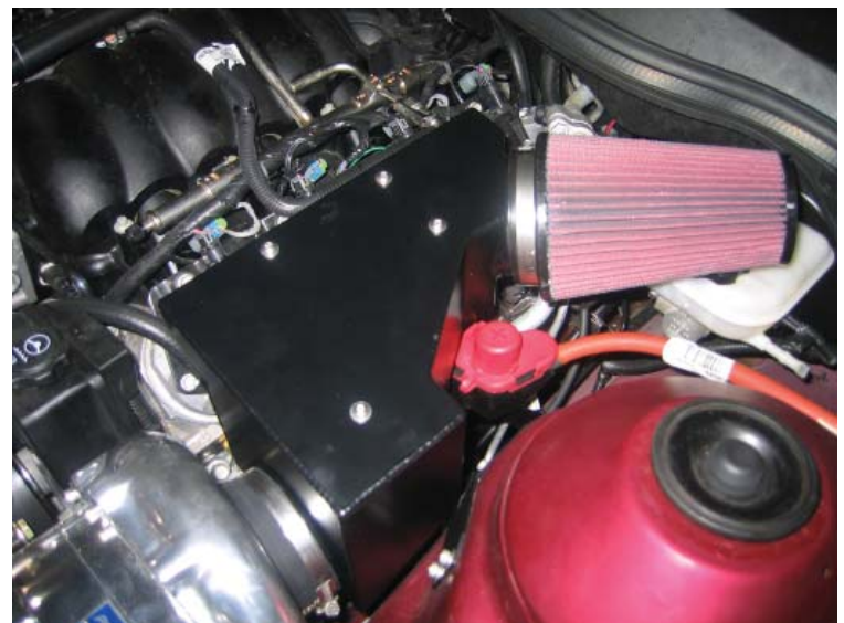
Air Inlet Box Installed
