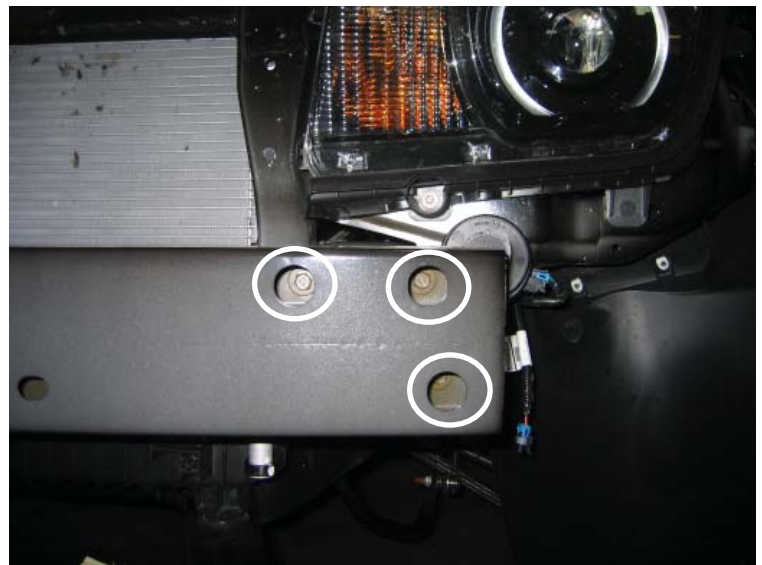
Remove Front Bumper (Driver's Side Fasteners)
