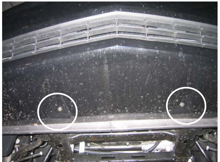
Lower 10mm Screw Removal (2X)
