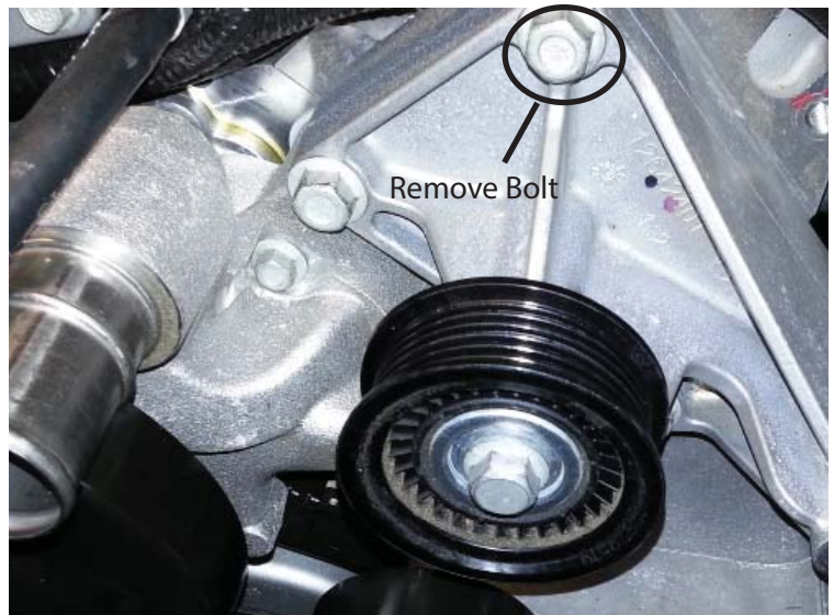
Remove Bolt From Idler Bracket
