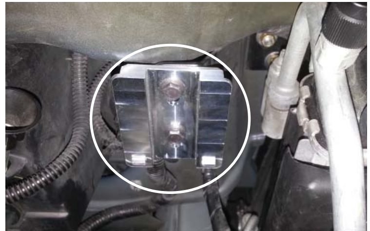
Windshield Washer Reservoir Brackets Mounted
