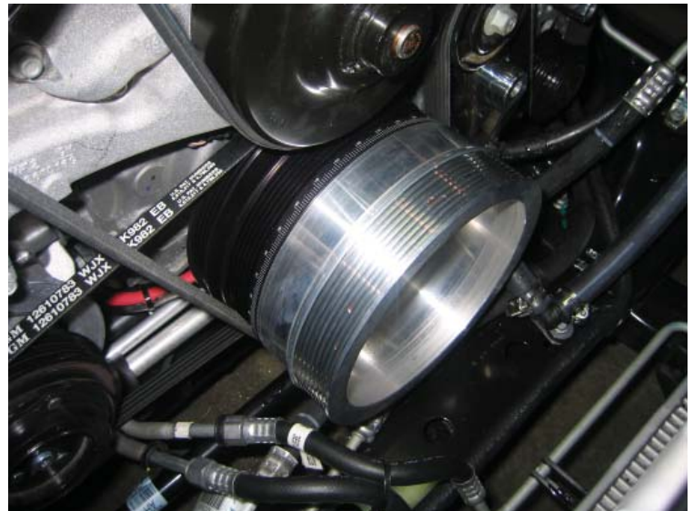
Crank Pulley Installed
