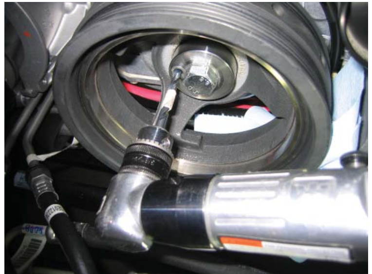
Drill Fixture In Place
