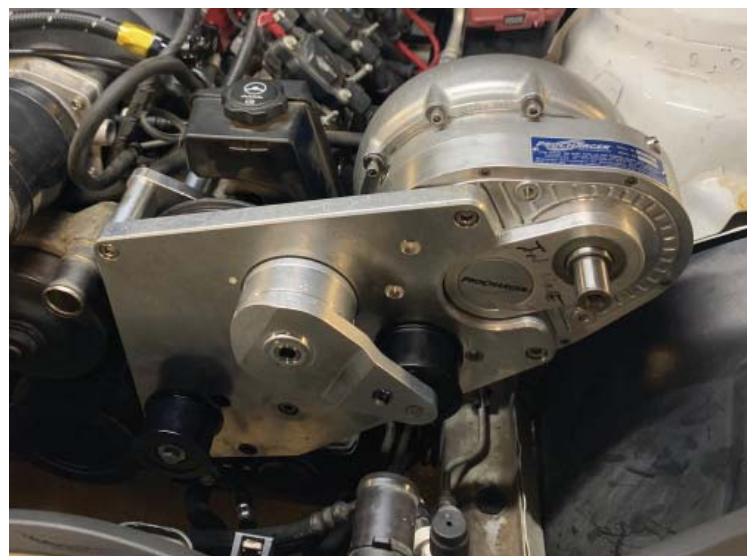
Main Bracket Installed
