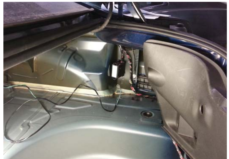
Trigger Wires and Trunk Fusebox
