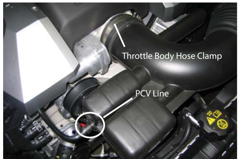
Disconnect PCV Line and Loosen Hose Clamp
