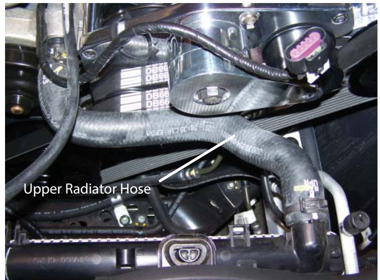
Remove Upper Coolant Hose
