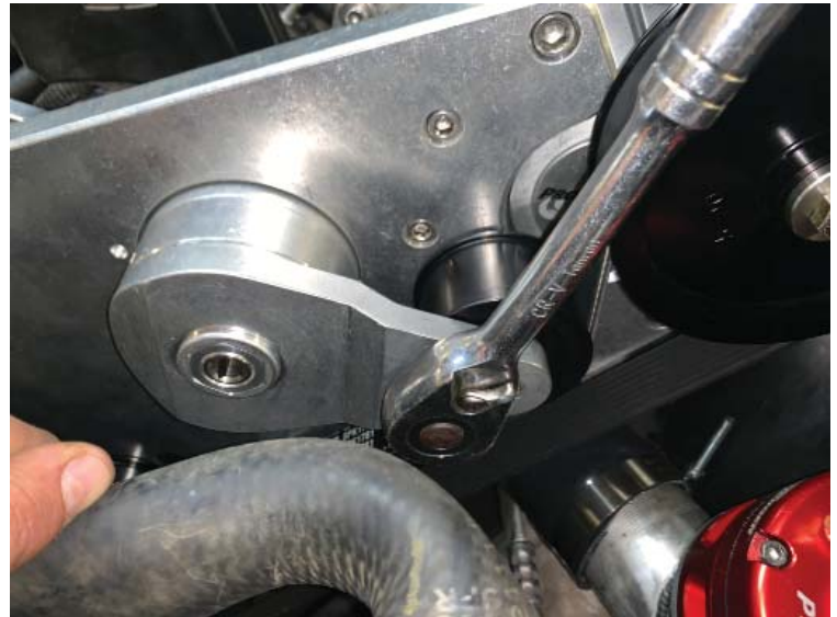
Rotate Tensioner Counter Clockwise
