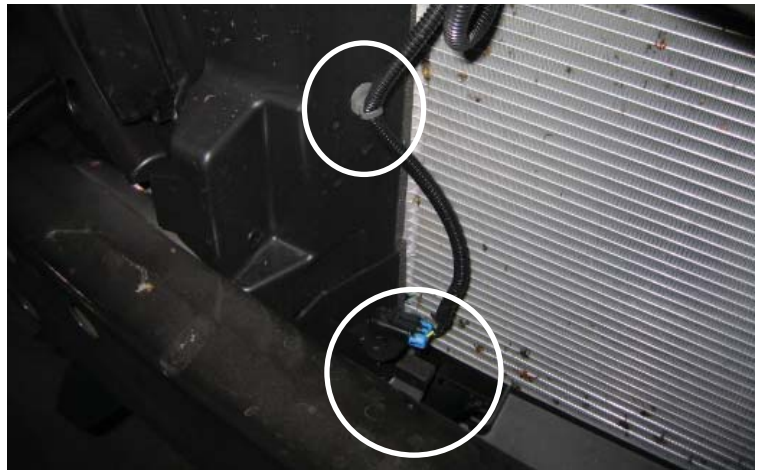
Unclip Wiring Harness and Temp. Sensor
