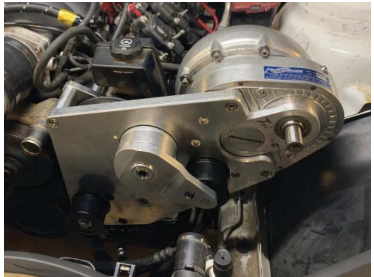
Main Bracket Installed
