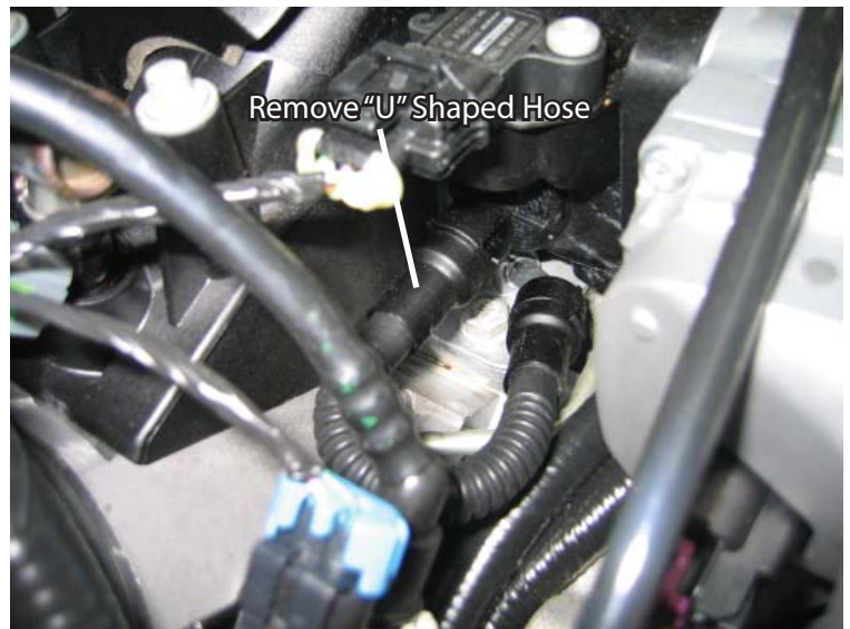
Remove "U" Shaped Hose Remove Factory PCV Hose
