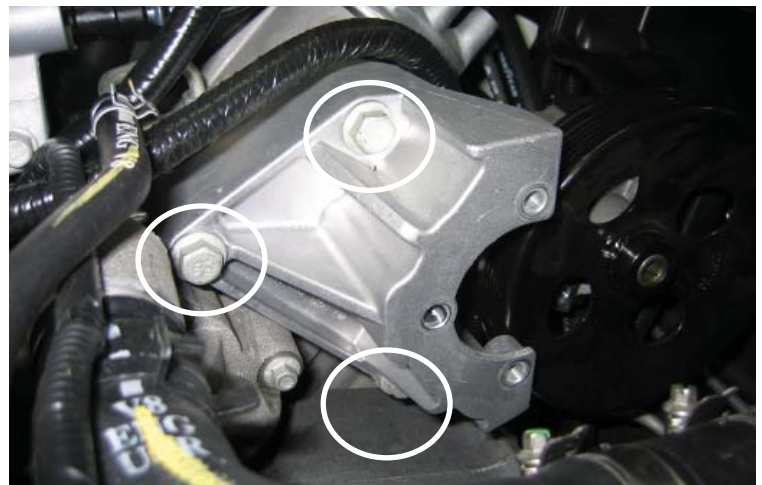
Remove Power Steering Pump Bracket Bolts (3X)
