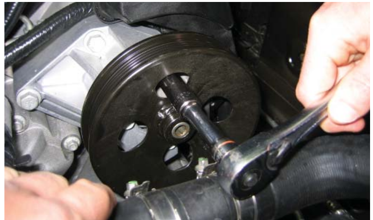
Remove Power Steering Pump Bolts (3X)
