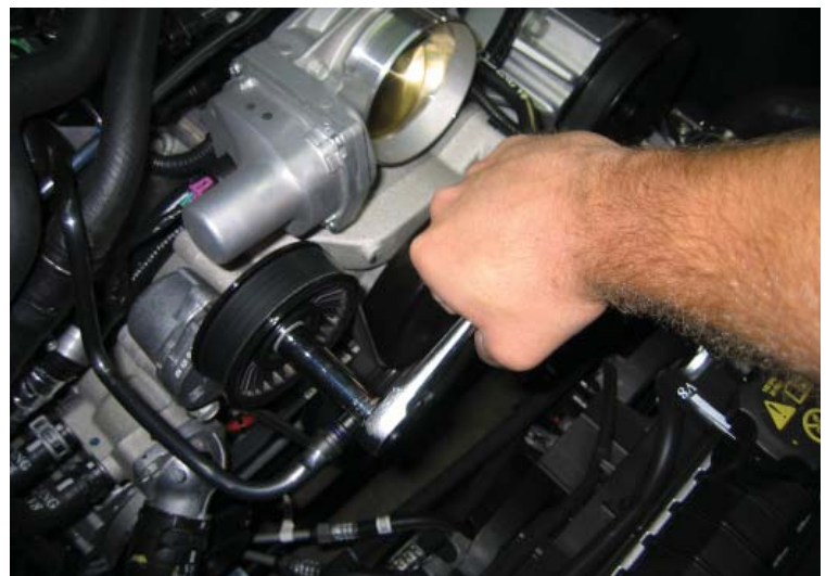
Loosen Tensioner and Remove Accessory Belt
