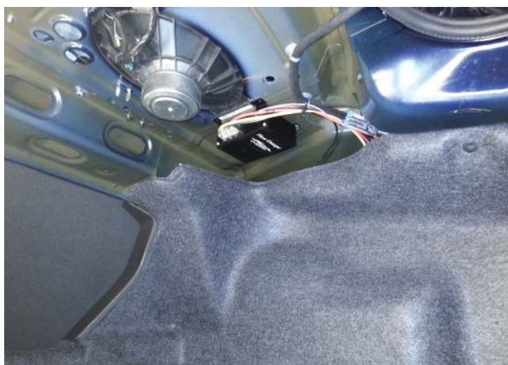
Fuel Pump Booster Installed
