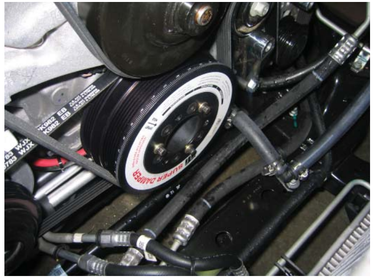
ATI PP Damper Installed
