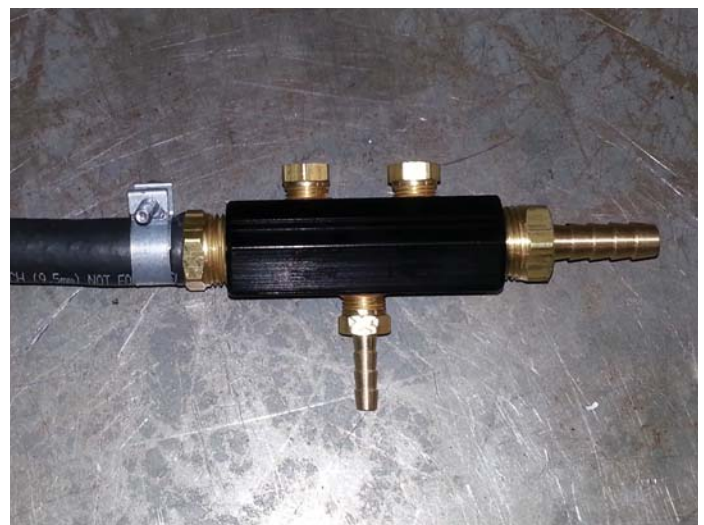
Vacuum Manifold Assembled
