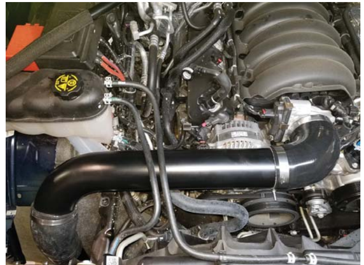
Tubing To Throttlebody Installed
