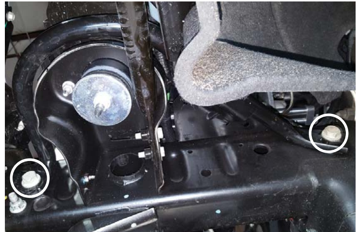
2016: Remove Tubular Frame Rod
