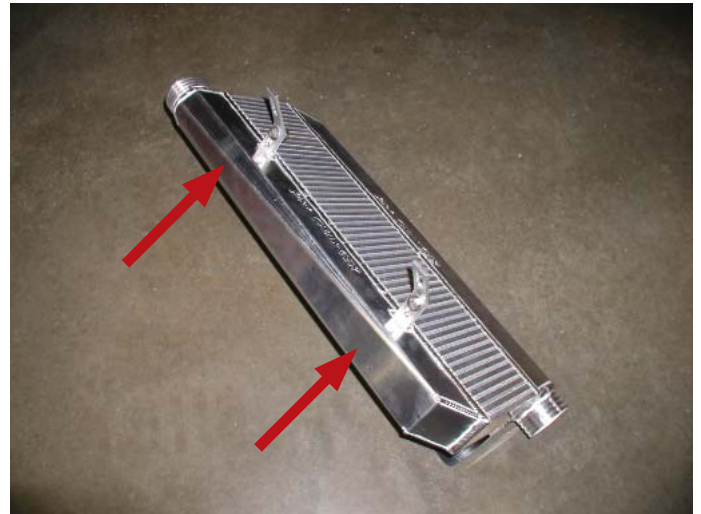
Front Intercooler Brackets Installed
