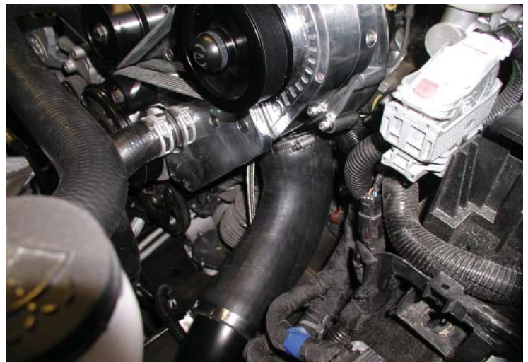
Coupler Connection At Supercharger
