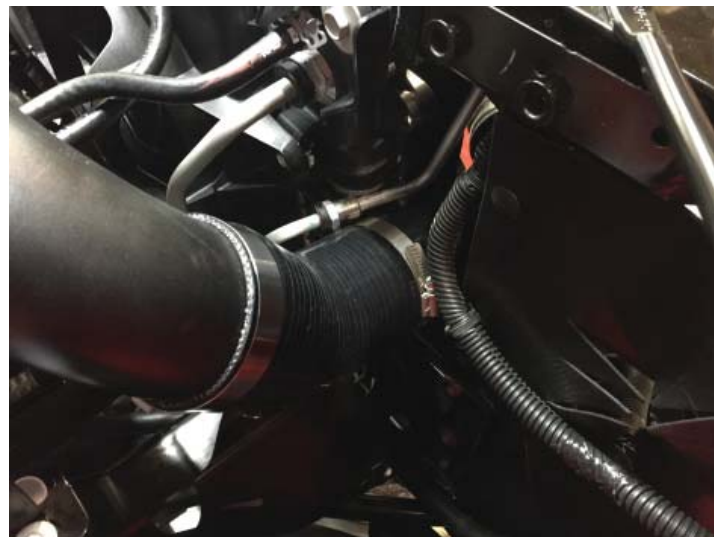
Tube #348 And Silicone 45° Reducer
