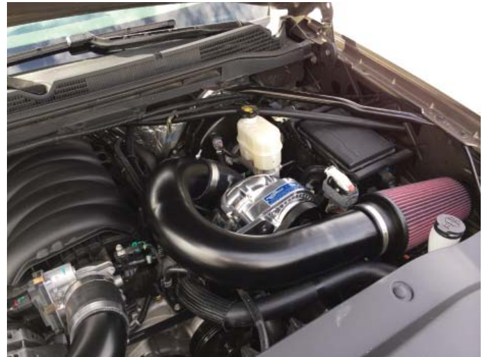
Front Facing Inlet Installed
