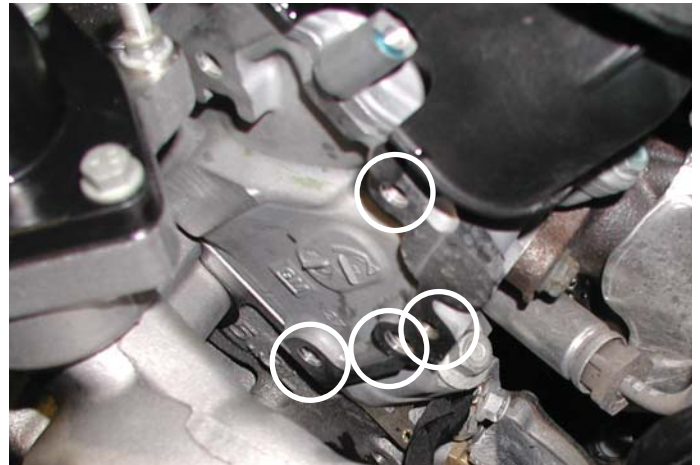
Sub Bracket Mounting Hole Locations
