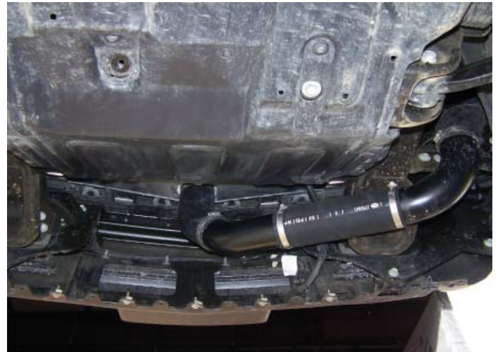
2014-15 Intercooler Discharge Installed
