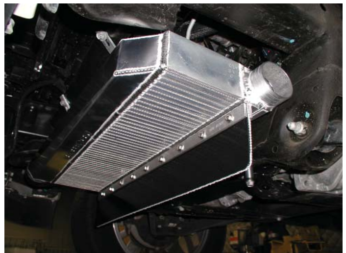
Intercooler Assembly Installed
