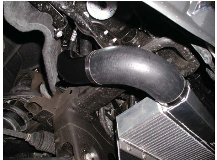
2015-14 Model: Intercooler Discharge Coupler and Tube Installed
