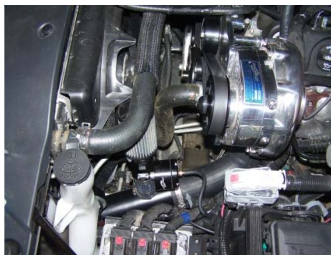
Surge System Installed (Vertical Intercooler)
