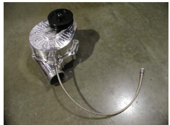
Oil Drain Line Installed
