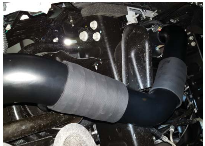
2016 Model Year: Tube #348 Installed
