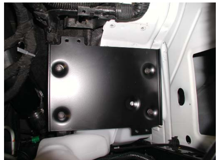
ECU Relocation Bracket Installed
