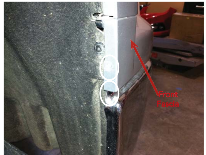
Remove Side Fascia Hdw. (Pass. Side Shown)
