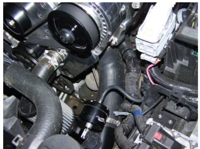
Coupler Connection At Supercharger
