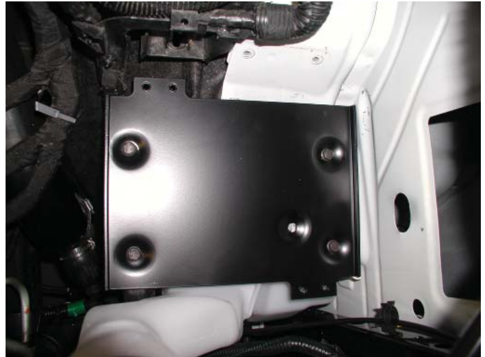
ECU Relocation Bracket Installed
