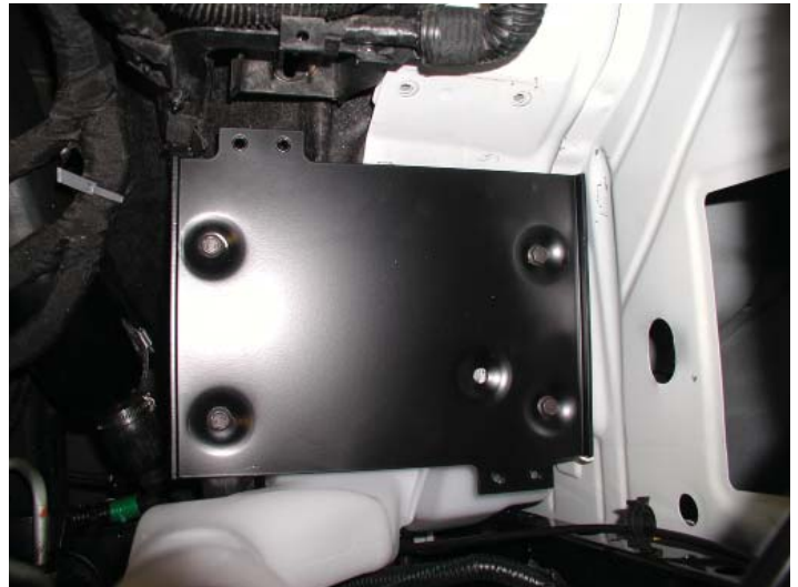
ECU Relocation Bracket Installed
