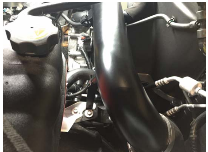
Throttle Body Tube Bracket Installed
