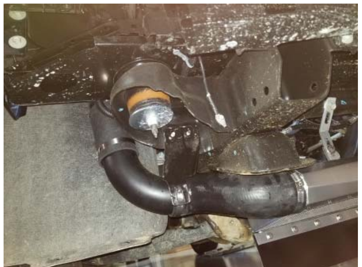
Tubing Out Of Intercooler Installed
