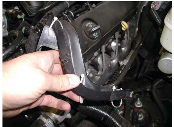
Main Wiring Harness Plastic Bracket Removed
