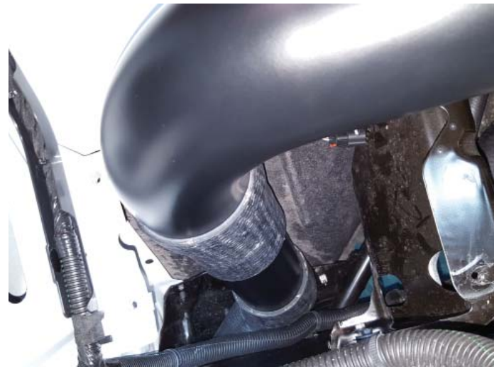
Tube #203 and Rubber Reducer Installed
