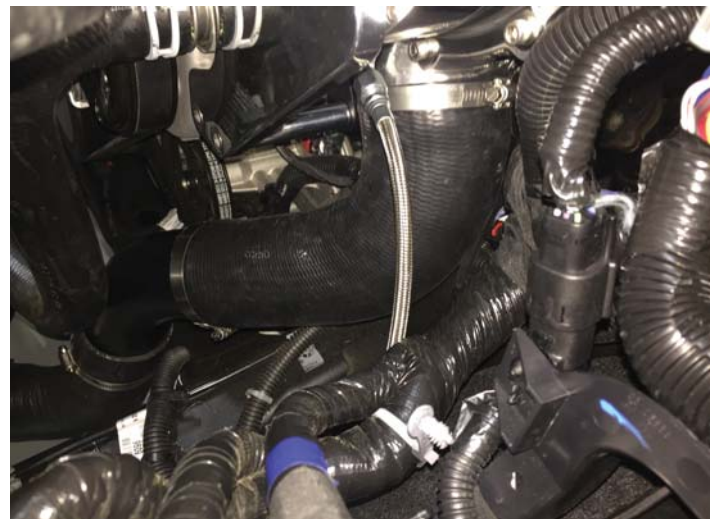
Tubing Out Of Supercharger
