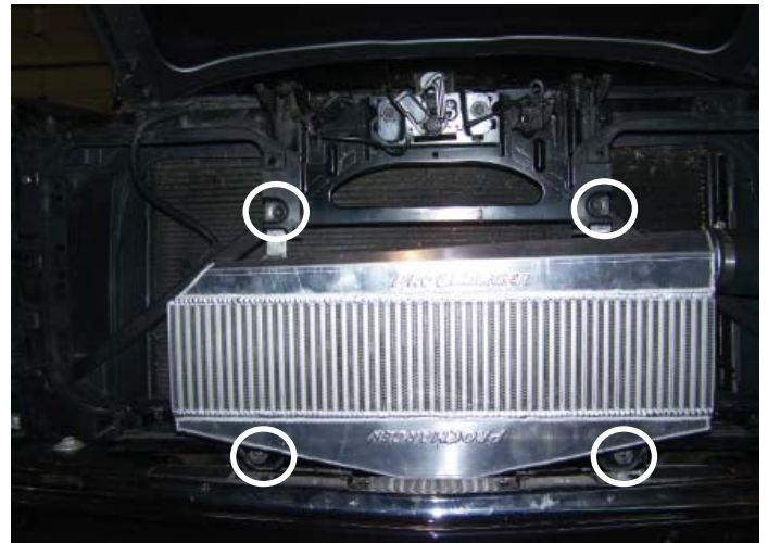
2014-15 Intercooler Assembly Installed
