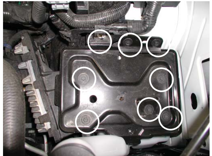
Auxiliary Battery Tray Bolt Locations
