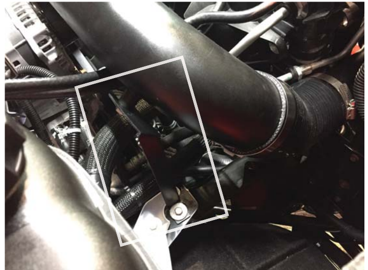
Throttlebody Tube Brace Installed
