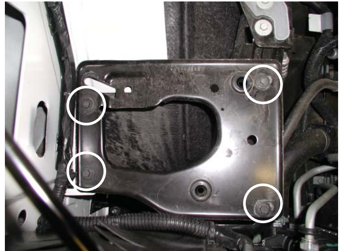
Factory Airbox Mounting Bracket Bolt Locations
