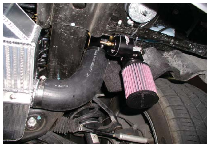
Surge System Installed (Horizontal Intercooler)
