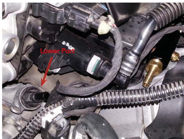
Vacuum Manifold Lower Port (5.3L)
