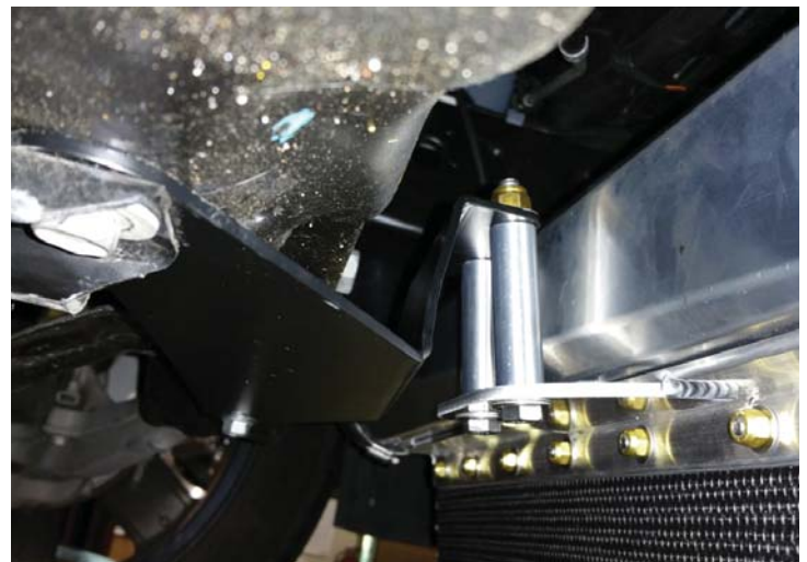
Rear Intercooler Bracket Installed On IC
