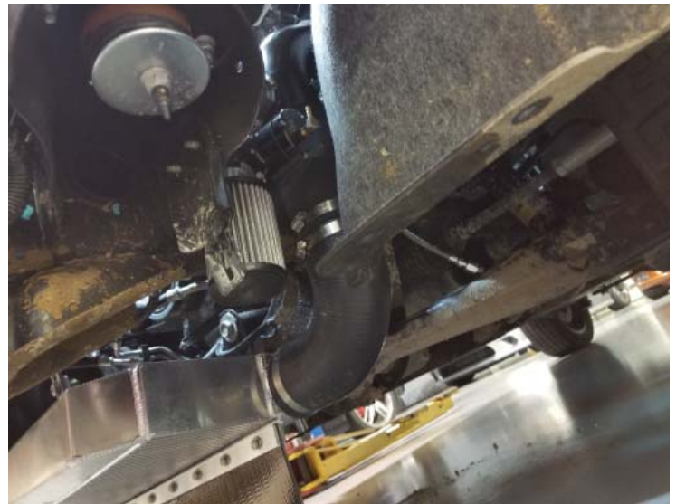
2017 SUV Tubing To Intercooler Installed
