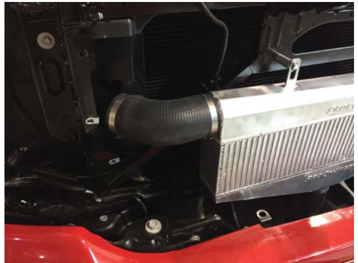
Tubing Out Of The Intercooler
