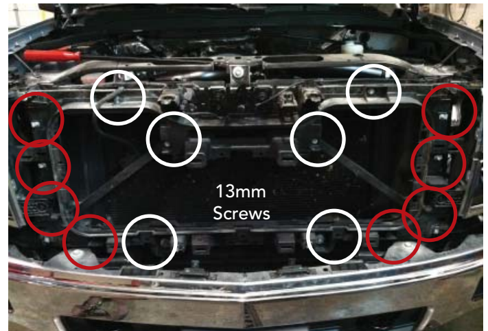
Remove Plastic Radiator Shroud
