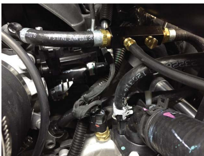
Vacuum Manifold Port (6.2L)
