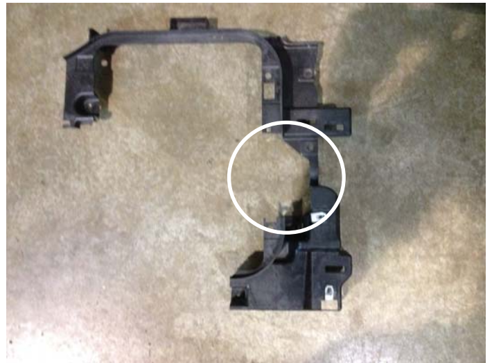
Drivers Side Radiator Shroud Trimmed
