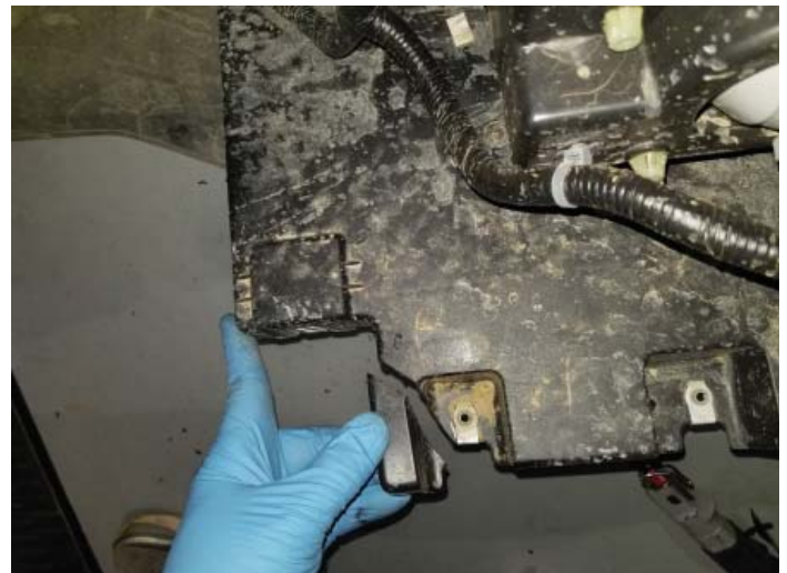
Fender Panel Trimmed (shown from above)
