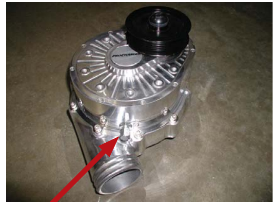
Remove Drain Cap
