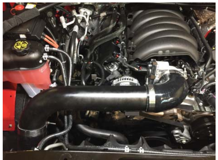
Tubing To Throttlebody Installed
