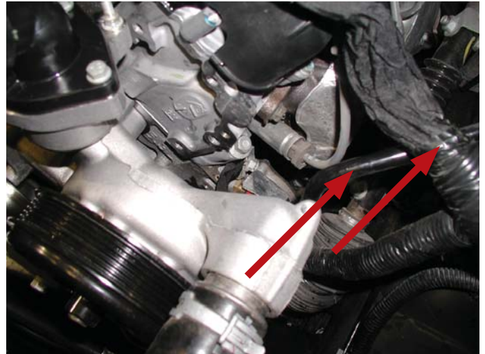
Harness and Brake Booster Line Relocation
