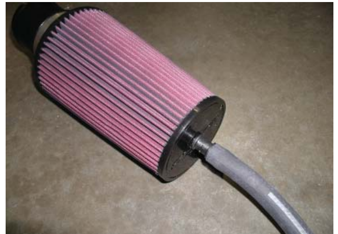
Air Filter With PCV Line Installed
