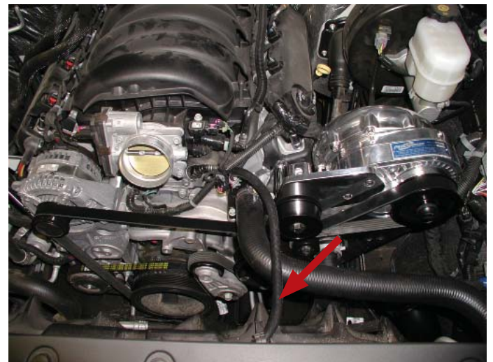
Slide Coolant Line Over For Additional Clearance
