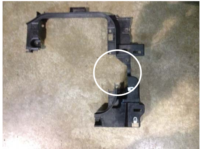
Drivers Side Radiator Shroud Trimmed
