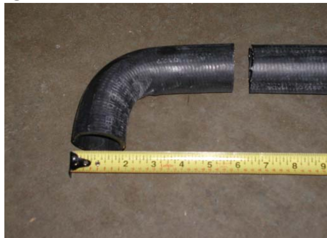
1.5" Rubber Elbow Trimming (Horizontal Intercooler)
