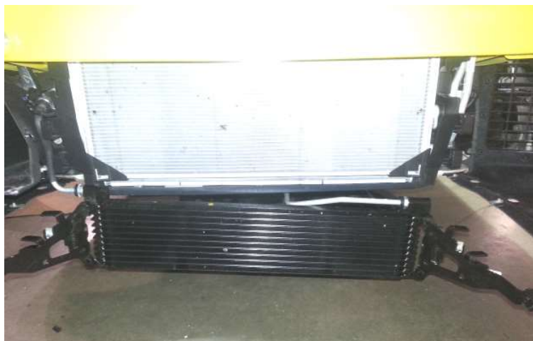
Transmission Cooler Dropped Down
