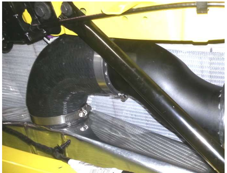
Tube #316 Installed (H.O. Intercooler Only)
