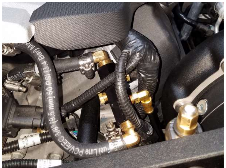
Vacuum Manifold Installed
