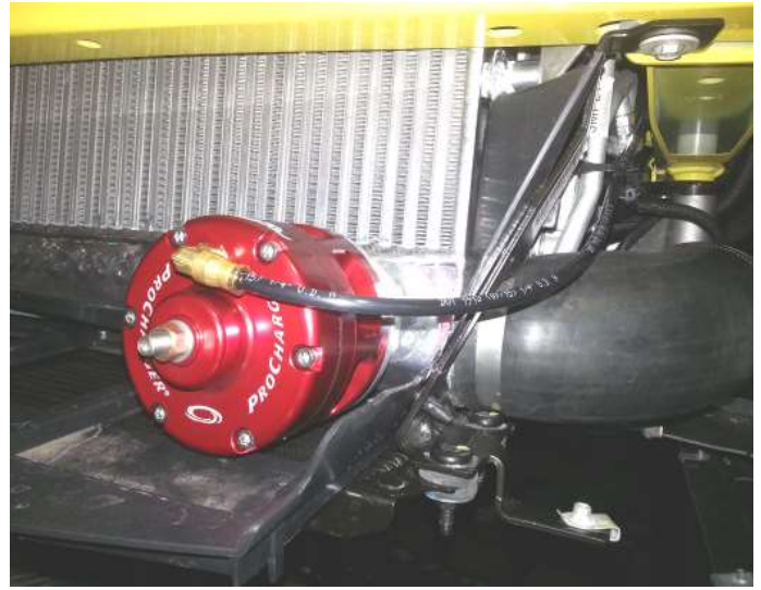
Race Valve Installed
