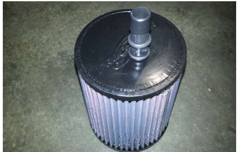
Plastic Fitting Installed in Air Filter
