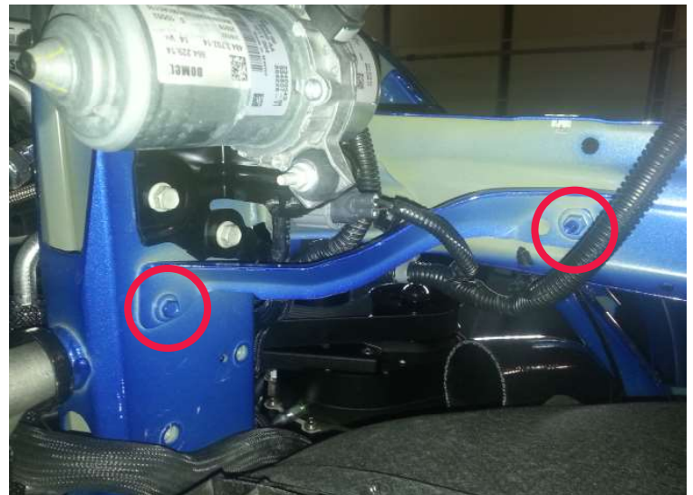
Fender Support Brace
