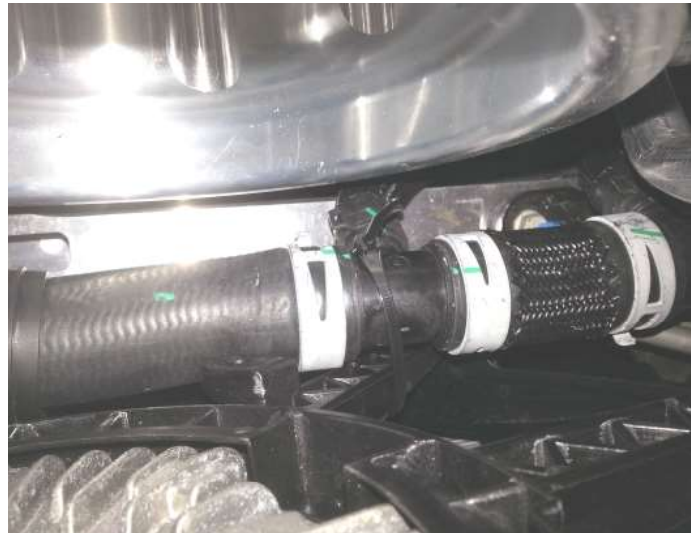
Zip Tie Radiator Hose to Fan
