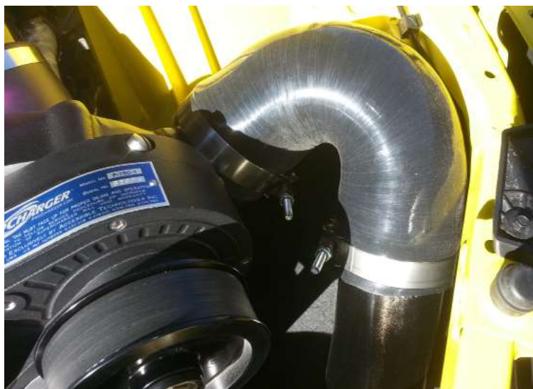
Blower Discharge Tube Installed
