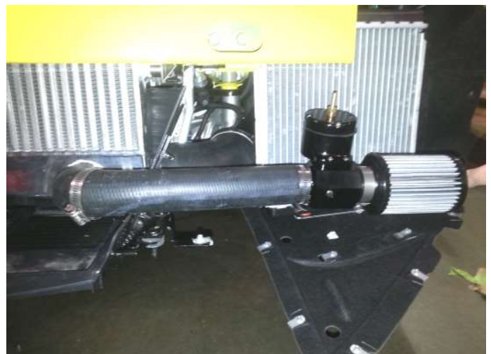
Proflow Surge Valve Installed
