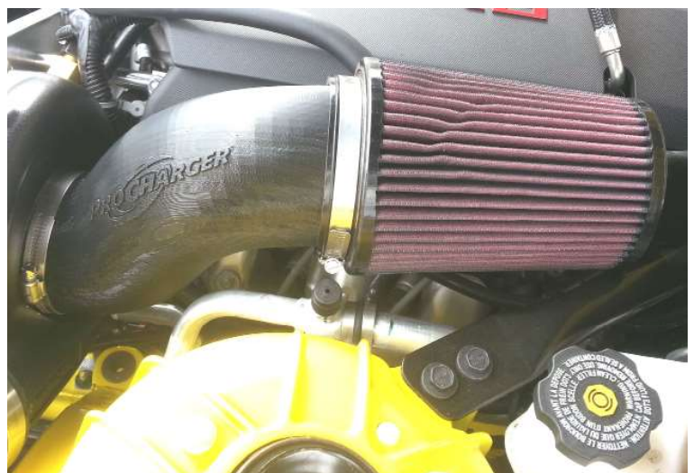
W/O Strut Tower Brace Air Inlet Installed
