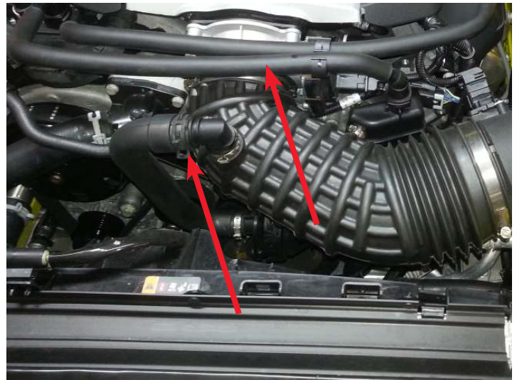
Disconnect Hoses from Inlet Tube
