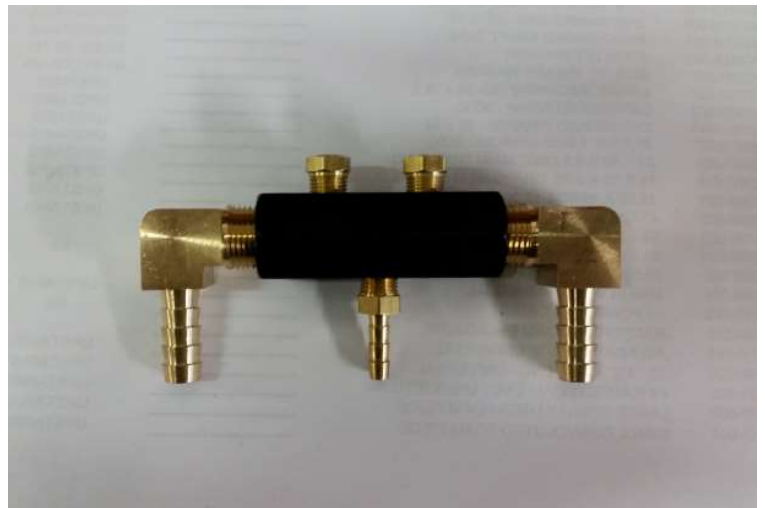
Vacuum Manifold Assembled
