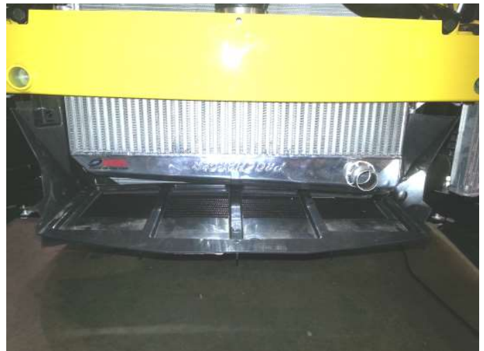
Modified Air Shroud Installed
