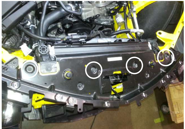
Remove Radiator Cover Bolts
