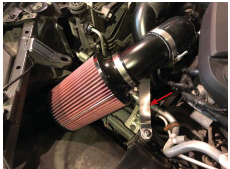
Air Inlet Brace Installed
