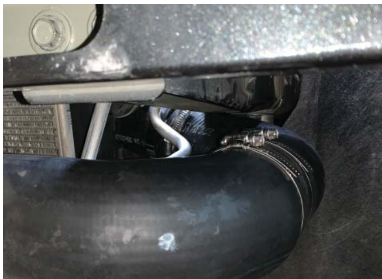
Lower Intercooler Connection
