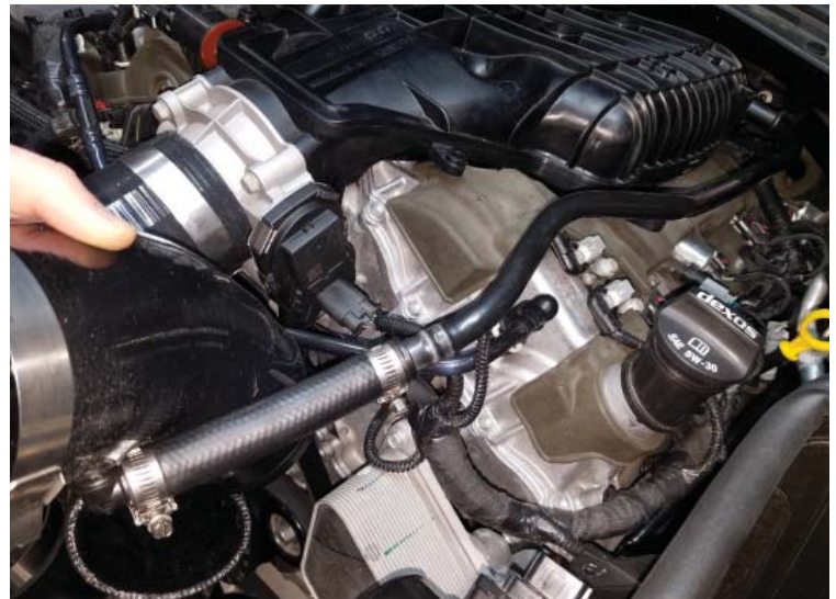
Rotomold Inlet Installed
