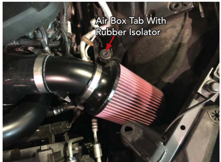
Air Filter Installed
