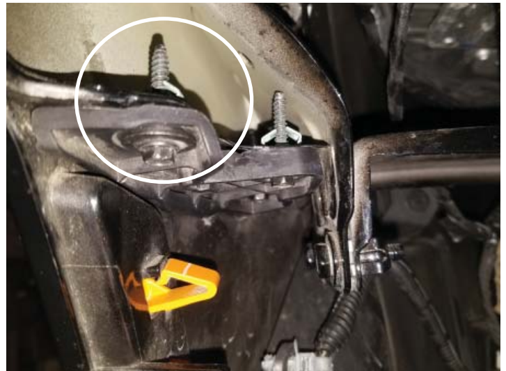
Screws Behind Wheel Liner
