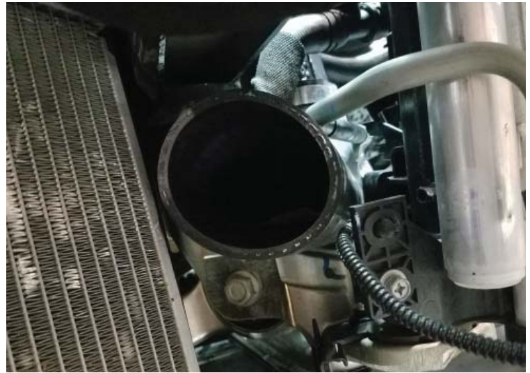
Blower Discharge Tube Installed
