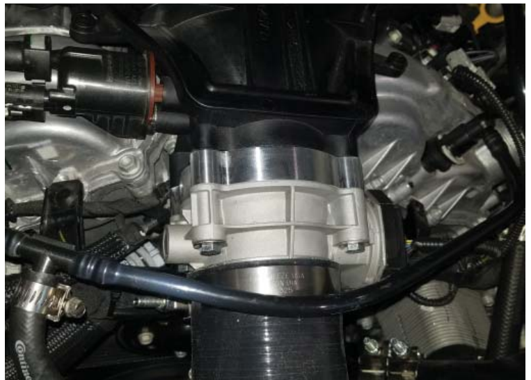
Throttle Body Spacer
