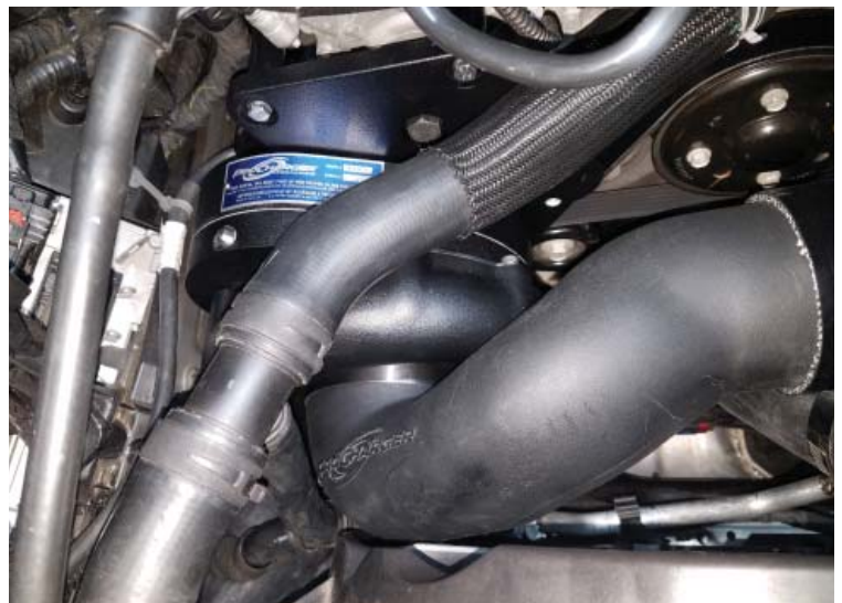
Rotomold Inlet Installed
