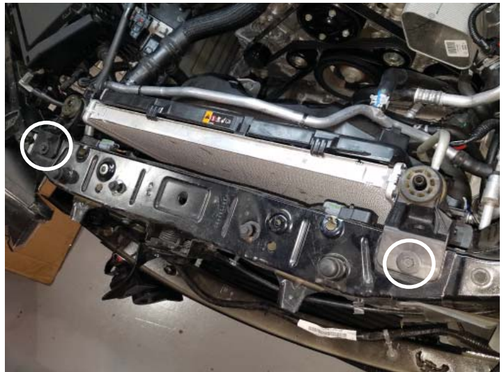
Upper Radiator Brackets Installed
