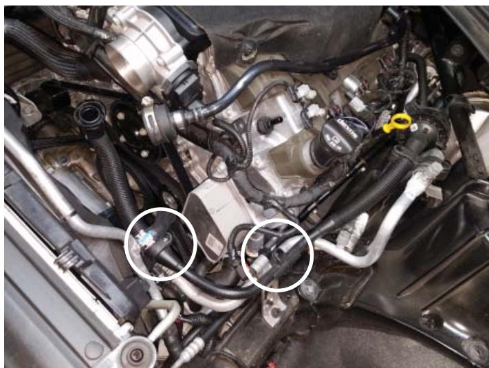
Sound Tube Connection
