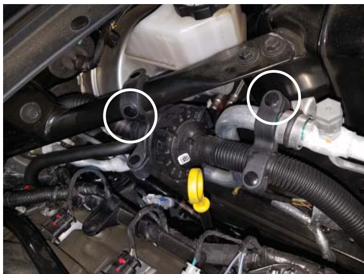
Sound Tube Connection
