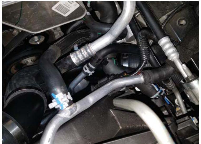
Lower Intercooler Connection
