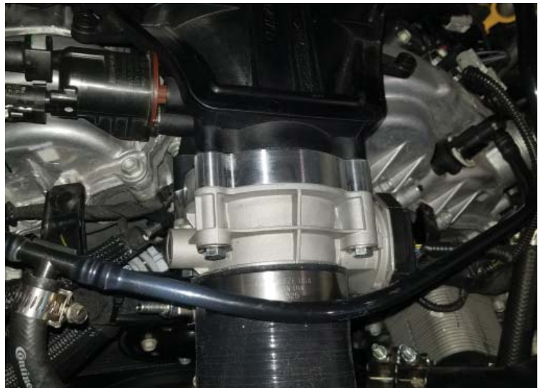
Throttle Body Spacer
