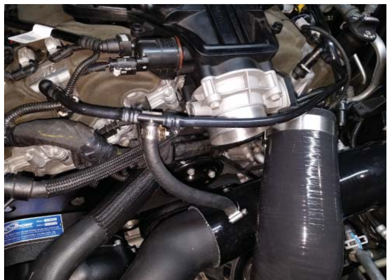
PCV Line Connected
