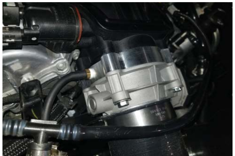
Vacuum Hose Installed
