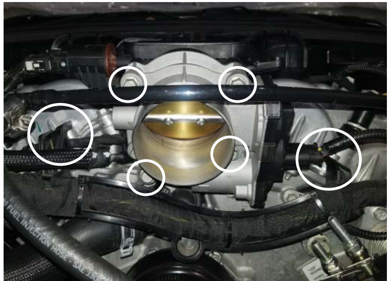
Throttle Body Removal
