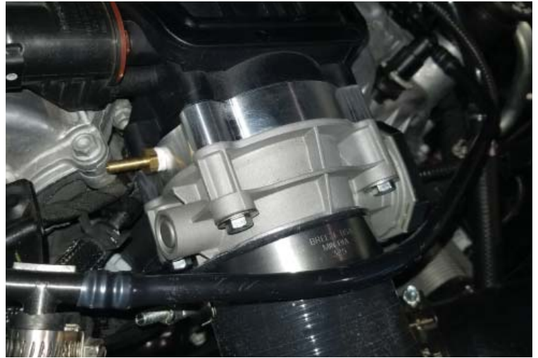
Vacuum Fitting Installed
