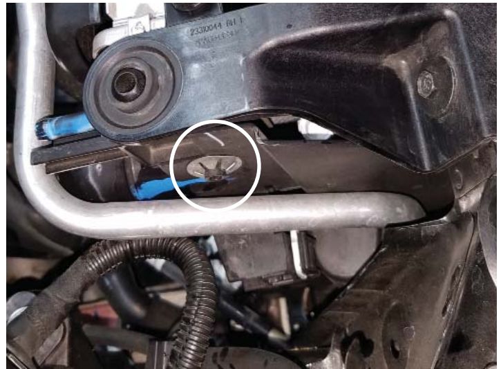
Pry Off Metal Retainers
