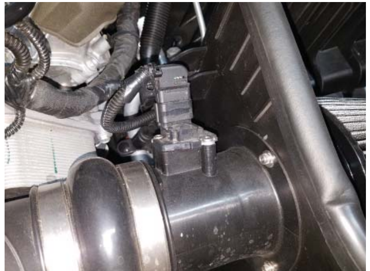
Disconnect MAF Sensor
