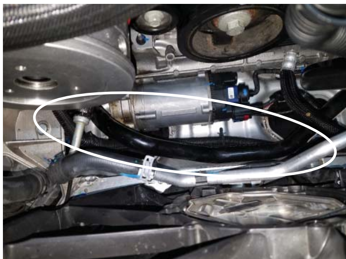
Relocated Wiring Harness
