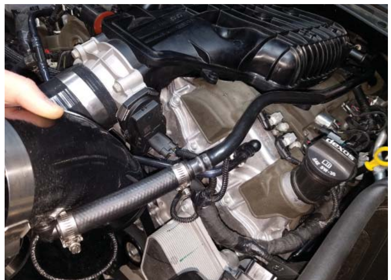
Drivers Side PCV Line Connected
