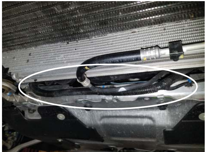
Release Wiring Harness
