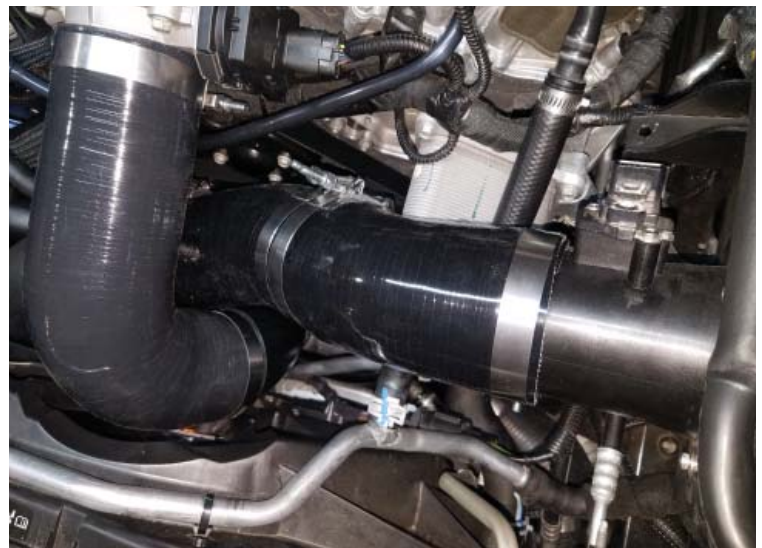
Air Inlet Assembled
