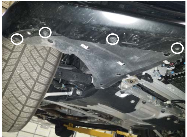
Remove Bottom Fascia Screws
