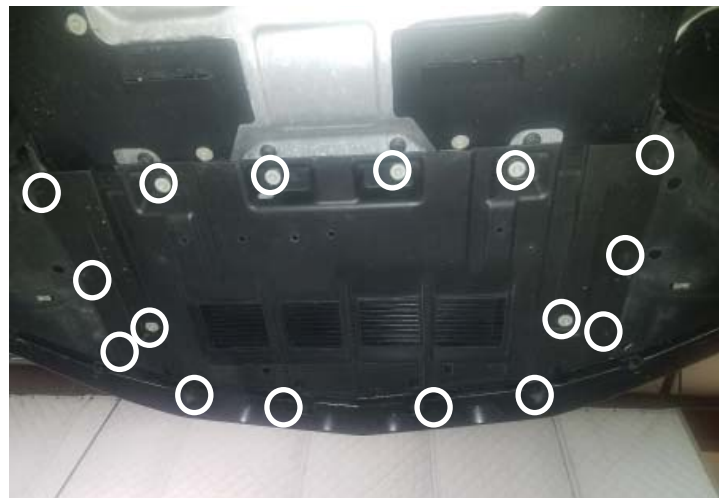
Plastic Splash Panel Screws and Bolts
