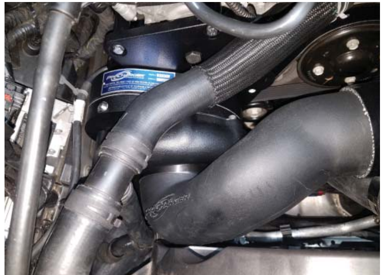
Rotomold Inlet Installed
