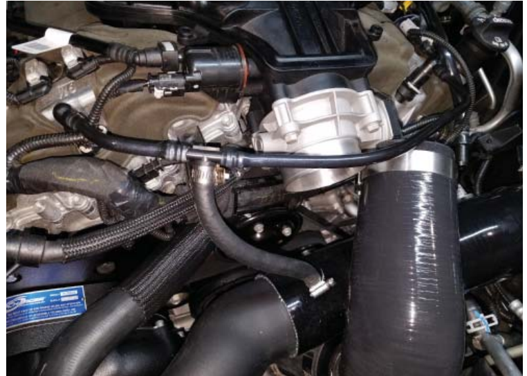
PCV Line Connected
