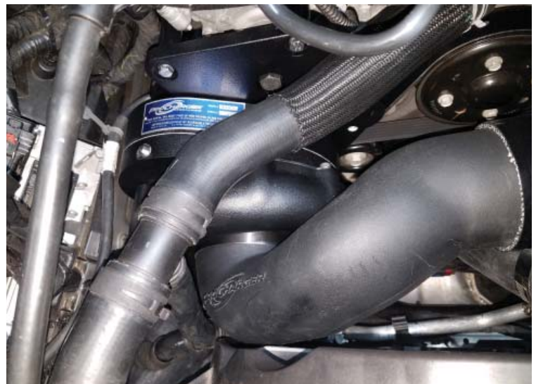
Rotomold Inlet Installed
