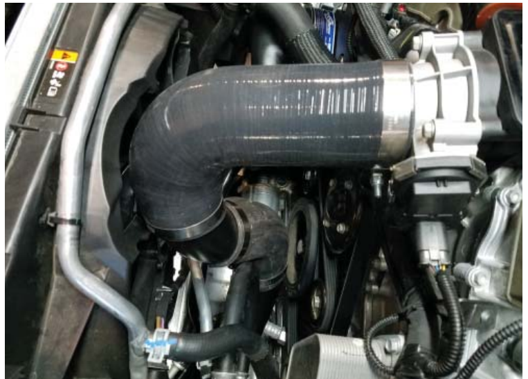
Throttle Body Connection
