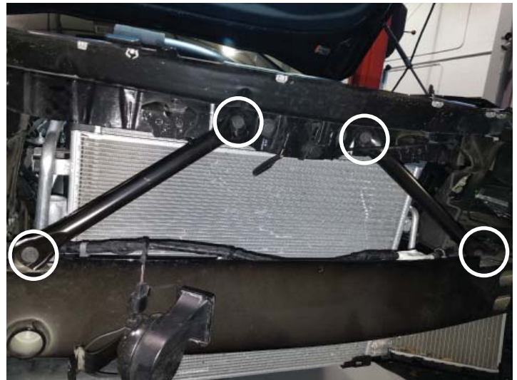
Core Support Braces
