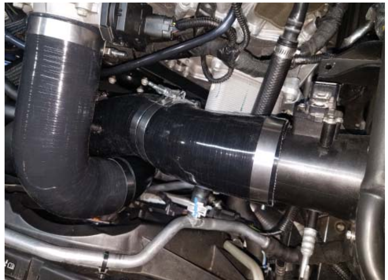
Air Inlet Assembled
