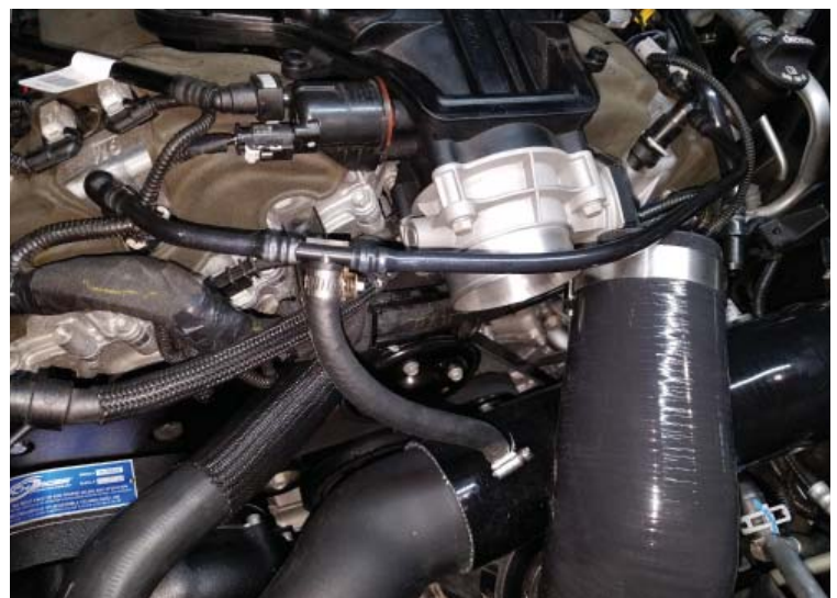
PCV Line Connected
