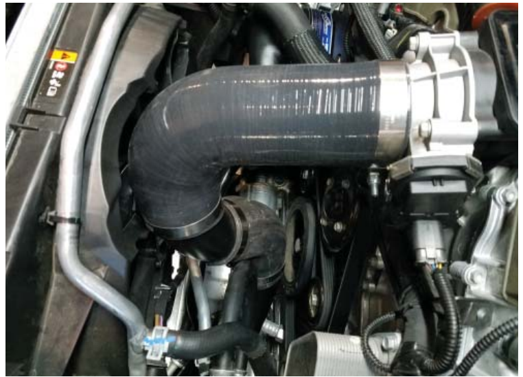
Throttle Body Connection
