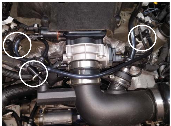
PCV Line Removal
