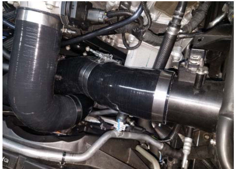
Air Inlet Assembled
