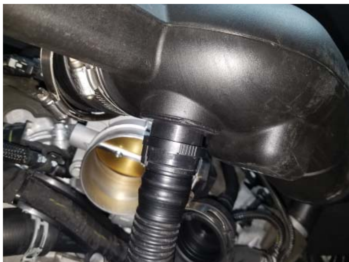
Sound Tube Connection
