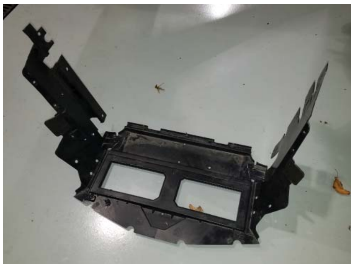
Radiator Shroud Removed
