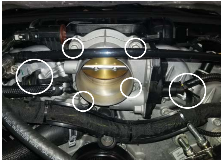
Throttle Body Removal
