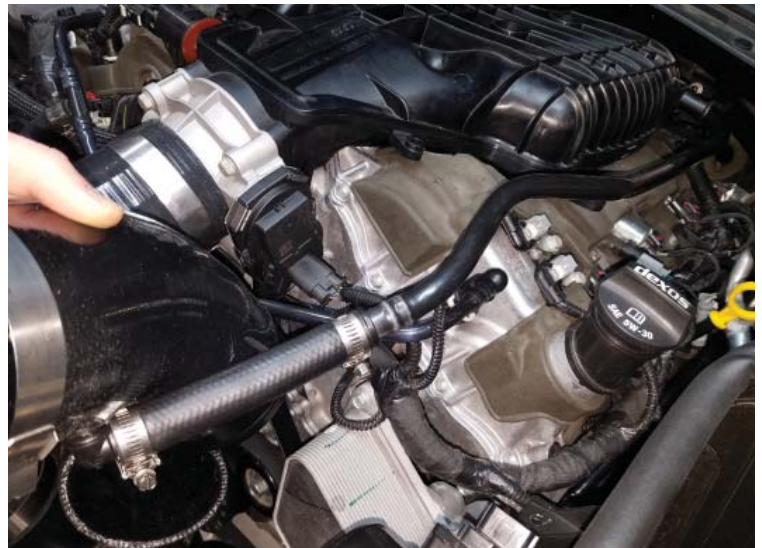
PCV Line Connected
