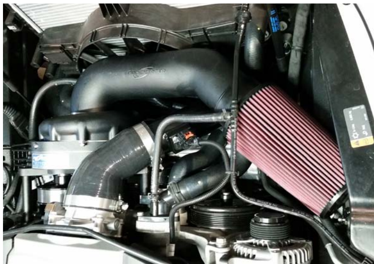
Stage 2 Air Inlet Installed
