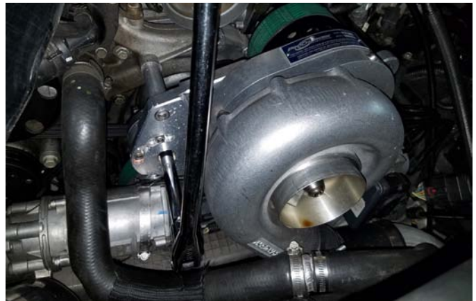
Rotate Tensioner Counter Clockwise
