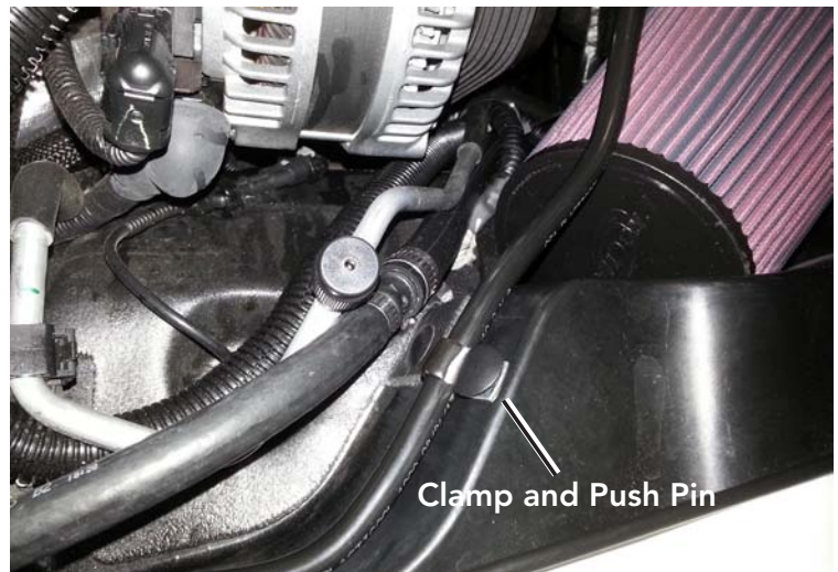
Coolant Hose Loop Clamp Installed
