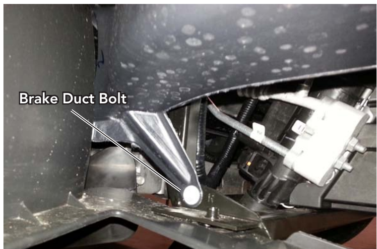
Brake Cooling Duct Bolt (x2)
