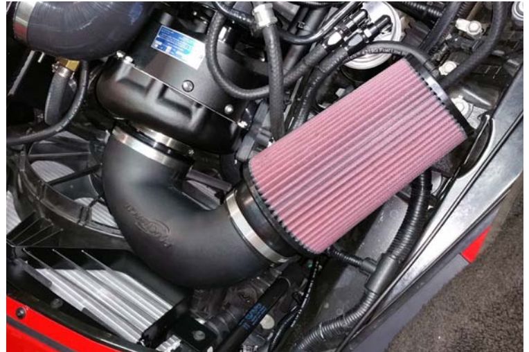
Rotomold Air Inlet Installed
