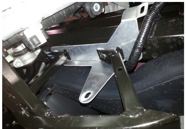
Intercooler Bracket Installed (Driver's Side)
