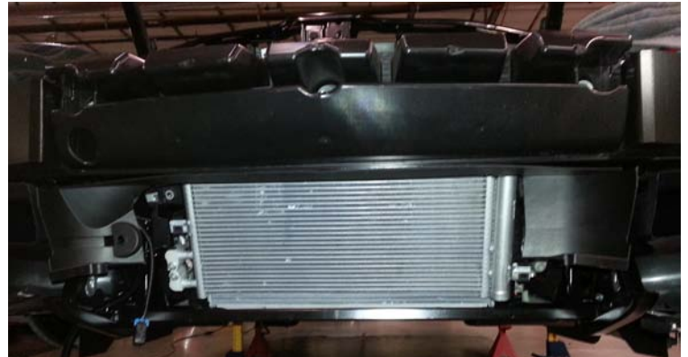
Modified Plastic Shroud Installed
