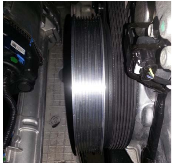
Crank Pulley Installed
