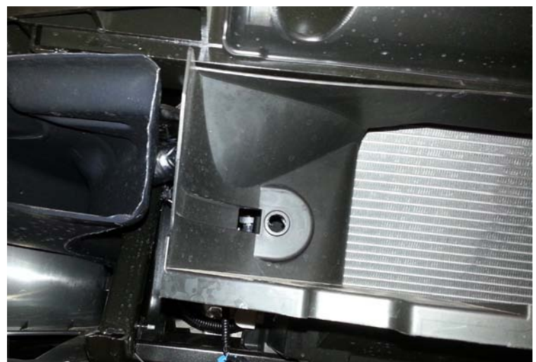
Ambient Air Temperature Sensor Removed
