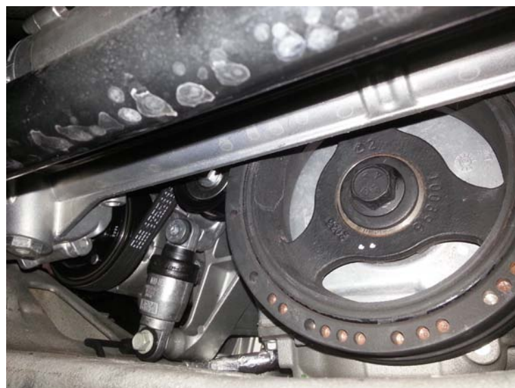
Crankshaft Balancer Bolt
