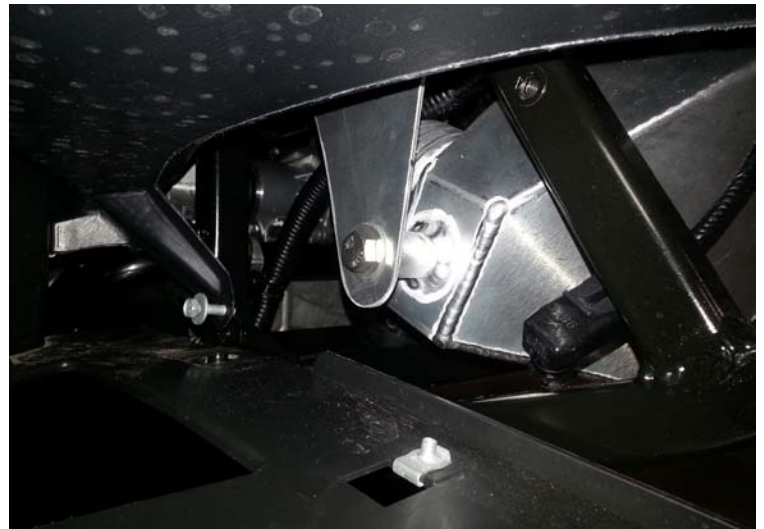
Lower Intercooler Bolts Installed
