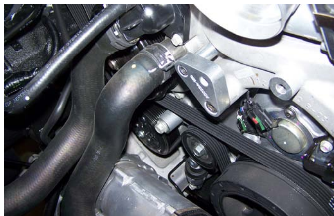
Sub Bracket Installed
