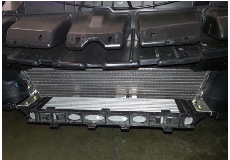
Trans Cooler Mounted (If Equipped)
