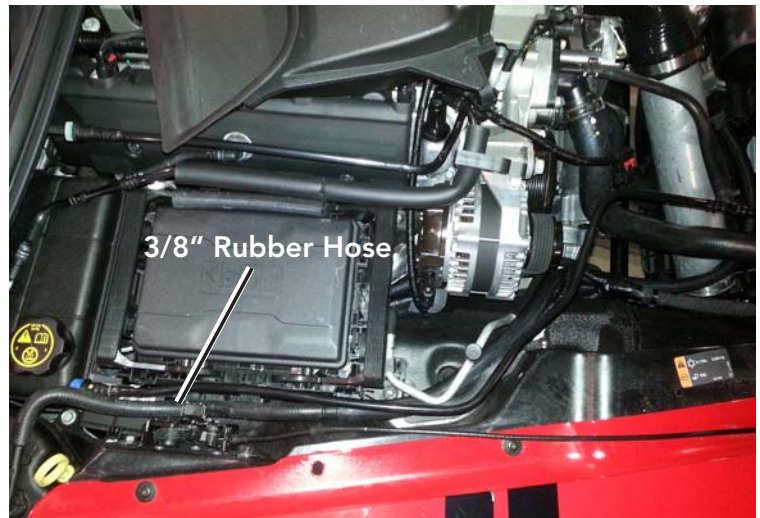
Passenger's Side PCV Routing
