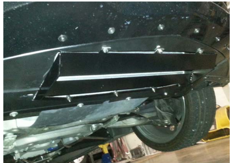
Modified Skid Panel Installed (Horizontal I/C)
