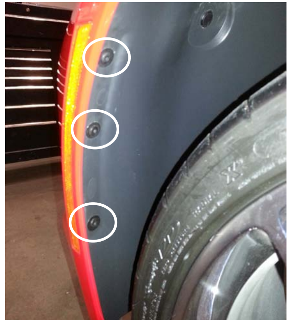
Wheel Liner Screws (3 Per Side)
