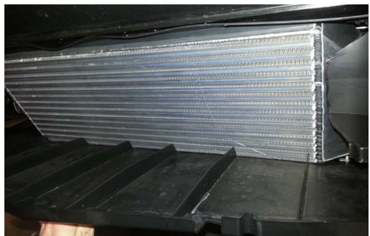
Modified Skid Panel Installed (Vertical I/C)
