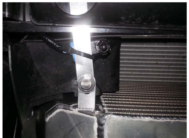
Ambient Air Temperature Sensor Installed
