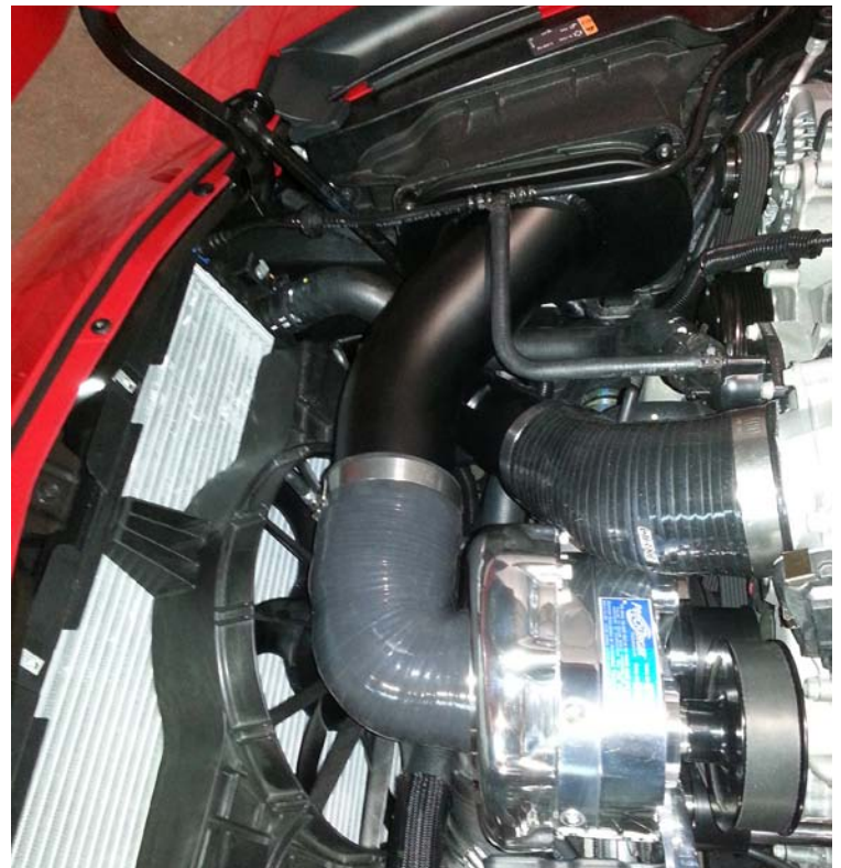
Inlet Tube Installed
