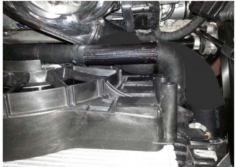
Cooling Fan Installed
