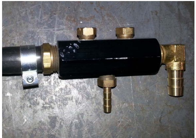
Vacuum Manifold Assembled
