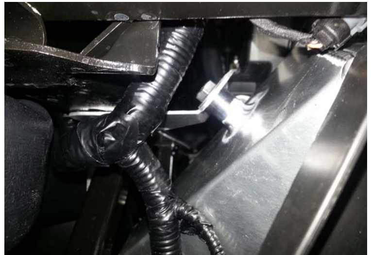
Upper Intercooler Bolts Installed
