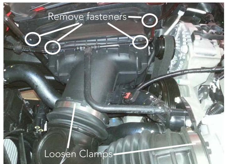
Loosen Clamps and Remove Fasteners
