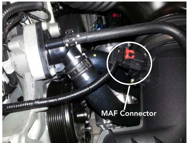
Disconnect MAF Harness From Intake Tube
