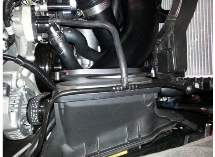
Connecting the Inlet Tube to Factory Air Box
