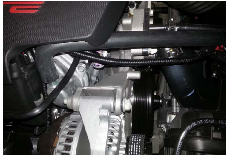
Passenger's Side PCV Routing
