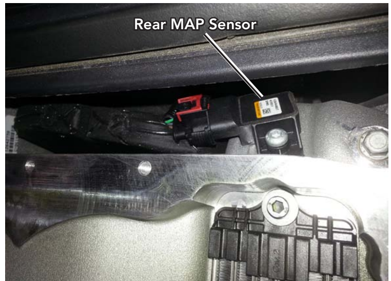
Disconnect Rear MAP Sensor
