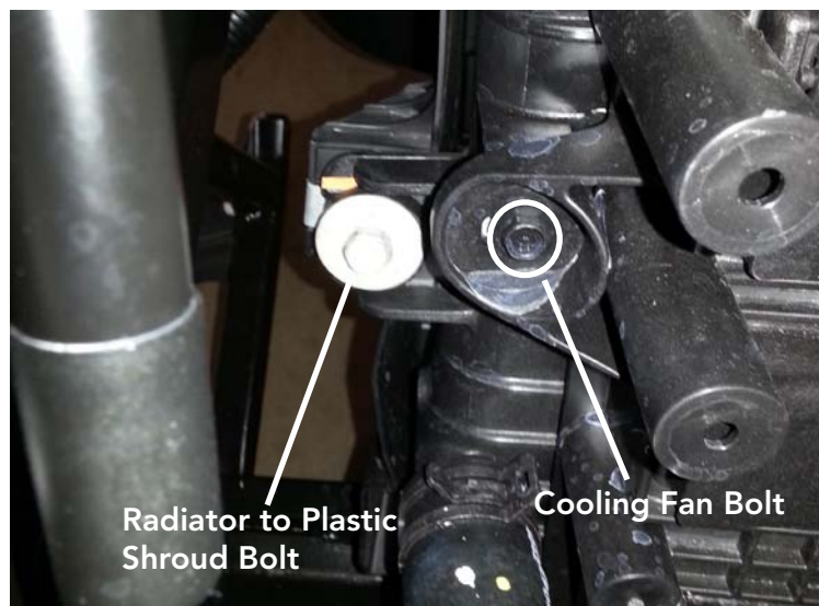
Radiator and Fan Bolts (x2)
