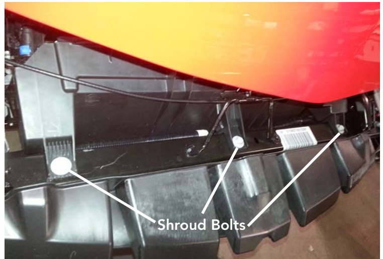
Shroud to Bumper Support Bolts
