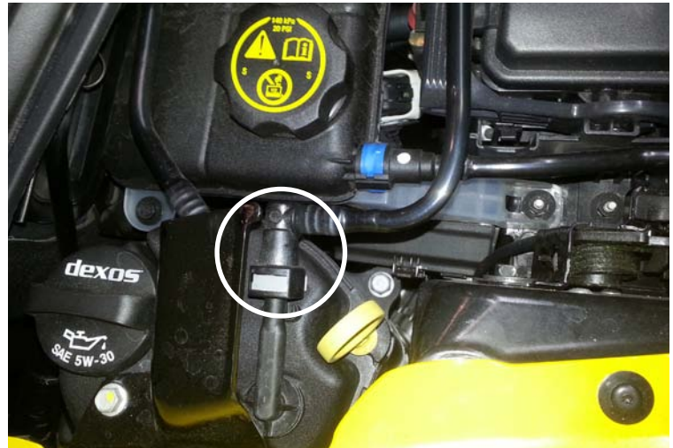
Disconnect Factory PCV Line
