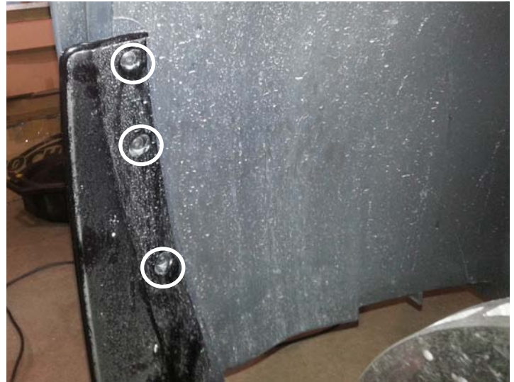
Wheel Liner Screws
