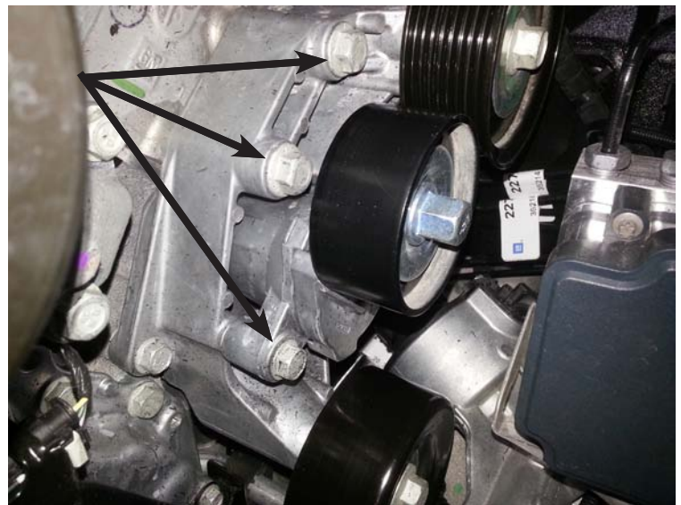
Tensioner and Idler Bracket
