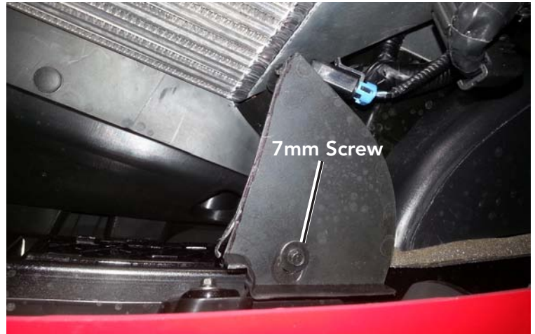
Plastic Shroud to Fascia Screw (x2)
