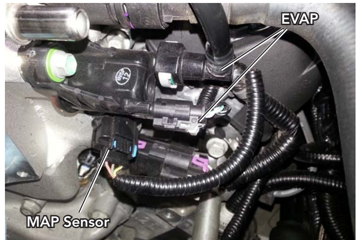
Disconnect MAP and EVAP (Driver's Side)
