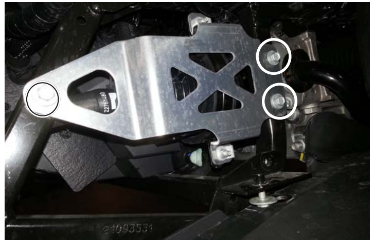
Pump Bracket Bolts
