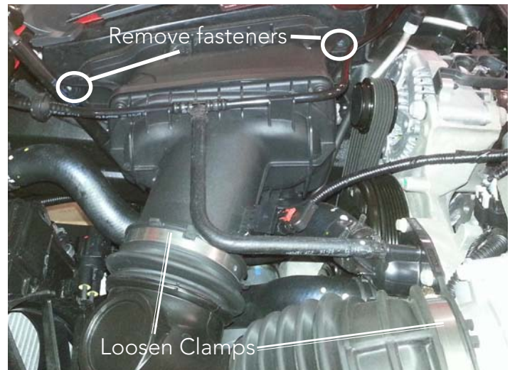
Loosen Clamps and Remove Fasteners
