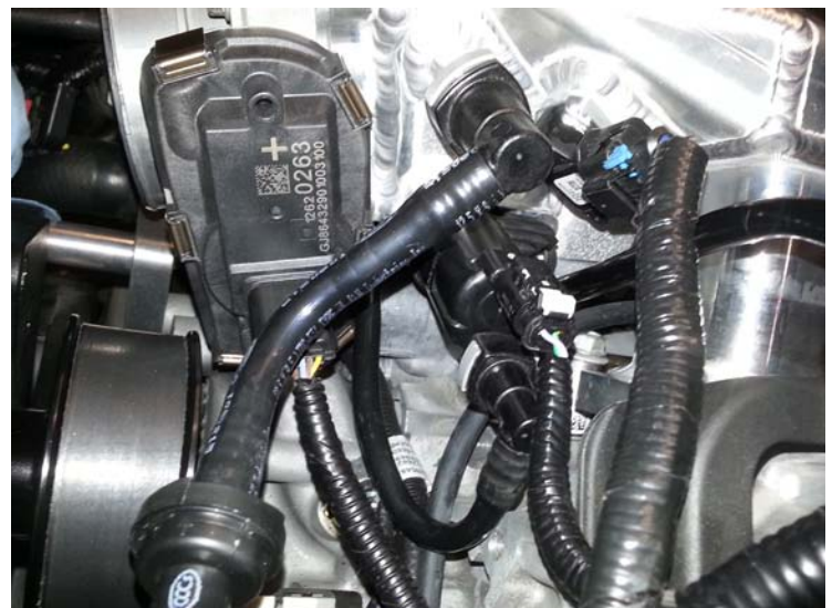
MAP, EVAP and PCV Lines Connected
