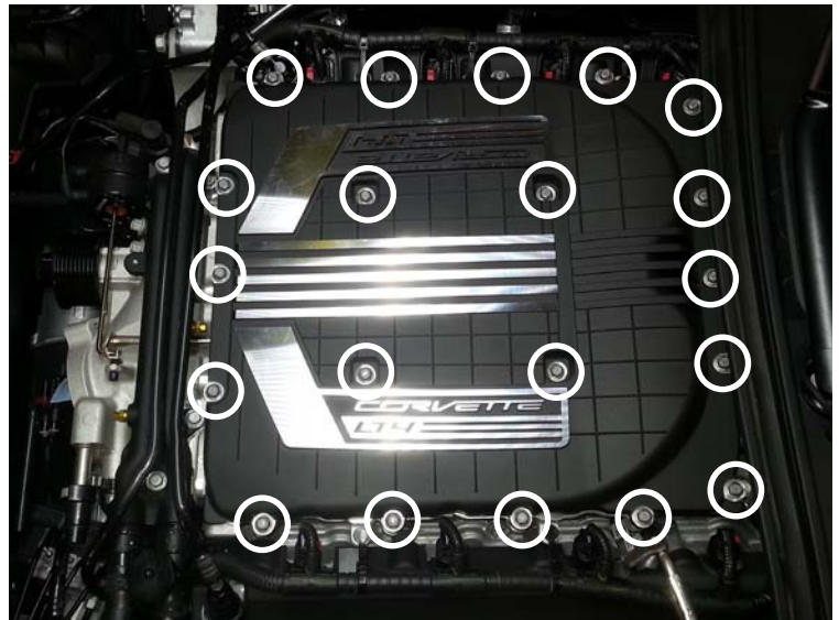
Supercharger Lid Bolts
