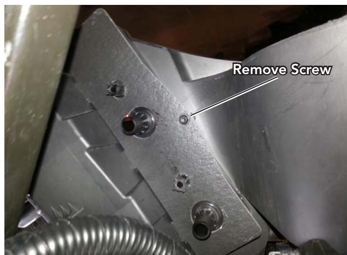
Heat Exchanger Cover
