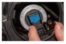
1. Referencing your vehicle's user manual or online resources, locate and remove your factory bulb. In most cases, the bulb must be disconnected from the factory electrical connector, and turned counterclockwise to remove.
