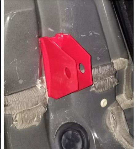
11. With the help of a friend to hold the reinforcement plate, install the two 3/8" bolts with a washer in each drilled hole on each side of the car. Ensure that you tighten each bolt in steps so that you do not bind the screws going thru the holes (This will cause you to strip the bolts). Torque the 3/8" bolts to **35 ft lbs**
