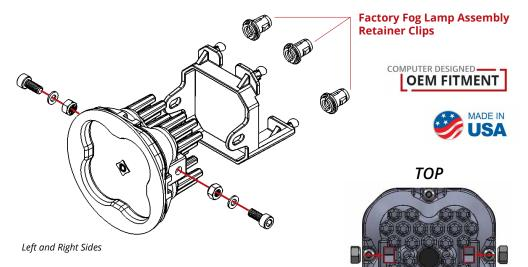
1. Attach the bracket to the pod, using one screw on each side. These screws will also determine the aim of your SS3 pods. Adjust the angle of the light in the bracket, then tighten down these screws. See diagrams above and to the right. Make sure the bracket is in the correct orientation.
